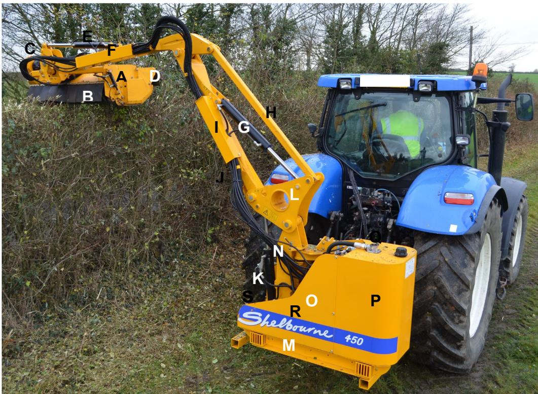
A fully independent PTO operating at 540 rpm, with a 1 & 3/8" SAE 6 spline shaft and rotating in a clockwise direction is required.
