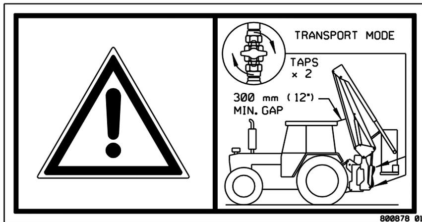
10. For 400 models the slew cylinder should be mechanically locked by the slew locking device being put in place during all transportation on the public highways.
