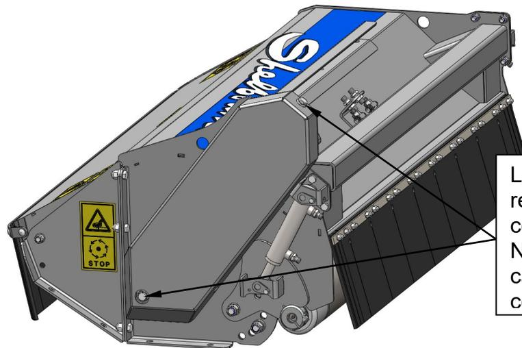
Loosen fixings to remove drive cover
