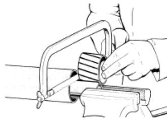
Shorten the inner and outer Sliding profiles by the same length as the guard tubes.
