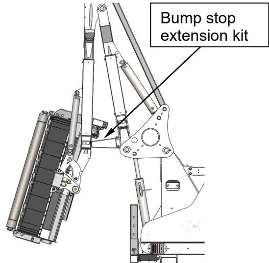
4. For 400 models use the slew cylinder to rotate the arms fully back, and then position the cutting head with the flail facing the operator and the top of the cutting head towards the traffic.
