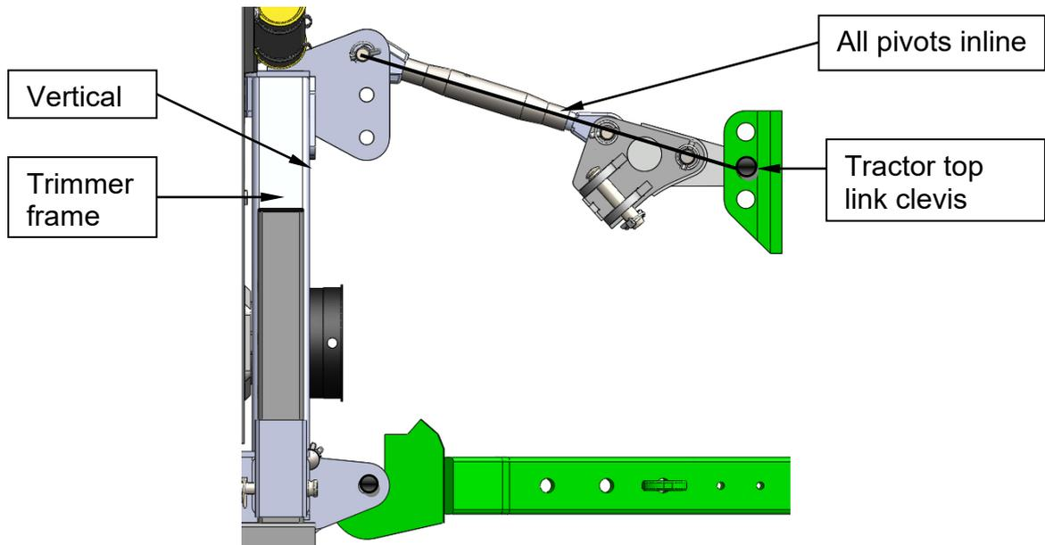
11. Lengthen or shorten the top link so that on level ground the trimmer frame is vertical. This will also affect the angle of the cutting head in relation to the ground.
