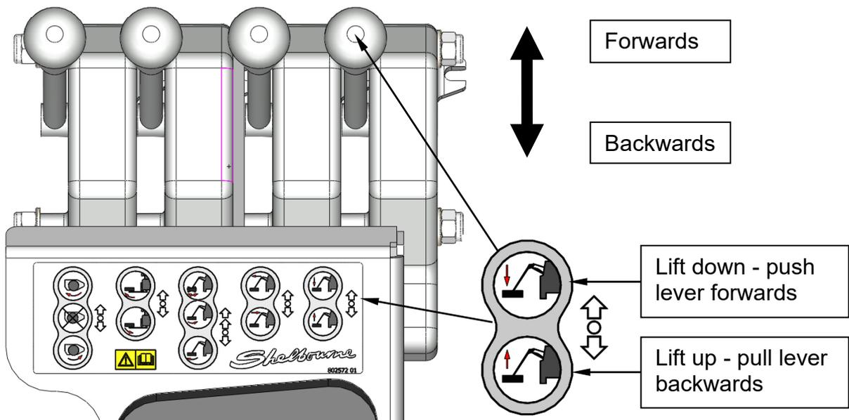
**Reach:** By moving the lever forward and backwards from the operator gives reach out and in respectively for the operation of the reach service.
