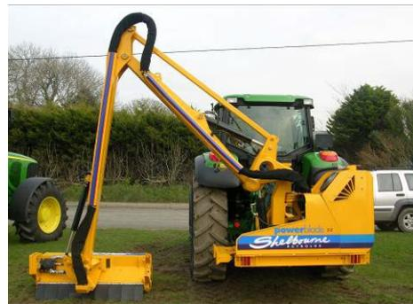
16. Correct adjustment has been reached when with the booms in the work position the machine remains parallel to the rear axle of the tractor. Take tyre squash into account when viewing this.
