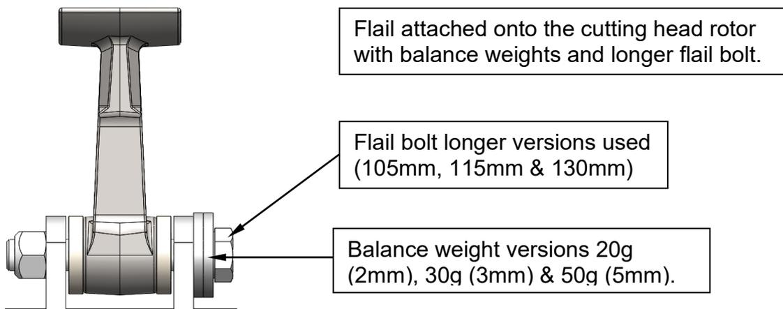
Replace spacers, bolts and nuts exactly when replacing flails. The flails themselves should wear evenly and be replaced as a set. Should one flail be lost then the flail at 180°, one place along should be renewed at the same time to preserve the balance.
