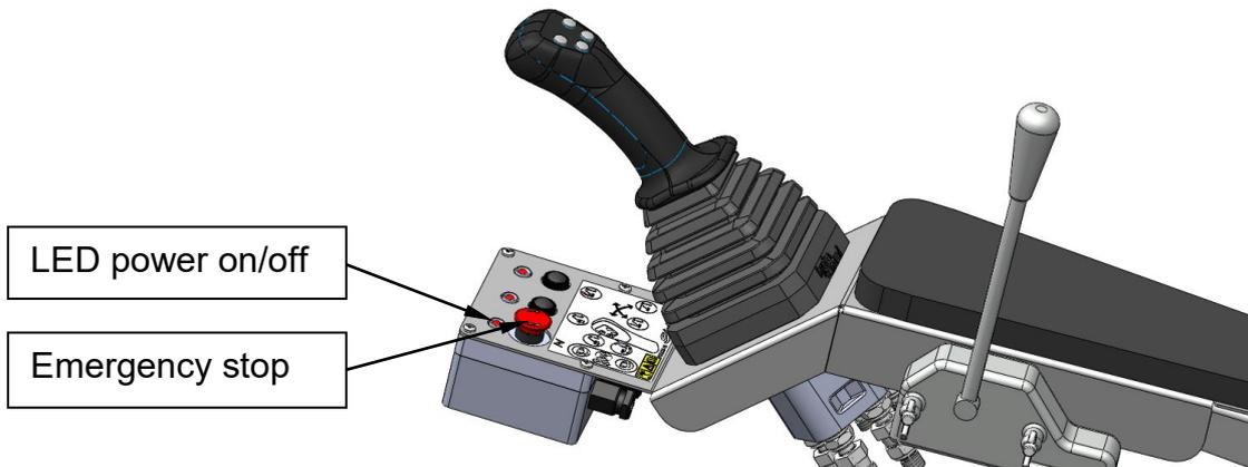
**Lift & Reach:** By moving the joystick to the left and right the reach cylinder is actuated in the relevant direction; moving it back/towards and forwards/away from the operator gives lift and lower respectively. These actions are proportional; that is small joystick displacements give slow cylinder movements and large displacements faster movements.
