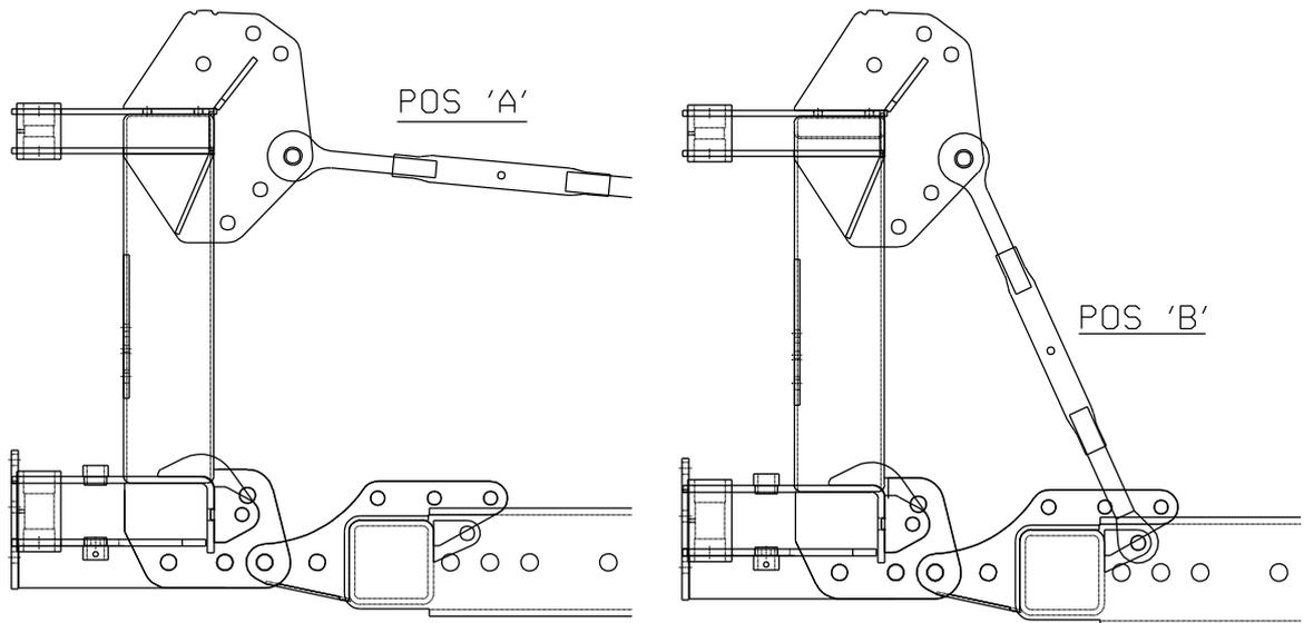
5. Detach the tractor drop arms from the drop links (item 12) by removing the drop link pin.
