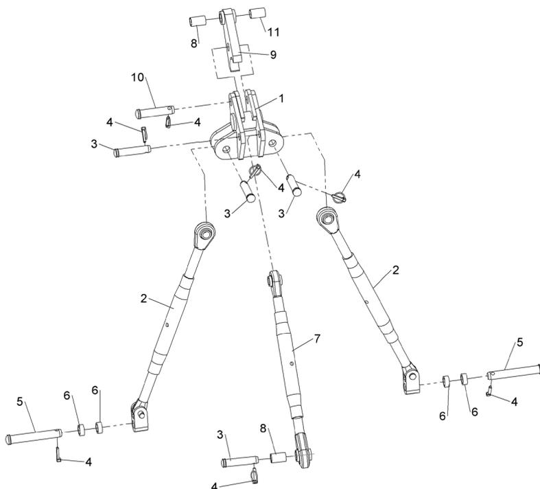
1. Identify if the tractor has lift arms with fixed ball ends or has a quick release ball end style. For Lift arms with the fixed ball ends remove lynch pin (item 4) before withdrawing the pin (item 5) allowing space for the fixed ball end.
