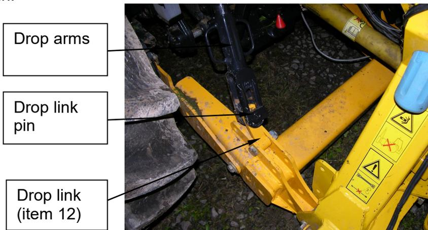
6. Release the axle bracket latches, allowing the sub frame to be lowered clear of the tractor by extending the adjustable top link.
