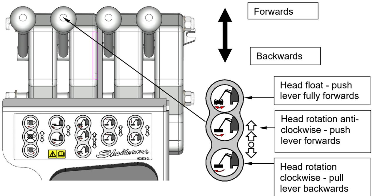
**Rotor up cut:** Engage the cutting head rotor in the up cut direction by moving the lever backwards.
