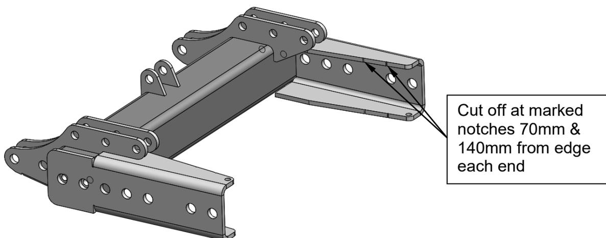
4. With the correct width and overall length identified assemble items 2 together with item 1 using items 3, 4, 5 and 6.
