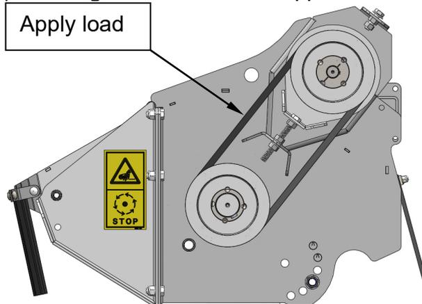
To adjust, slacken the nuts at the motor fixing bolts and the adjuster locknut, then turn the adjuster bolt in the required direction. Then tighten lock nut and fixing bolts and replace the drive cover.
