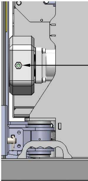
Sight glass for checking gearbox oil level
