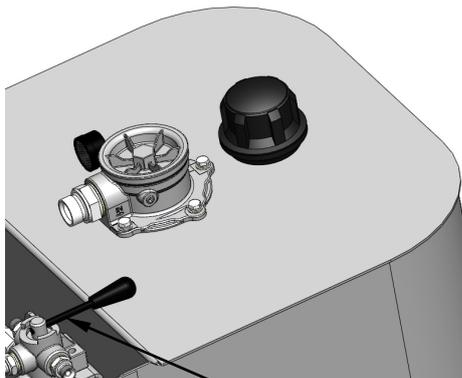
Manual lift float valve position on trimmer main frame
