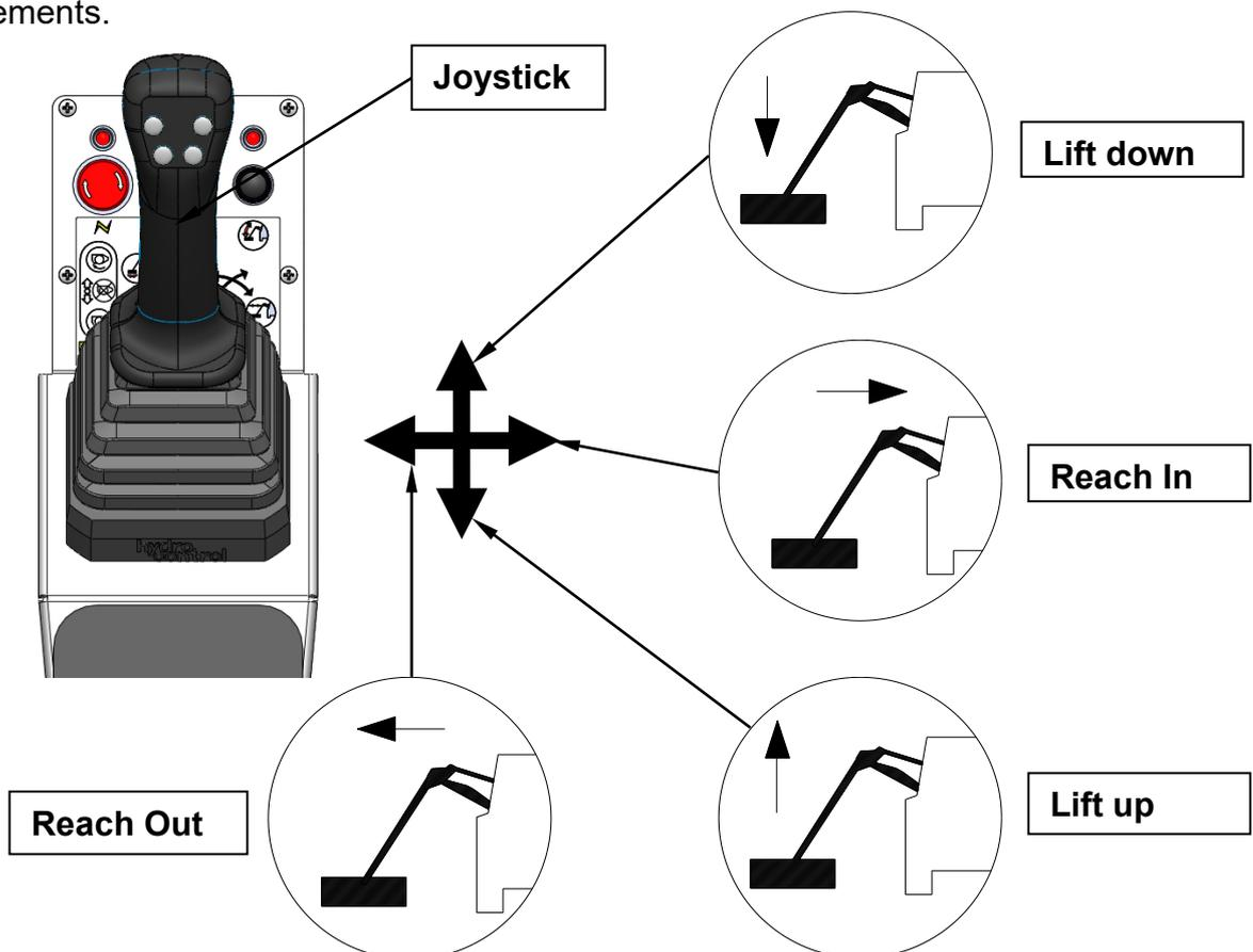
The top two buttons on the joystick operate the head rotation service either on or off.
