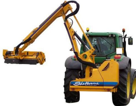
2. For 300 models fully close the head rotation cylinder so the flails are facing away from the operator. Then using the lift and reach cylinder bring the booms as close as physically possible to the tractor resting outer boom against the inner boom bump stop (this may not be possible for all tractors).
