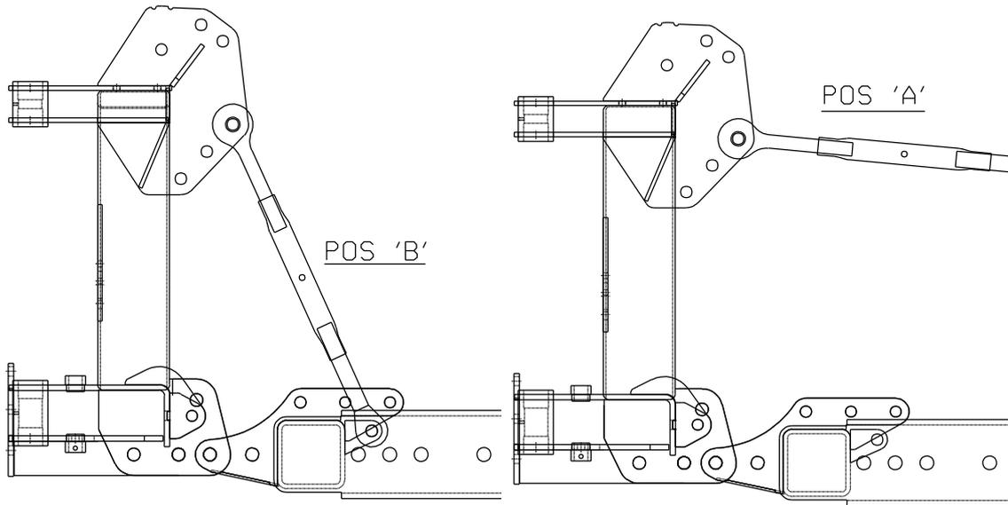
7. The machine should then be slowly and carefully raised to a height that brings the tractor's PTO shaft and the gearbox input shaft to the same approximate height, whilst checking at all times that if the lift arms are still attached they are fouling nothing.
