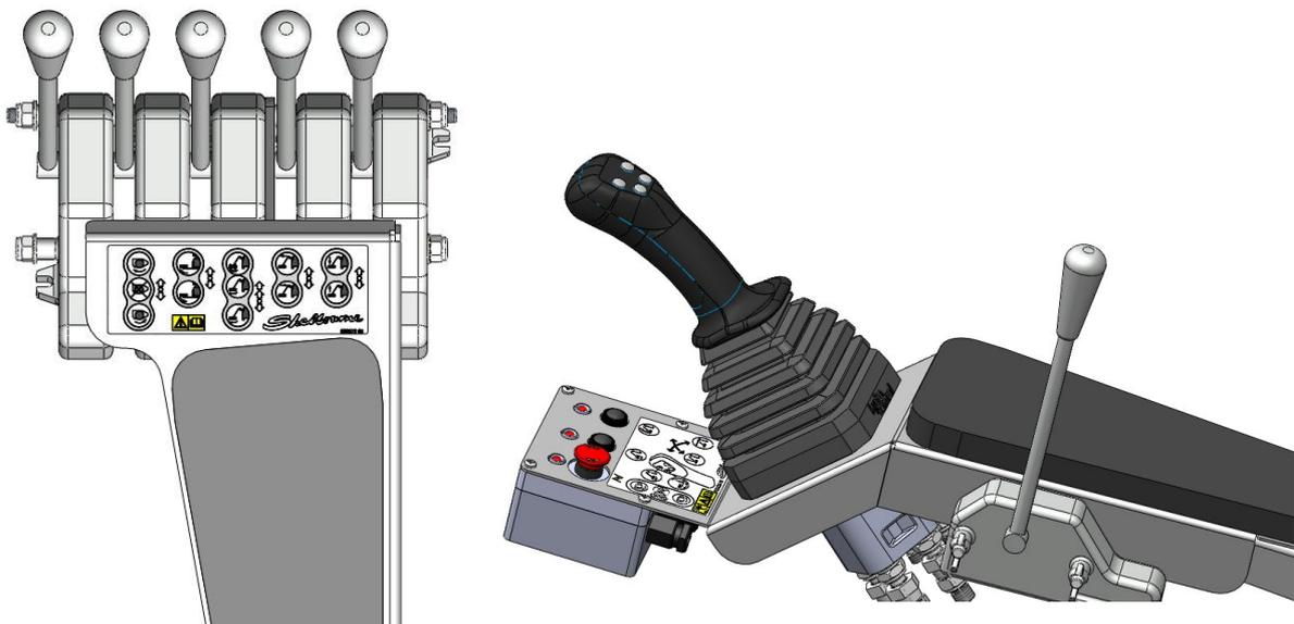
A 12 volt power supply is required for the Oil proportional controls. These must be connected, via a suitable fuse. The power supply must not come from the cigarette lighter, three pin connector or trailer 7 pin socket; due to the oil proportional controls having a high current draw. Low voltage will cause the system to function erratically. Therefore we recommend wiring directly to the tractor battery to guarantee system operation, with the supplied power lead, fuse and connectors.
