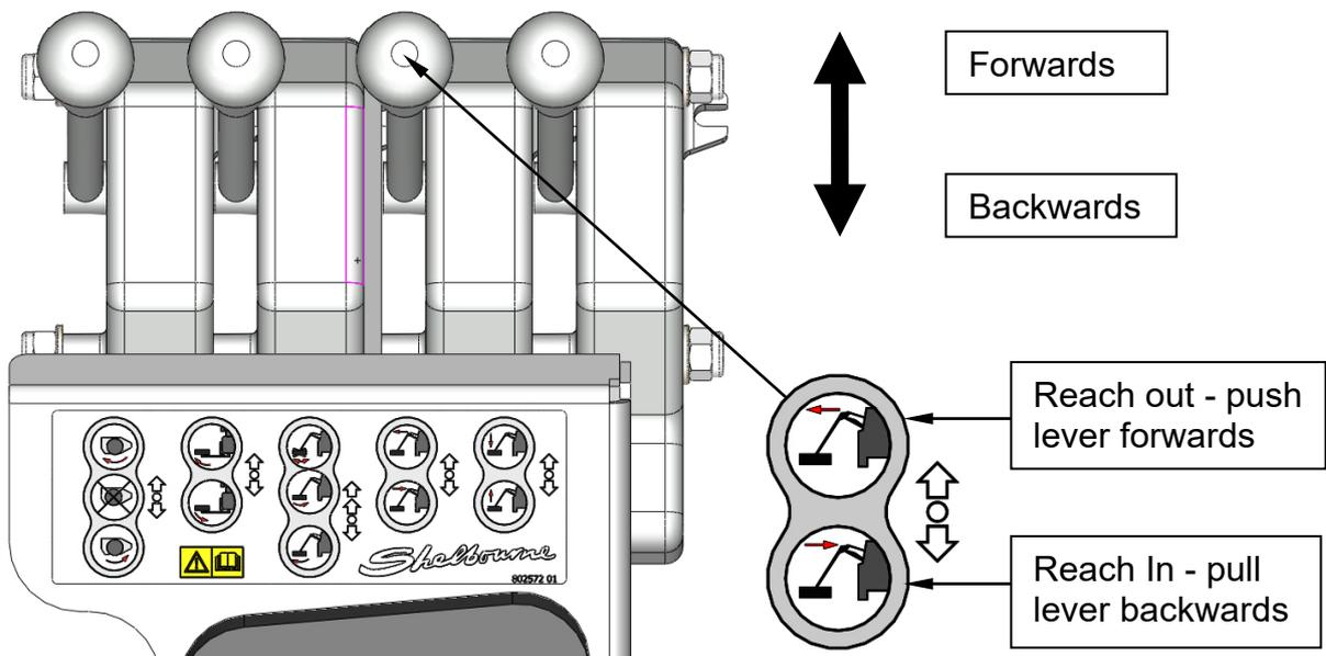
**Head rotation:** By moving the lever forwards and backwards from the operator gives head rotation anti-clockwise and clockwise respectively for the operation of the head rotation service.
