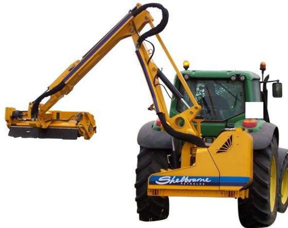
3. 400 models slew the machine fully backwards, so that the booms are directly behind tractor. For 300 models machines bring the booms as close as possible to the tractor tire without contact.
