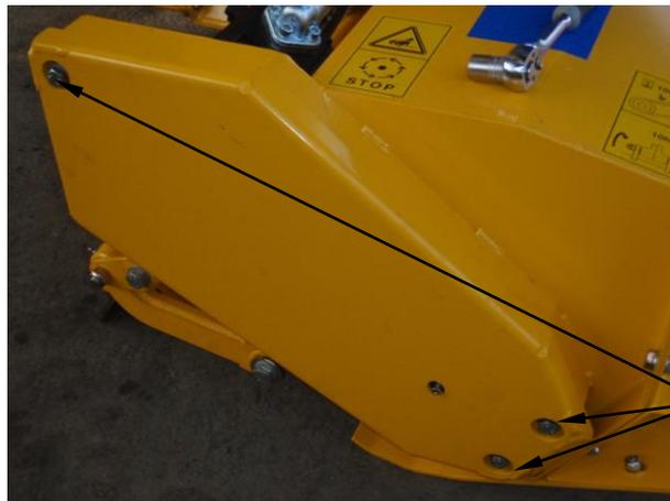
Loosen fixings to remove drive cover
