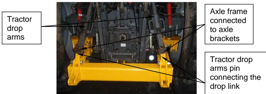
9. Follow the previous procedure up until step 5. Then using suitable lifting equipment connect the axle frame into the axle brackets as picture above.
