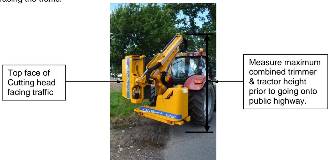
It is recommended to disconnect all electrical, hydraulic connections and the PTO driveshaft from the Powerblade so that it cannot be inadvertently operated during road transport.
