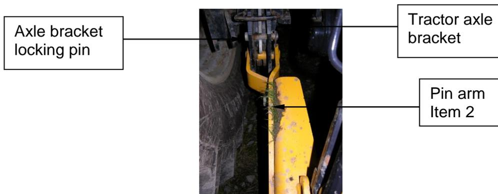
5. Once frame is connected to axle bracket lower drop arms until top link (in position B) becomes unloaded.
