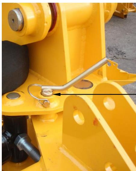
Slew locking device locking the slew cylinder during 'trans
