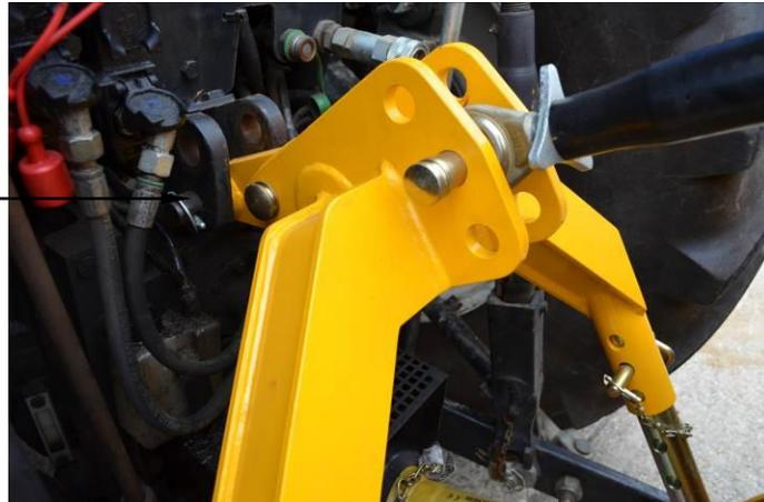
9. Fit the top link (item 13) between the trimmer main frame and the 3 point yoke using the pins and lynch pins provided. Ideally maintain a straight line through the pivot points once in the raised position.
