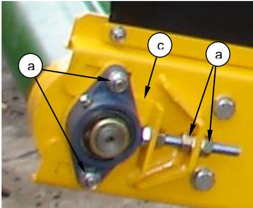
With the belt slack mark 2 lines 500mm apart on the topside of the belt, along each edge. Tension the belt until the 2 lines have stretched from 500mm to 503mm apart.
