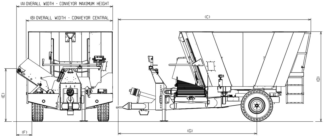
Above machine supplied with single axle fitted with 305/55R22.5 tyres
