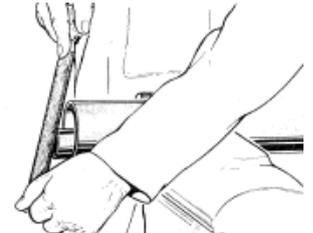
Remove all sharp edges and burrs, grease the sliding . Profile tubes
