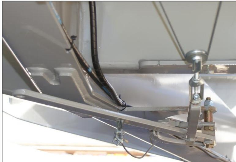
Twin auger models (16-25 m<sup>3</sup>) are supplied with a Rotary spindle type handbrake (See below). To apply the handbrake, simply rotate the crank handle clockwise to tighten the cable which in turn will activate the brake.
