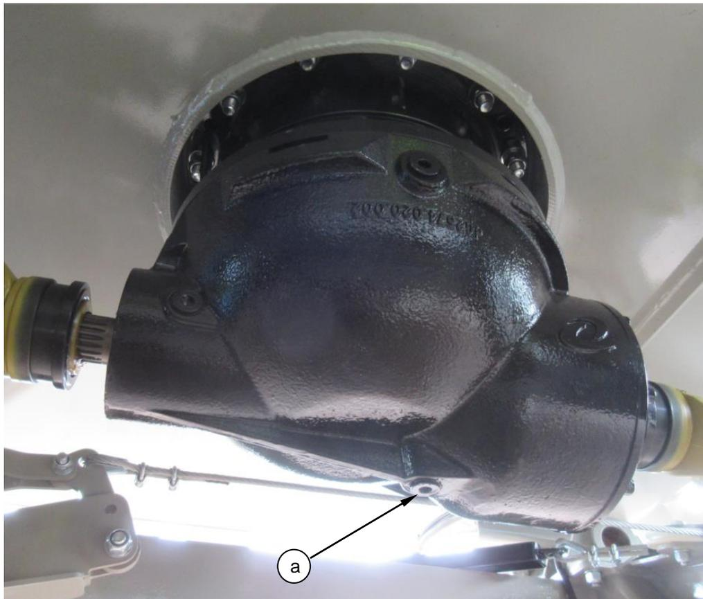
The planetary gearbox contains 2 taper roller bearings. These are positioned in the housing above the oil level of the gearbox. Although the bearings are sealed and pre-packed with long life grease, a small amount of long life grease should be applied every 600 hours (or twice a year).
