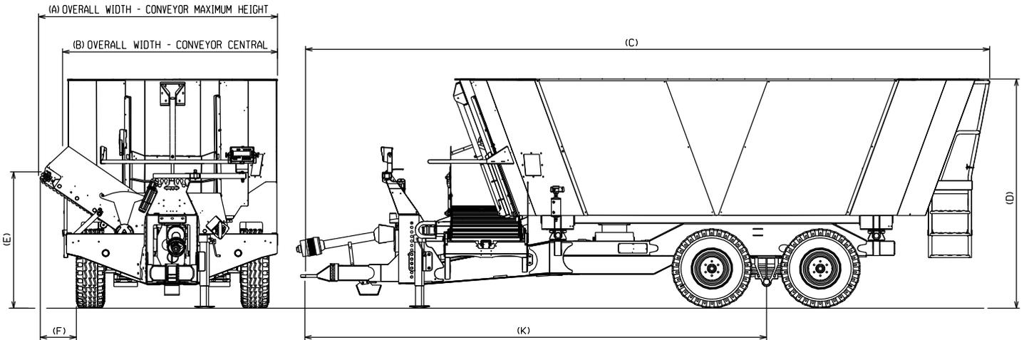
Above machine supplied with sprung loaded tandem axle fitted with 385/55R22.5 tyres.
