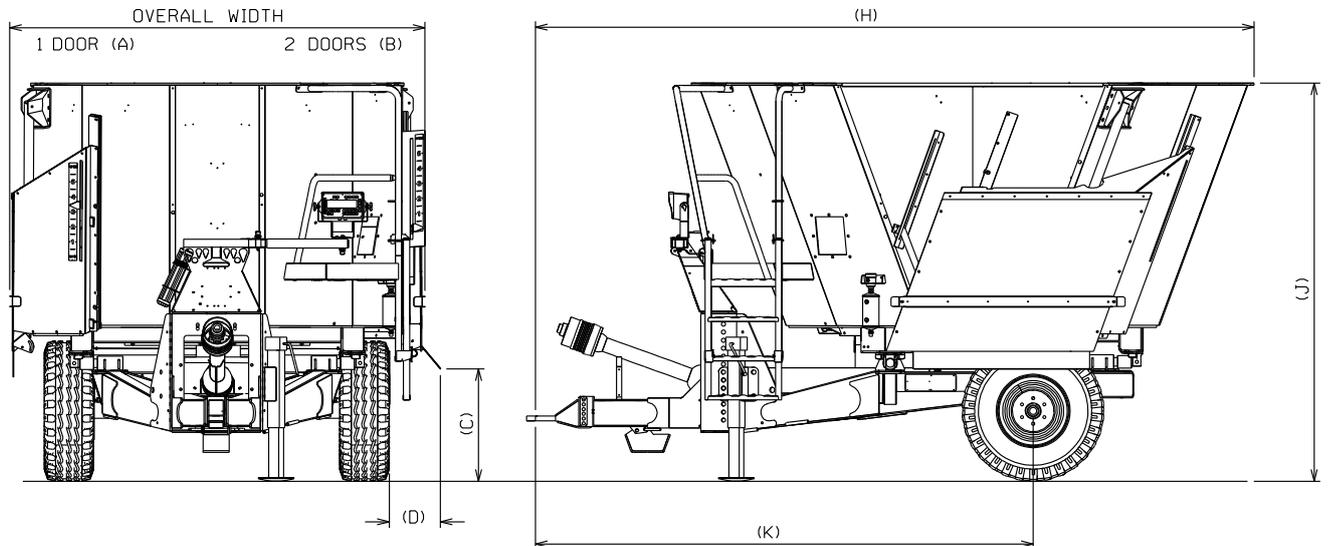
Above machine supplied with single axle fitted with 305/55R22.5 tyres
