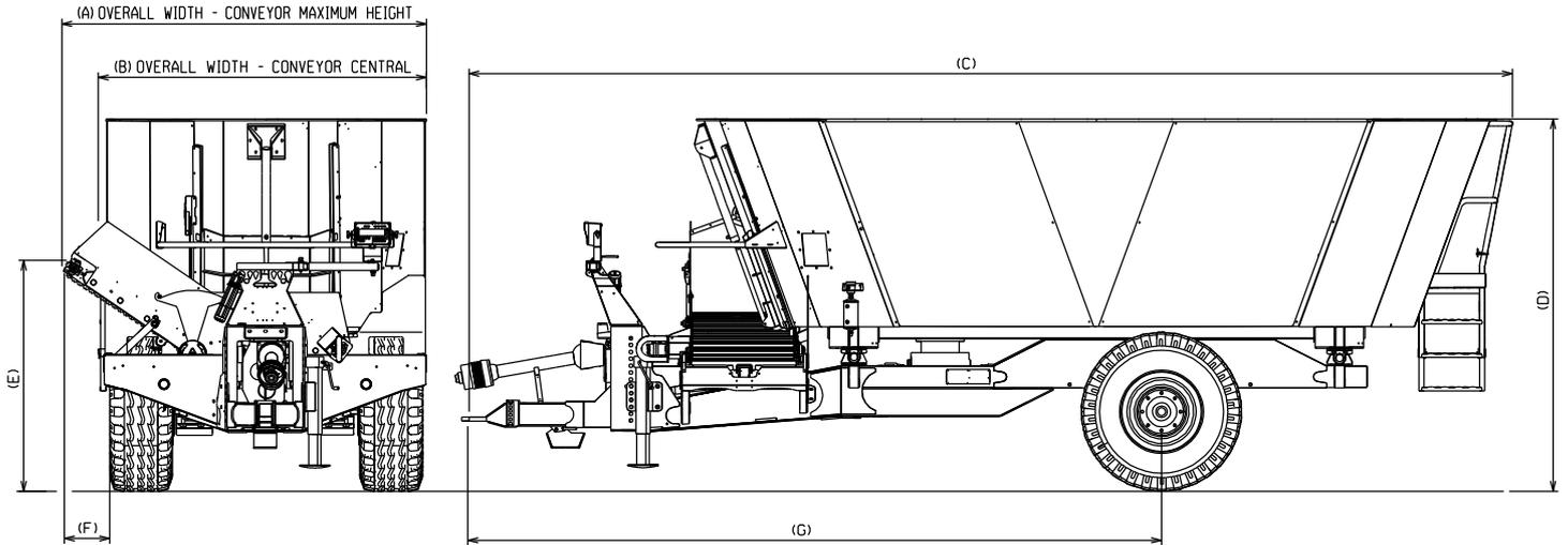
Above machine supplied with a single axle fitted with 18R22.5 or 435/50 R19.5 tyres.
