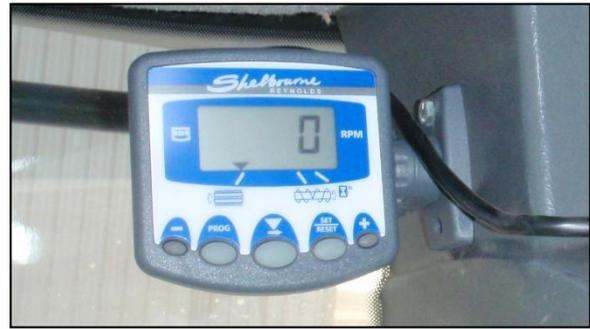
Assemble the two brackets, and mounting plate with clamping knobs, and attach to the head unit. Each pivot point on the mounting bracket can be indexed to angle the head unit in relation to the mounting plate.
