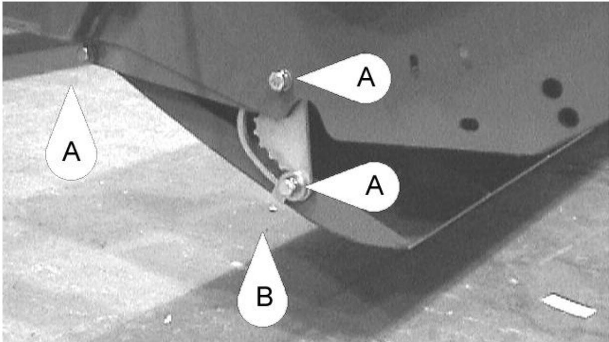
The skids under the *Shelbourne* Header are adjustable FIG 2, and can be moved by slackening off the 6 bolts (A) on each skid, and using a 24mm (15/16") open end spanner (B) as shown, rotate the cam plates in the slots to the required position. Tighten the bolts.
