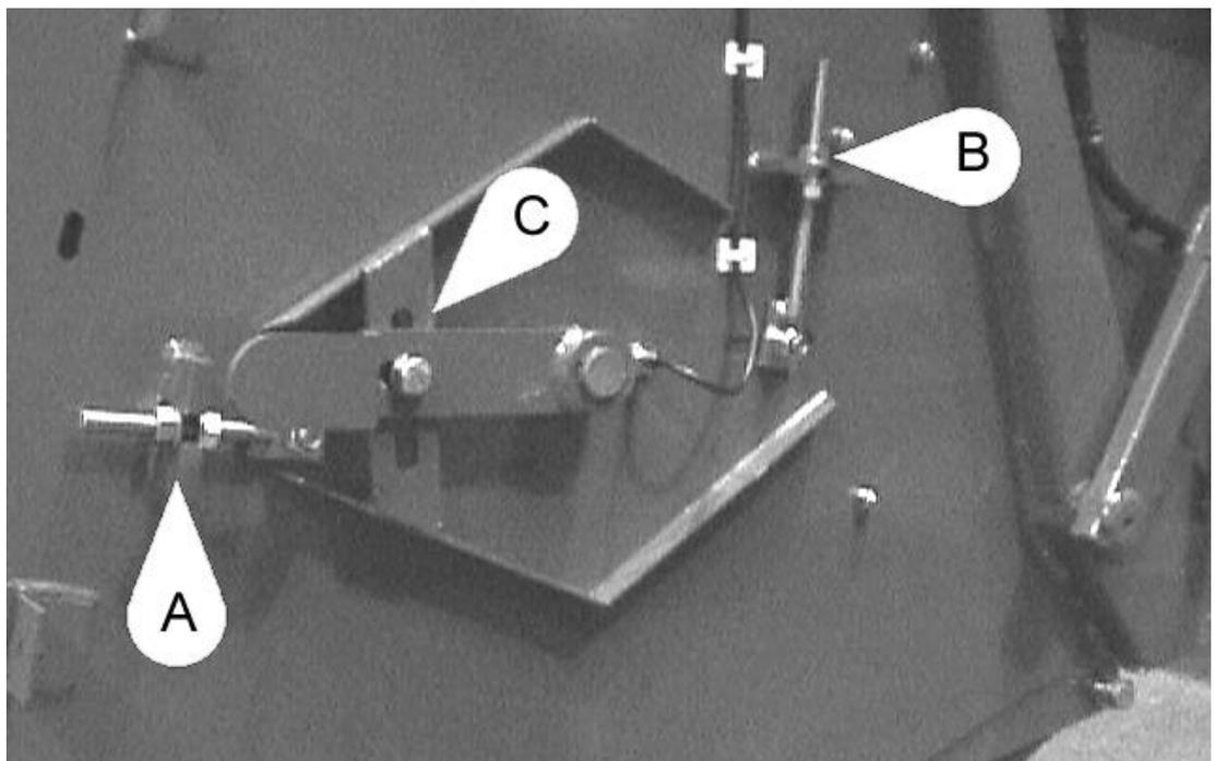
1. To **move up or down**, slacken off the auger support plate locking bolt and adjust stud 'B' as indicated. Adjust both ends of the auger equal amounts.
