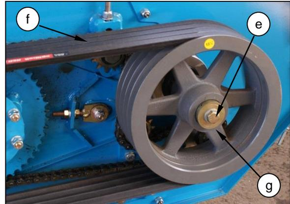
5. If the desired speed is obtainable by swapping the input pulley then change the pulley and reassemble.
