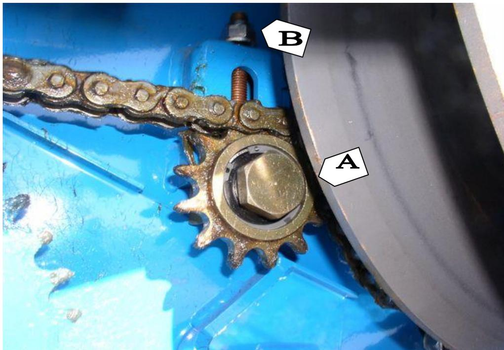
Over tensioning could result in auger drive shaft failure/damage.
