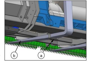
straps (a) and underneath the forklift support plates (b). This will ensure that the tine does not contact the stripping rotor. Use a piece of wood to prevent the rear of the tine carriage contacting the adaptor plate.
