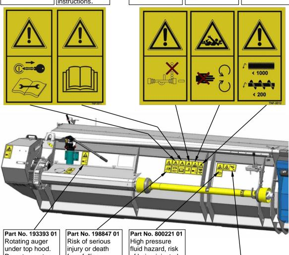
Do not open top hood whilst engine is running. Failure to comply could result in death or serious injury.
