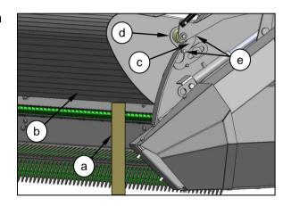
Charge the crop deflector hydraulic system and raise the crop deflector by operating the combine's reel raise function. Remove support (a), then fully lower the crop deflector by operating the combine's reel lower function.
