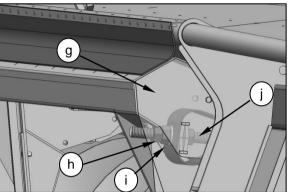
Once the required pitch has been achieved adjust inner nuts (j) to the adaptor plate and tighten outer nuts (i) fully. Tighten lock nuts (h). Ensure that the adjustment is the same either side of the adaptor plate. If the Stripper Header needs to be pitched down follow the same procedure, except wind nuts (h, i & j) towards the combine. Do not unthread the nuts off of the bolt as this will cause the Stripper Header to fall.
