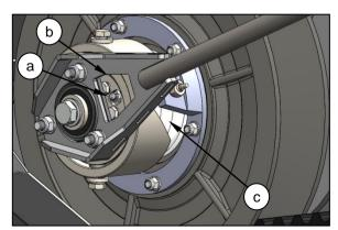
Remove the left hand drive guard and rotate the pulley until the grease point (a) is aligned with the hole in the tie rod (b). Grease the rotor pulley until fresh grease is expelled through the breather hole into the spring area (c).
