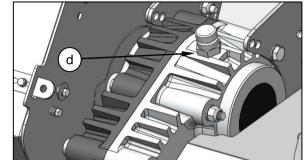
Remove the breather filler cap (d) and then remove the drain plug (e) and drain the oil into a suitable container. Dispose of the oil correctly and safely.
