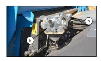
Remove the coupler (g) from its storage bracket (j) on the header and clean both multicoupler faces.
