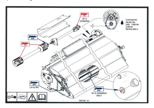
An additional decal is fitted to CVS and RVS machines that indicates the grease points on the variable speed drive pulleys and is located under the left hand drive guard.
