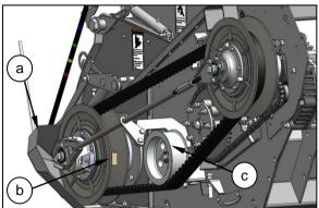
**8.** Ensure that the wooden block is wedged securely between the rotor pulley sheaves and remove the belt, first from the rotor pulley, then from the gearbox pulley.
