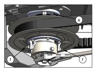
**6.** Left hand end auger bearing (Where grease facility is fitted).
