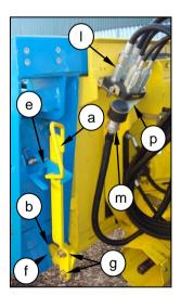
To connect the combine hydraulic quick coupler (I) to the header multicoupler (h), open the cover (j), then depress the red button (k) and raise the handle (n) up to the "fully open" position.
