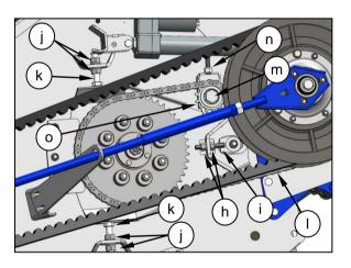
Adjust the auger at the other end, ensure the nuts (h & j) are fully tightened and refit all guards.
