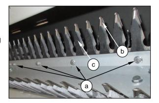
Place the new section in position, ensuring formed cups are pointing in the correct direction. If it is difficult to push into the rotor, it may be tapped into place with a small bar in the bottom of the keyhole.
