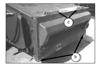
Raise the feeder house to lift the header, ensuring that the pivot blocks (c) are properly seated in the pockets (e) in the adaptor plate top beam, then fully raise the header.
