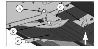
Lower the skid to the desired position and then refit bolt (b) aligning it with the required
