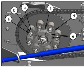
Replace the clutch plates with two new ones, ensuring the four pegs locate into the clutch hub (f) and drive disc when refitted. Fit the nuts and washers and adjust as described above.
