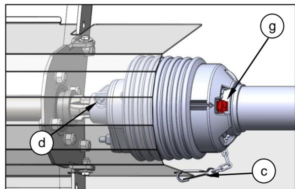
The guard should slide away from the shear bolt clutch allowing access to change the shearbolt. It may still be necessary to remove the PTO shaft from the Stripper Header input shaft.
