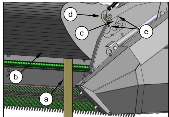
Undo the M6 fasteners (e) that secure the plate (c) to the horse shoe plate (d).
