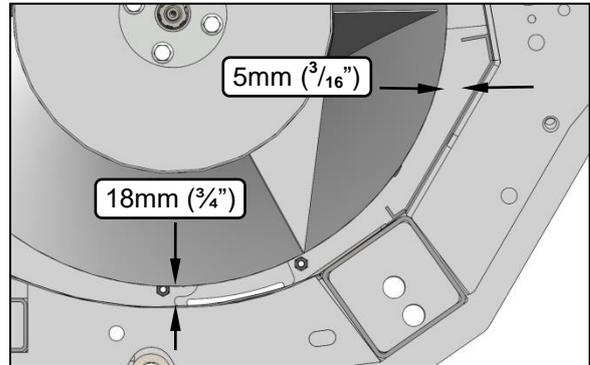
Check the auger flight clearance. There should be a gap of 18mm ( $\frac{3}{4}$ " ) between the flight and the bottom of the auger trough and 5mm ( $\frac{3}{16}$ " ) between the auger flight and rear scraper.
