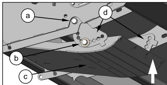
Repeat the process on the other skids, ensuring that both outer skids are adjusted to the same height. Inner skids should be set two positions higher than outer skids.
