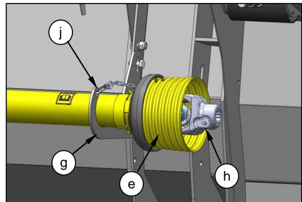
Check that the locking pin or collar has engaged properly on the shaft.
