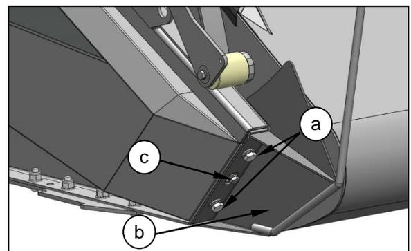
On a CVS repeat this process on the left hand end and ensure the correct handed marker is fitted to the correct end as shown.
