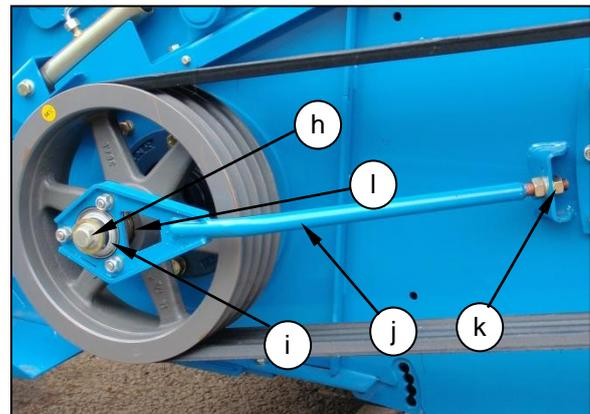
7. Remove the washers and tapered collars (l), remove the pulley, ensure that the inner tapered collar is left on the shaft and not removed. Fit the correct pulley order to get the desired speed.
