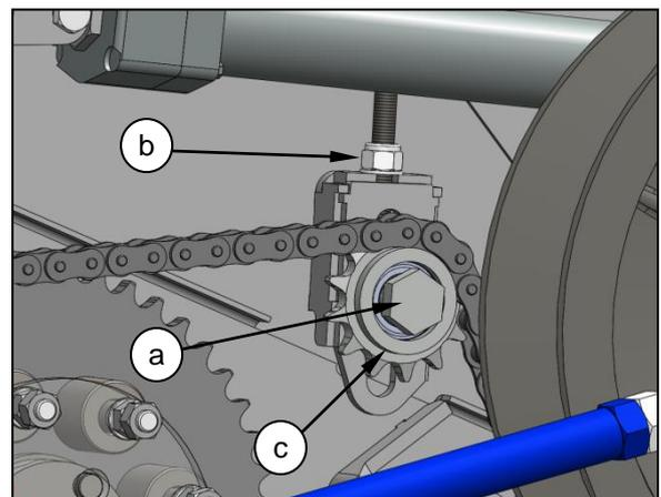
complete, tighten the idler spindle (a), check that the chain tension does not increase as the idler spindle is tightened.
