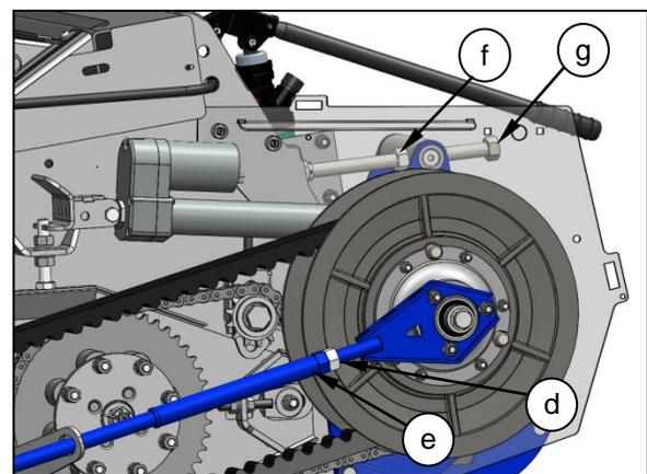
8. Ensure that the wooden block is wedged securely between the rotor pulley sheaves and remove the belt, first from the rotor pulley, then from the gearbox pulley.
