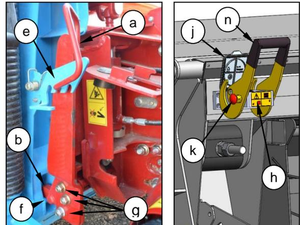
Lift the locking plate (e), pull and lower the handle (a) to disengage the hooks (b) from the pins (f).
