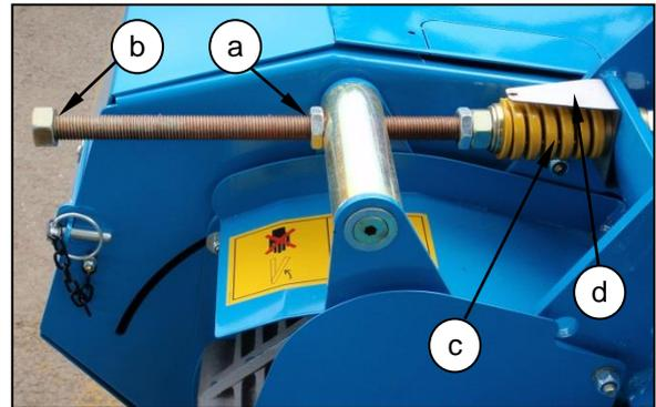
**⚠ Do not over tension the belts as this can damage the drive system**
