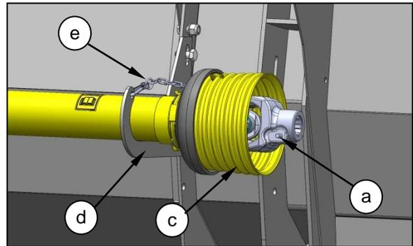
Place the PTO shaft in the storage bracket (d).
