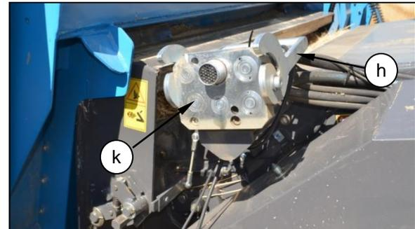
If the combine is not fitted with a multicoupler the hydraulic and electrical couplers will have to be connected separately.
