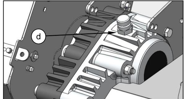
Remove the breather filler cap (d) and then remove the drain plug (e) and drain the oil into a suitable container. Dispose of the oil correctly and safely.
