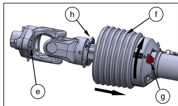
Refit the guard and ensure it has engaged on all three points of the locking collar, rotate the guard anticlockwise, again a screw driver may be required to pry the locking collar, then refit the red retaining clip.
