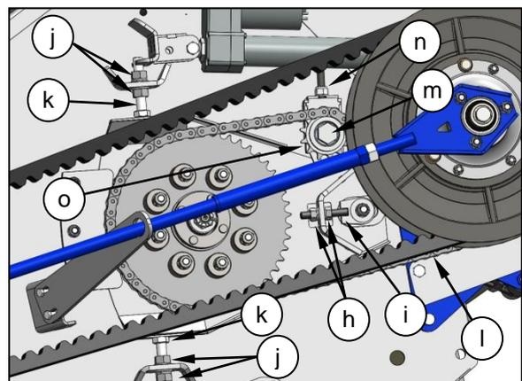
To move the auger up and down, wind the nuts (j) on the setscrews (k).
