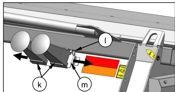
Fit one header stand (k) to both front corners (underside) of the Stripper Header, slide the header stand forwards, onto the dividing plate (n) from the rear of the machine. Secure in position by fitting the linchpin (l).
