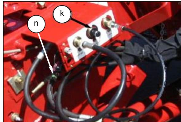
Connect the header 3 pin electrical cable connector (m) to the combine electrical connector (n).
