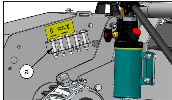
On RVS and RSD machines the shearbolts (b) are located on the rear left hand end of the mainframe, beside the hand pump.
