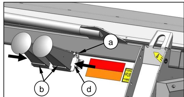
Remove the feeder house cylinder lock.
