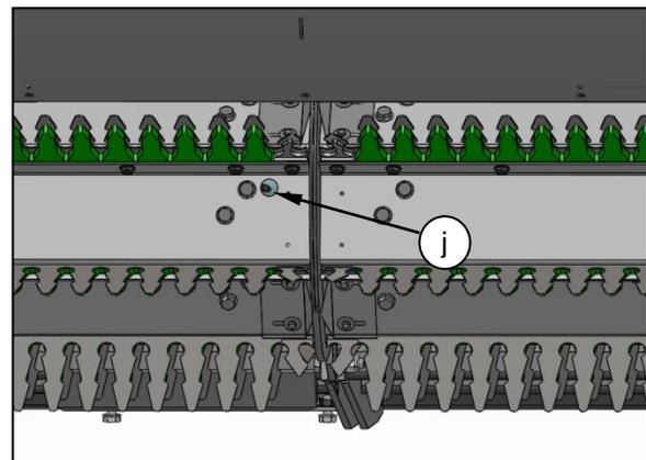
Refit the grease hole plug.
