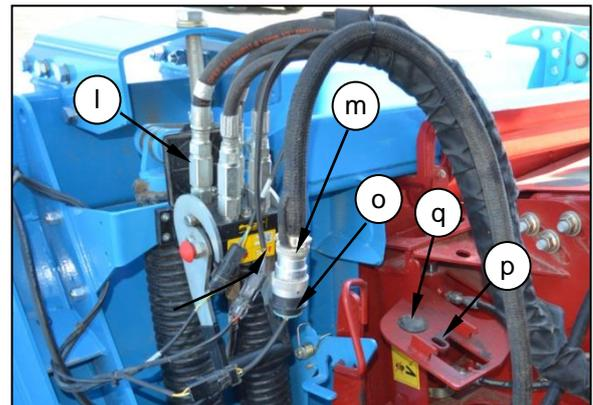
Depress the red button (k) on the header multicoupler (h) and raise the handle (n) to release the combine quick coupler (l).
