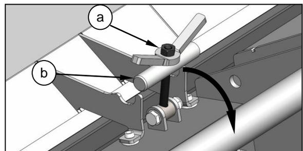
Open the hood. To do this, unwind (anticlockwise) the two retaining nuts (a) and release the retaining bars (b).
