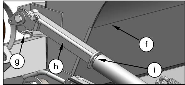
Check that there is clearance between the auger flight and paddles and the combine feeder house. If this is too close then the adaptor plate may need to be adjusted as described in Section 6.5.
