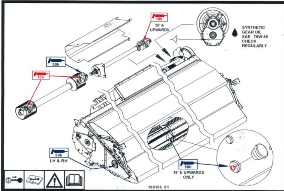
An additional decal is fitted to CVS and RVS machines that indicates the grease points on the variable speed drive pulleys and is located under the left hand drive guard.
