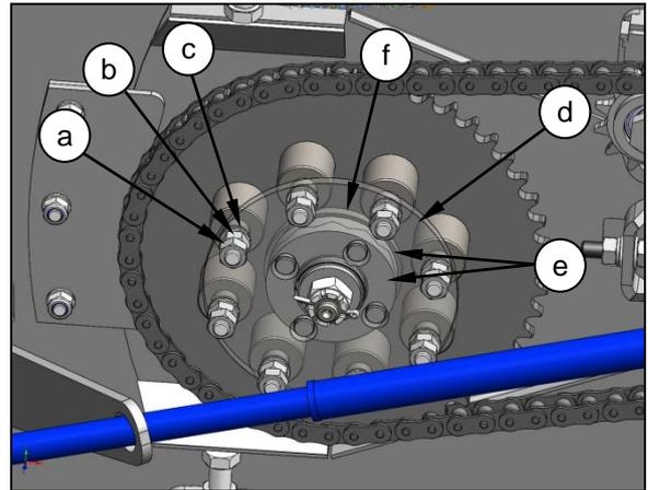
Replace the clutch plates with two new ones, ensuring the four pegs locate into the clutch hub (f) and drive disc when refitted. Fit the nuts and washers and adjust as described above.
