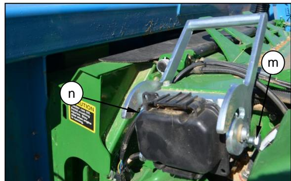
Push up the multicoupler handle (a) to the "nearly up position", remove the plastic cover (n) from combine multicoupler (e) and clean the multicoupler face.
