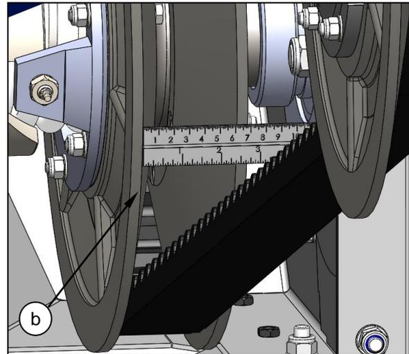
4. To achieve the correct gap adjust the idler pulley (c). Raising the idler will reduce the pulley gap and vice versa. To adjust the idler, slightly slacken the idler bolt (d) and then turn nut (e). Once the idler is adjusted tighten the idler bolt (d).
