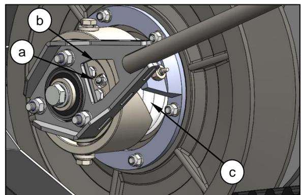
Remove the left hand drive guard and rotate the pulley until the grease point (a) is aligned with the hole in the tie rod (b). Grease the rotor pulley until fresh grease is expelled through the breather hole into the spring area (c).
