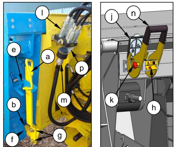
Lift the locking plate (e), pull and lower the handle (a) to disengage the pins (f) and the hooks (b).
