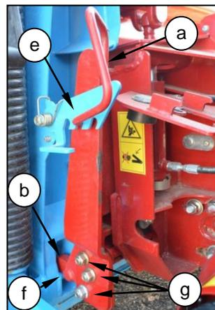
If the hooks (b) do not fully engage the pins (f) on the adaptor plate when the handle (a) and the locking plate (e) are engaged, loosen the bolts (g) and adjust the hooks as required, so that some resistance is felt when the locking plate (e) is engaged with the handle (a). Retighten bolts.
