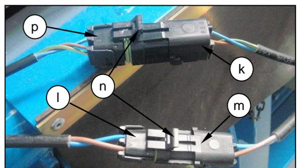
CVS and RVS Stripper Headers have an additional two pin plug (l) and socket (m) which needs to be connected, to supply power to the variable speed linear actuator.
