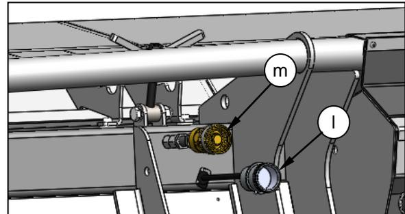
Connect the PTO shaft and monitor electrical connectors. Then remove the header stands, as described in Section 5.1.10.
