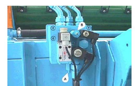
Note – On top of the auger drive motor there is bolted a cross line relief valve unit. This is to protect the auger motor from over pressurising when shuttling from forward to reverse rotation. It is pre-set and must not be adjusted.
