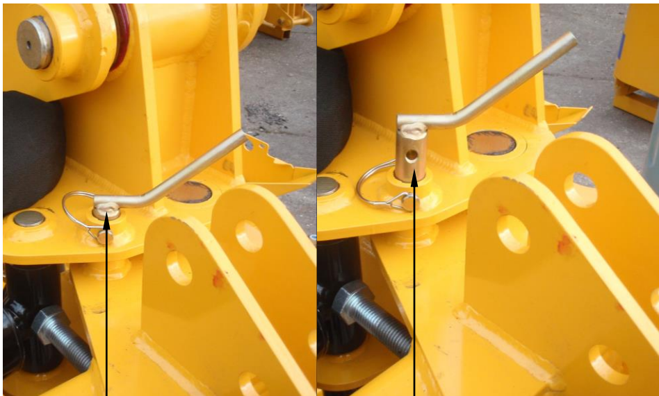
Slew locking device locking the slew cylinder during 'transport'
