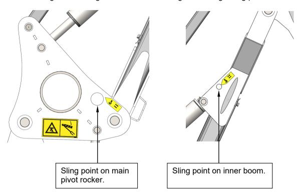
Ensure lift cylinder taps are closed before lifting commences and slew locking device is fitted (400 models) see section 7.
