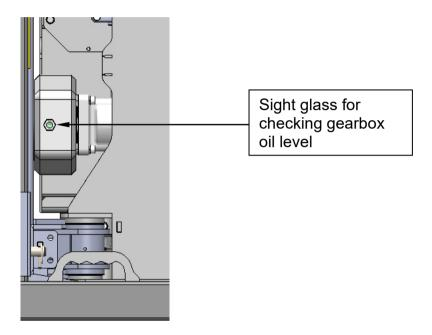
To minimise contamination – Ensure that any oil, containers and funnels used to top up the system are scrupulously clean and that the filler area is cleaned thoroughly before removing the cap. Follow the stated change intervals for the return and suction filters. When undertaking repair or servicing keep all components scrupulously clean. Ensure the filler cap and breather are intact and always kept in place (moisture is a contaminant as well as dirt).
