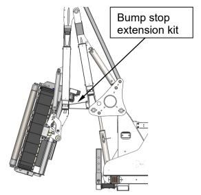
4. For 400 models use the slew cylinder to rotate the arms fully back, and then position the cutting head with the flail facing the operator and the top of the cutting head towards the traffic.
