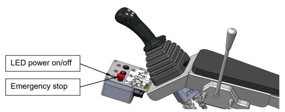
**Lift & Reach:** By moving the joystick to the left and right the reach cylinder is actuated in the relevant direction; moving it back/towards and forwards/away from the operator gives lift and lower respectively. These actions are proportional; that is small joystick displacements give slow cylinder movements and large displacements faster movements.
