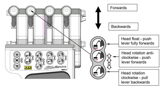
**Rotor up cut**: Engage the cutting head rotor in the up cut direction by moving the lever backwards.
