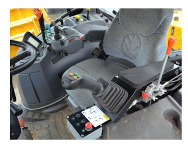
The Powerblade 300 and 400 series trimmer ranges have two types of control system. Cable levers controls or Oil proportional controls.
