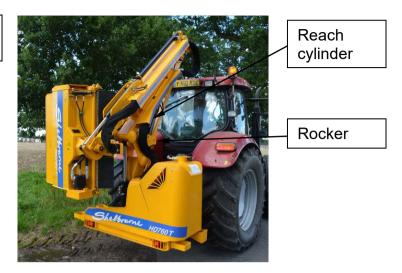
Use the lift, reach and head angling cylinders to bring the head to a position near to the tractor, parallel to, and close to the ground.
