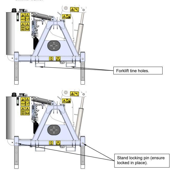
Insert the tines as far as they can go, to get the trimmer as close to the forklift as possible.
