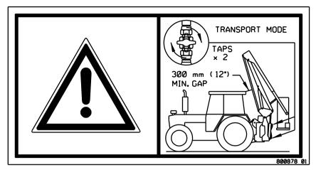
10. For 400 models the slew cylinder should be mechanically locked by the slew locking device being put in place during all transportation on the public highways.
