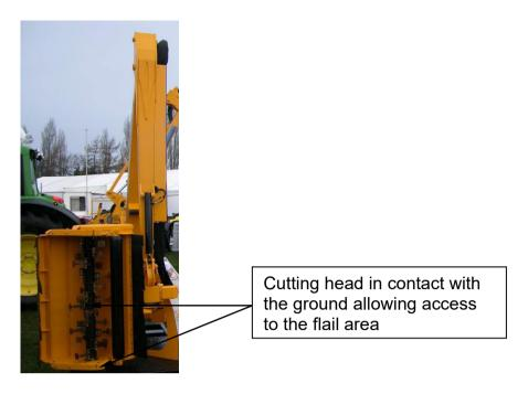
Ensure that there is nothing wrapped around the rotor or roller.
