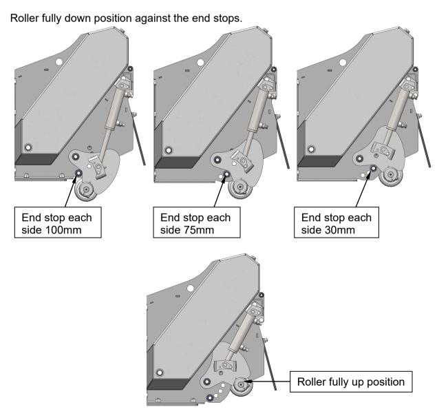
Adjustment of the end stops position should be done when the roller is in its fully up position.
