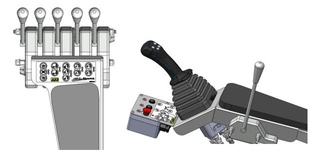
A 12 volt power supply is required for the Oil proportional controls. These must be connected, via a suitable fuse. The power supply must not come from the cigarette lighter, three pin connector or trailer 7 pin socket; due to the oil proportional controls having a high current draw. Low voltage will cause the system to function erratically. Therefore we recommend wiring directly to the tractor battery to guarantee system operation, with the supplied power lead, fuse and connectors.
