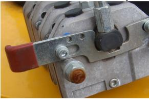
• Engage rotor in the up cut direction.
