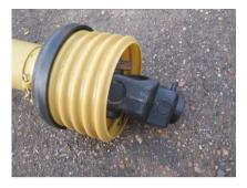
Connect the pull release yoke end to the tractor.
