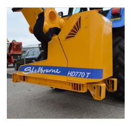
15. Point 13 and 14 should be repeated once the trimmer is fully operational. In some cases it's also required to place the head horizontal to the ground, close to the tractor tyre in the work position power the booms into the ground. This may then allow further adjustment to the tractor check chains and drop arms if required.
