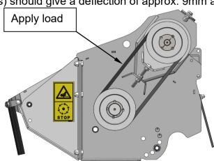
To adjust, slacken the nuts at the motor fixing bolts and the adjuster locknut, then turn the adjuster bolt in the required direction. Then tighten lock nut and fixing bolts and replace the drive cover.
