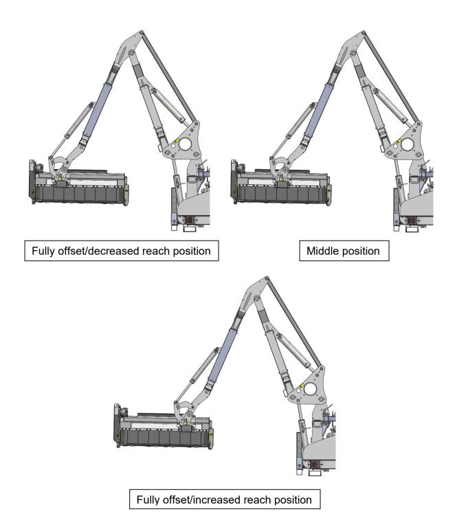
To adjust the sliding head, position the cutting head vertically in contact with the ground. Perform a 'SAFE STOP' procedure before leaving the tractor seat. Loosen the four bolts on the clamping bracket. Return to the tractor and using the lift service move the clamp bracket along the box section to the desired position. Perform a 'SAFE STOP' procedure before leaving the seat. Tighten the four bolts on the clamping bracket.
