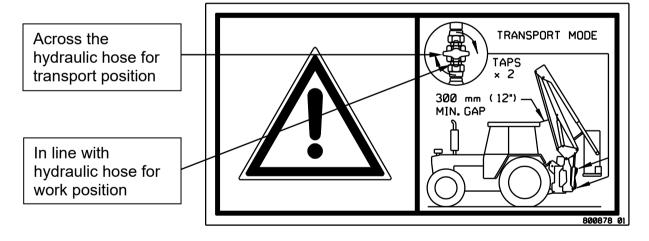
• Extend the reach cylinder so that when the slew cylinder is extended the trimmer head misses the tractor wheel/cab. Extending the slew cylinder will rotate the arms to the work position. 300 models are already in the work position.
