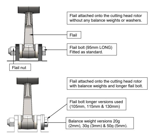
Replace spacers, bolts and nuts exactly when replacing flails. The flails themselves should wear evenly and be replaced as a set. Should one flail be lost then the flail at 180°, one place along should be renewed at the same time to preserve the balance.
