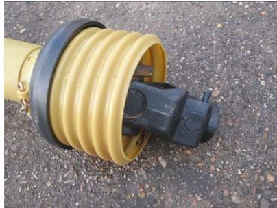
Connect the pull release yoke end to the tractor.
