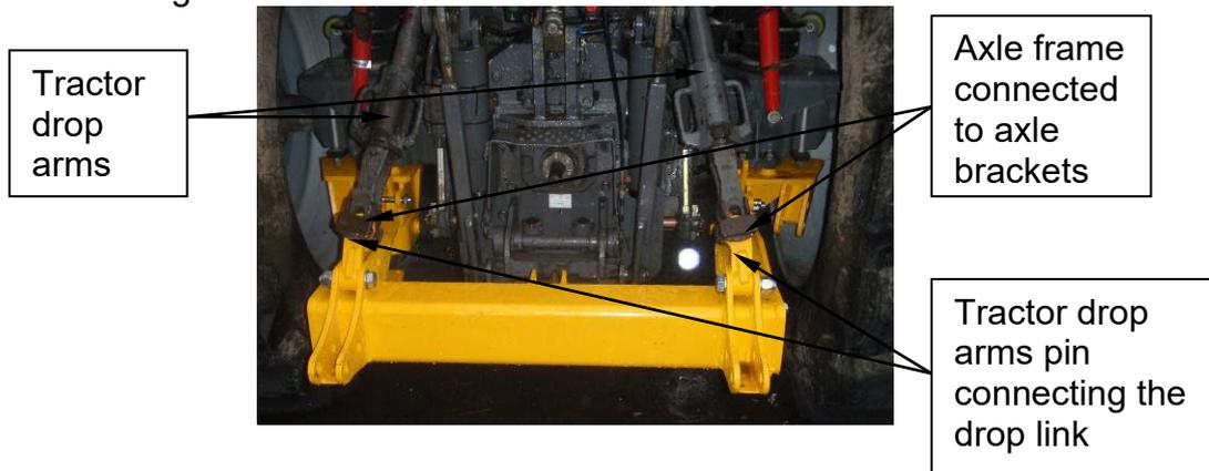
9. Follow the previous procedure up until step 5. Then using suitable lifting equipment, connect the axle frame into the axle brackets as picture above.
