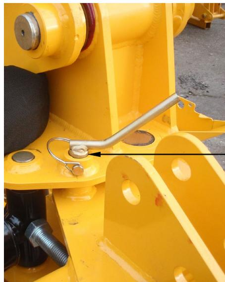
Slew locking device locking the slew cylinder during 'transport'
