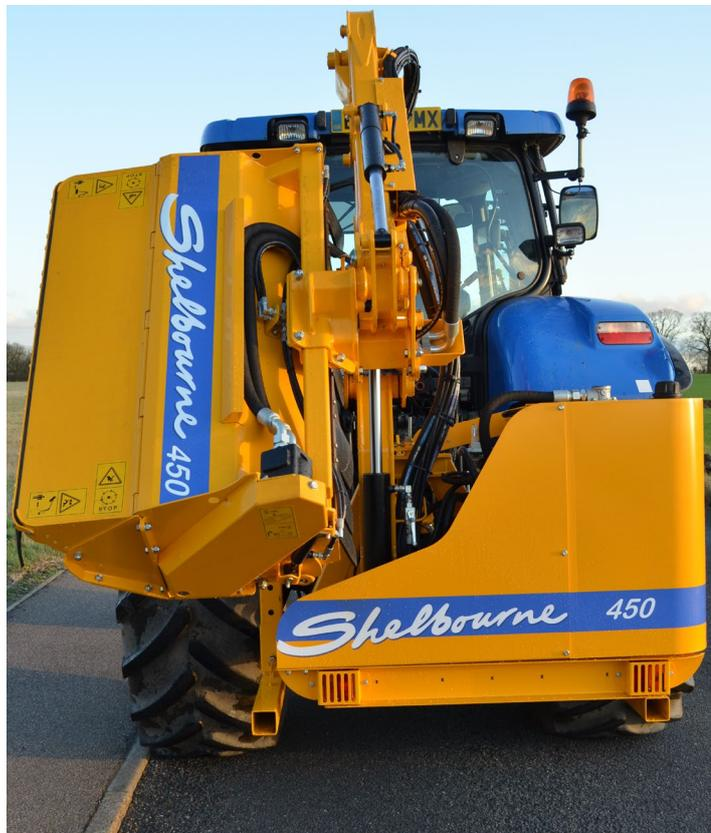
5. The reach cylinder can now be fully closed bringing the outer booms onto the bump stop on the inner boom.
