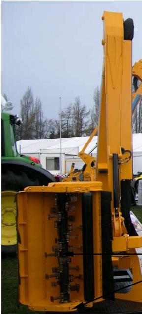
Cutting head in contact with the ground allowing access to the flail area
