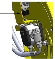
To ensure the fan is running smooth turn the tractor spools flow down to between 20 – 30 l/min or if the fan blower is hunting turn the tractor spool flow down until it runs smooth. Excessive tractor flow may cause heat build-up for both the tractor and the debris blower.
