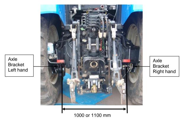
Shelbourne Reynolds axle brackets supplied will be accompanied by the axle bracket parts and operators manual (MAN-10104) which will include specific instructions on how to fit the axle brackets to specific tractors.
