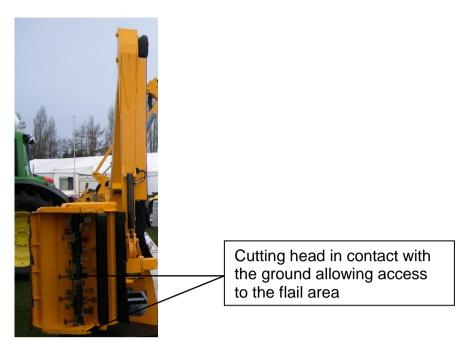
Ensure that there is nothing wrapped around the rotor or roller.
