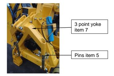
14. Remove the top link pin between the tractor and 3-point linkage rocker. Then swing the 3 point assembly away from the tractor towards the trimmer main frame. Reposition the rocker (item 8) from the front of the 3 point yoke to the rear enabling it to connect between the trimmer main frame and the 3 point yoke.
