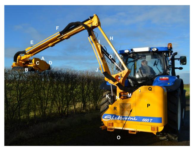
A fully independent PTO operating at 540 rpm, with a 1 & 3/8" SAE 6 spline shaft and rotating in a clockwise direction is required.
