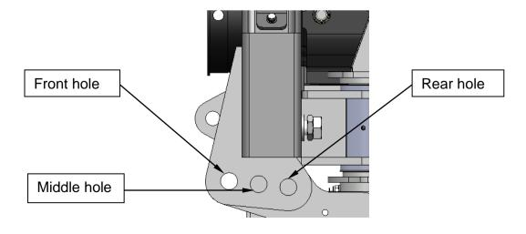
Note: Some tractor lift arms may not be compatible to use the rear hole if the crank within the lift arm is too great.
