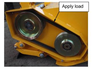
To adjust, slacken the nuts at the motor fixing bolts and the adjuster locknut, then turn the adjuster bolt in the required direction. Then tighten lock nut and fixing bolts and replace the drive cover.
