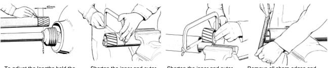
To adjust the lengths hold the half shafts next to each other in the shortest working position and mark them 40mm as shown.
