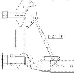
8. The axle frame is now assembled and ready for the tractor to be attached. It's also possible to attach the axle frame assembly to the tractor before then attaching to the Powerblade.
