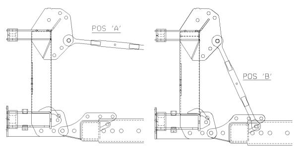
5. Detach the tractor drop arms from the drop links (item 12) by removing the drop link pin.
