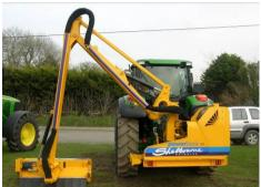
18. Correct adjustment has been reached when with the booms in the work position the machine remains parallel to the rear axle of the tractor. Take tyre squash into account when viewing this.
