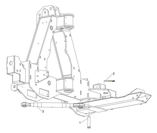
1 Connect the larger diameter end of the adjustable link into the tractor drawbar clevis using the tractor drawbar pin.
