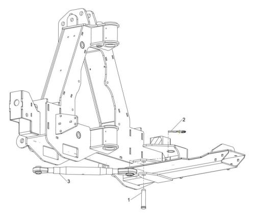
1 Fit item 3 into the clevis incorporated within the trimmer main frame assembly using item 1 and 2. Ensure the smaller diameter end of the adjustable link is fitted into main frame.
