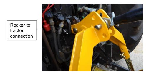
9. Fit the top link (item 13) between the trimmer main frame and the 3 point yoke using the pins and lynch pins provided. Ideally maintain a straight line through the pivot points once in the raised position.
