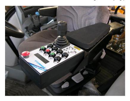
A 12 volt power supply is required for the electrical controls. These must be connected, via a suitable fuse. The power supply must not come from the cigarette lighter, three pin connector or trailer 7 pin socket; due to the electric controls having a high current draw. Low voltage will cause the system to function erratically. Therefore we recommend wiring directly to the tractor battery to guarantee system operation, with the supplied power lead, fuse and connectors.
