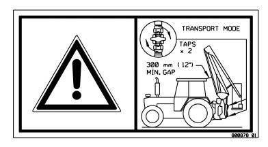
8. Even though the slew cylinder has PO check valves which locks the cylinder hydraulically a mechanical slew locking device should be put in place during all transportation on the public highways.
