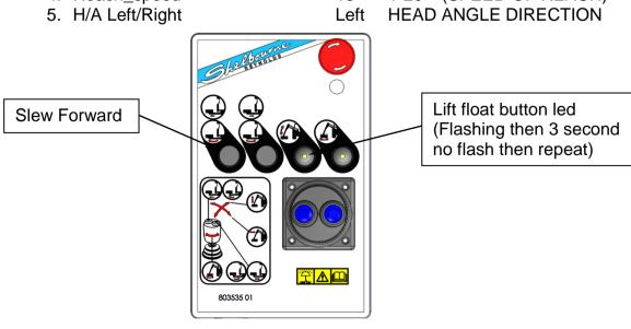
Before adjusting the setting value to another firstly cover the arm float button LED.
