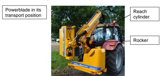
Use the lift, reach and head angling cylinders to bring the head to a position near to the tractor, parallel to, and close to the ground.
