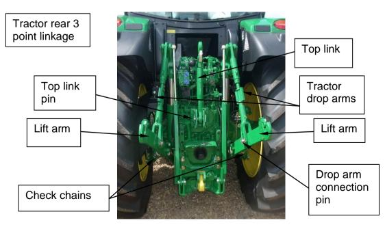
Ensure the tractor drop arms are of equal length ensuring they are kept at the minimum length required while still being able to hitch on the trimmer. Ensure the pin which connects the drop arm to the lift arm is positioned into the fixed rather than the float position (please refer to the tractor operators manual).
