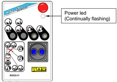
Before adjusting from one function to another (dead band lift & reach, dead band H/A, lift speed, reach speed and H/A) firstly cover the head float button LED. Then pressing the "Slew forward button" (left of the four buttons) will enable you to move from one function to another. The "Lift float button" led will then simultaneously change and flash to indicate which function you're in.
