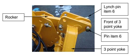
Note: A longer rocker is also available to order from SRE parts part number: 806071 01 if the tractor is not compatible with the standard fitment.
