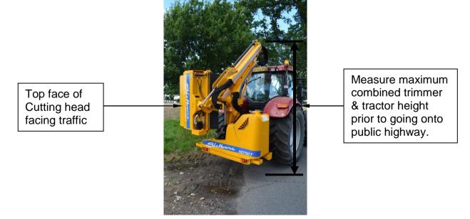
It is recommended to disconnect all electrical, hydraulic connections and the PTO driveshaft from the Powerblade so that it cannot be inadvertently operated during road transport.
