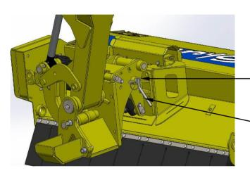
When the narrow lane bracket is not being used it can be locked in its fully closed position by inserting the locking pin using the hole nearest the pin handle.
