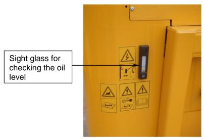
If a biodegradable oil is to be use, please contact Shelbourne Reynolds Ltd with the oil specification to check suitability.
