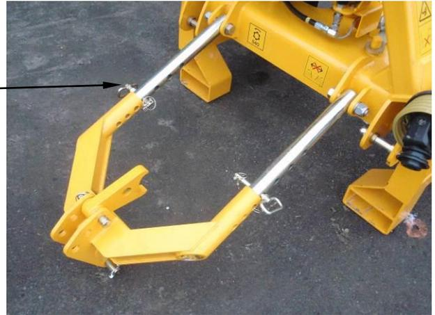
4. Connect item 8 into the middle hole of the three holes in item 7 using pins item 14 & 6.
