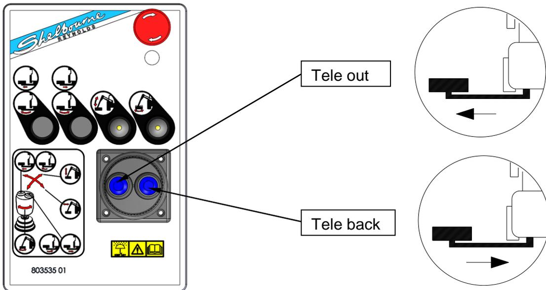
In addition to the joystick, there are 4 additional buttons; each represented by a diagram. Their meanings are detailed below.
