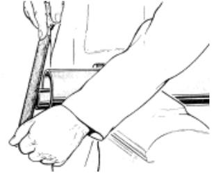
Remove all sharp edges and burrs, grease the sliding . Profile tubes
