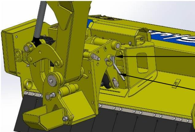
When the narrow lane bracket is not being used it can be locked in its fully closed position by inserting the locking pin using the hole nearest the pin handle.
