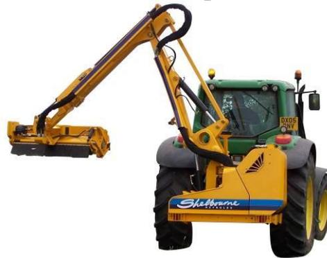
2. Use the slew cylinder to rotate the arms fully back, and then position the cutting head with the flail facing the operator and the top of the cutting head towards the traffic.
