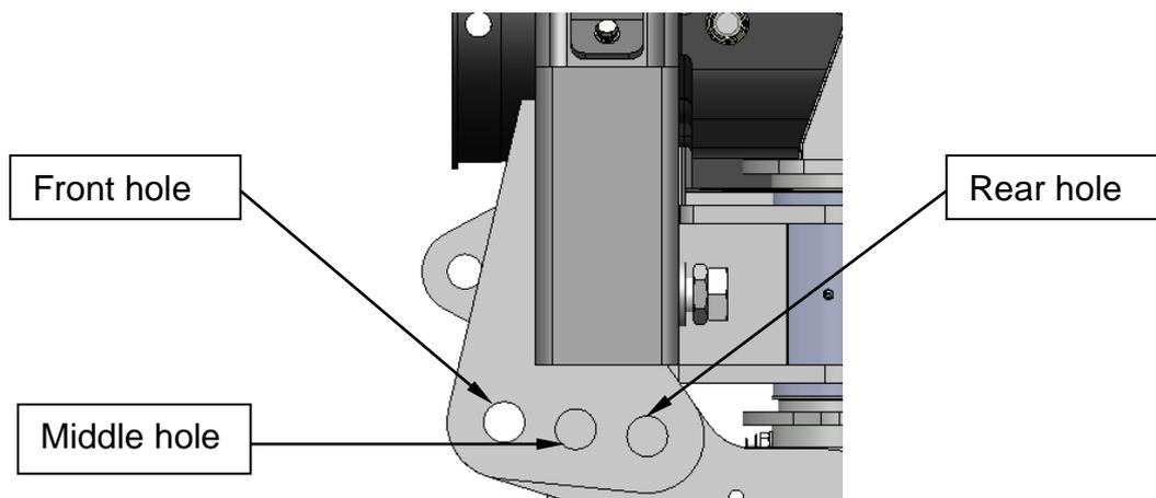
Note: Some tractor lift arms may not be compatible to use the rear hole if the crank within the lift arm is too great.
