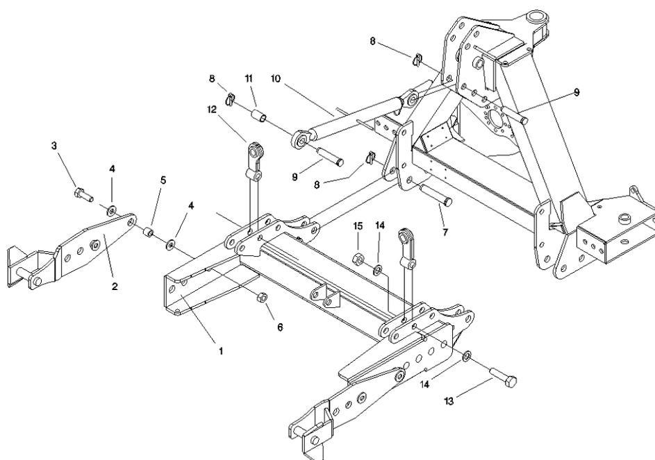
1. Remove the drop arm pin connecting the tractor's drop arms to the lift arms. Lift arms should ideally be removed or otherwise secured so that they cause no obstruction.
