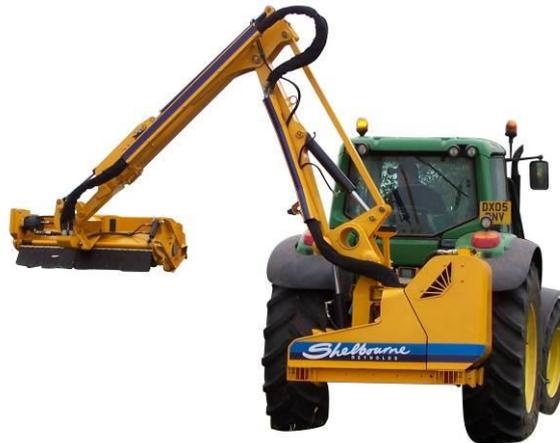
3. Slew the machine fully backwards, so that the booms are directly behind the tractor.
