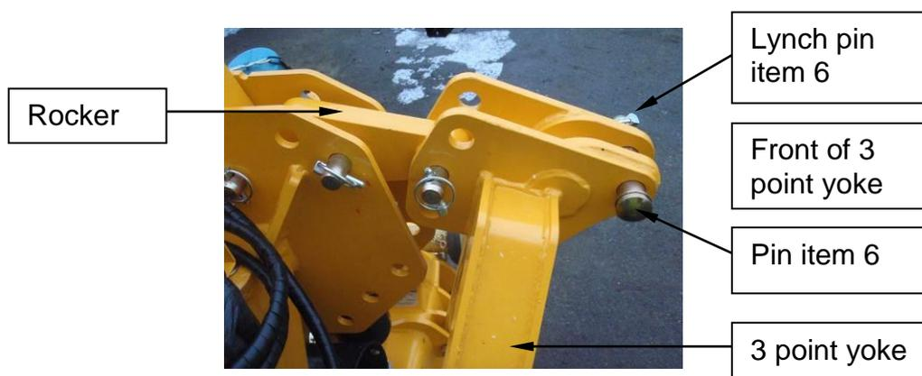
Note: A longer rocker is also available to order from SRE parts part number: 806071 01 if the tractor is not compatible with the standard fitment.
