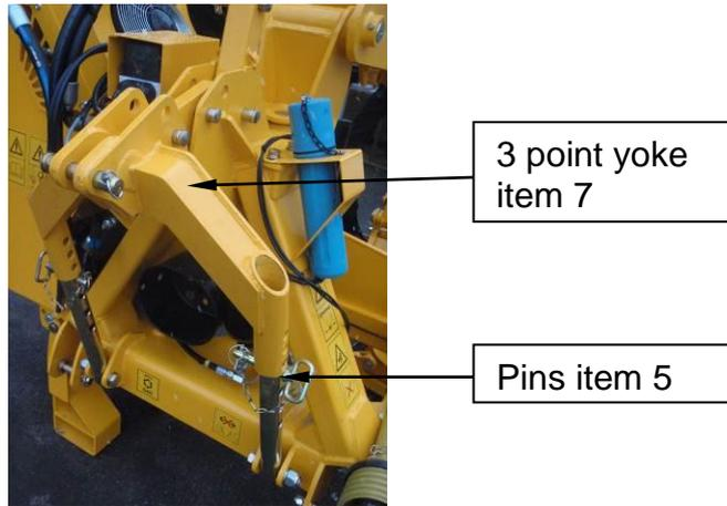
14. Remove the top link pin between the tractor and 3-point linkage rocker. Then swing the 3 point assembly away from the tractor towards the trimmer main frame. Reposition the rocker (item 8) from the front of the 3 point yoke to the rear enabling it to connect between the trimmer main frame and the 3 point yoke.
