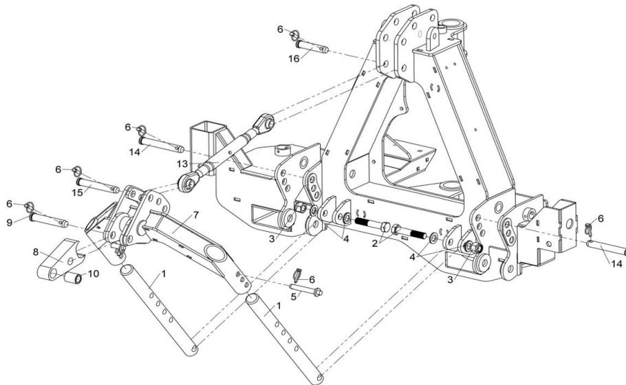
1. Identify if the tractor has lift arms with fixed ball ends or has a quick release ball end style. For Lift arms with the fixed ball ends prepare the pin, lynch pin and spacers
