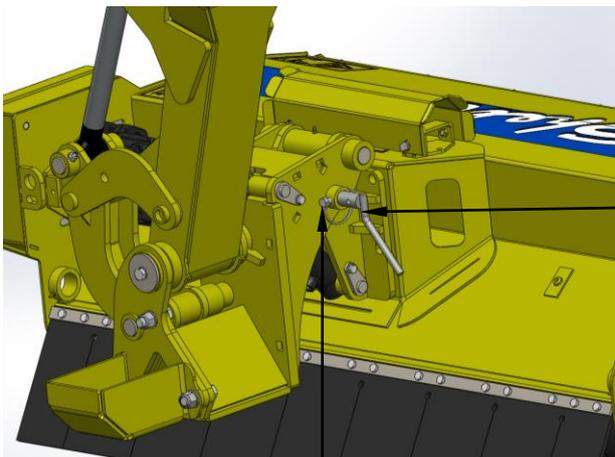
To unlock the narrow lane bracket with draw the locking pin, then fit the retaining pin in the locking pins second hole.
