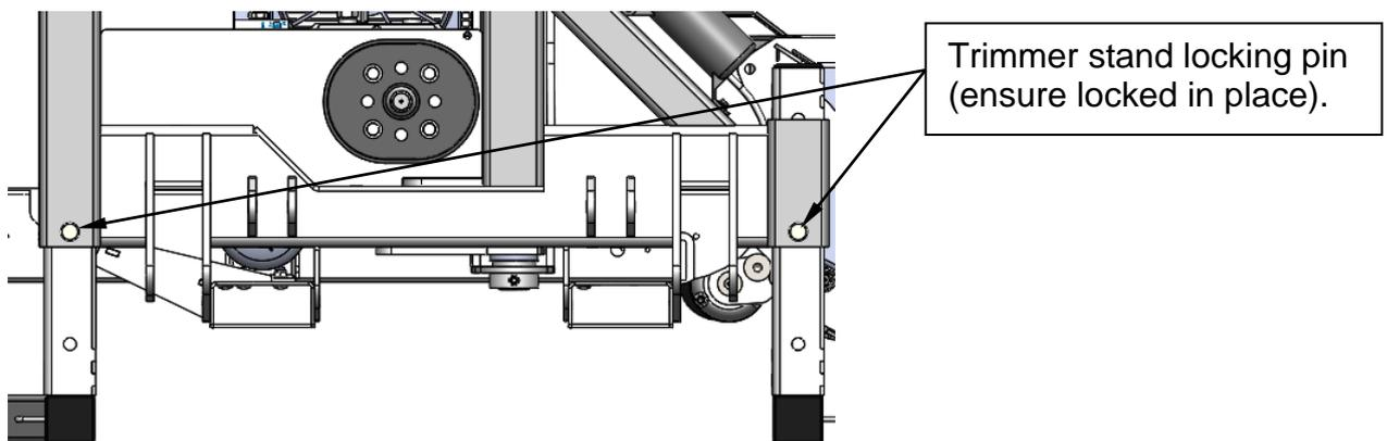
Insert the tines as far as they can go, to get the trimmer as close to the forklift as possible.
