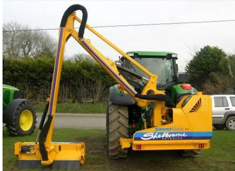
18. Correct adjustment has been reached when with the booms in the work position the machine remains parallel to the rear axle of the tractor. Take tyre squash into account when viewing this.
