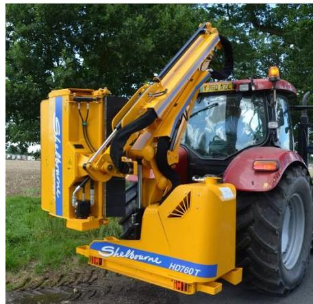
3. The reach cylinder can now be fully closed bringing the outer booms onto the bump stop on the inner boom.
