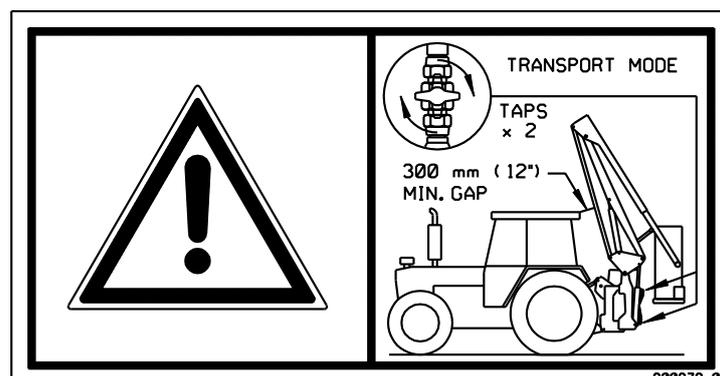
8. Even though the slew cylinder has PO check valves which locks the cylinder hydraulically a mechanical slew locking device should be put in place during all transportation on the public highways.
