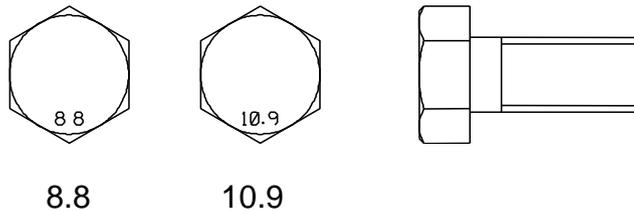
Note: Cutting head flail uses M16 higher grade fine threaded bolt which requires a torque setting of 270 Nm (200 lb/ft).
