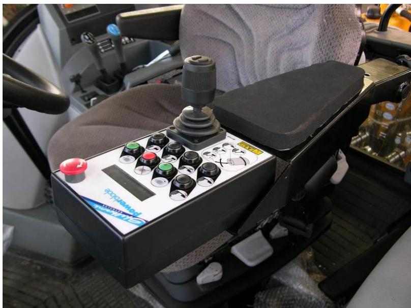
A 12 volt power supply is required for the electrical controls. These must be connected, via a suitable fuse. The power supply must not come from the cigarette lighter, three pin connector or trailer 7 pin socket; due to the electric controls having a high current draw. Low voltage will cause the system to function erratically. Therefore we recommend wiring directly to the tractor battery to guarantee system operation, with the supplied power lead, fuse and connectors.
