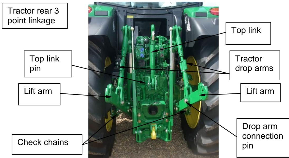
Ensure the tractor drop arms are of equal length ensuring they are kept at the minimum length required while still being able to hitch on the trimmer. Ensure the pin which connects the drop arm to the lift arm is positioned into the fixed rather than the float position (please refer to the tractor operators manual).
