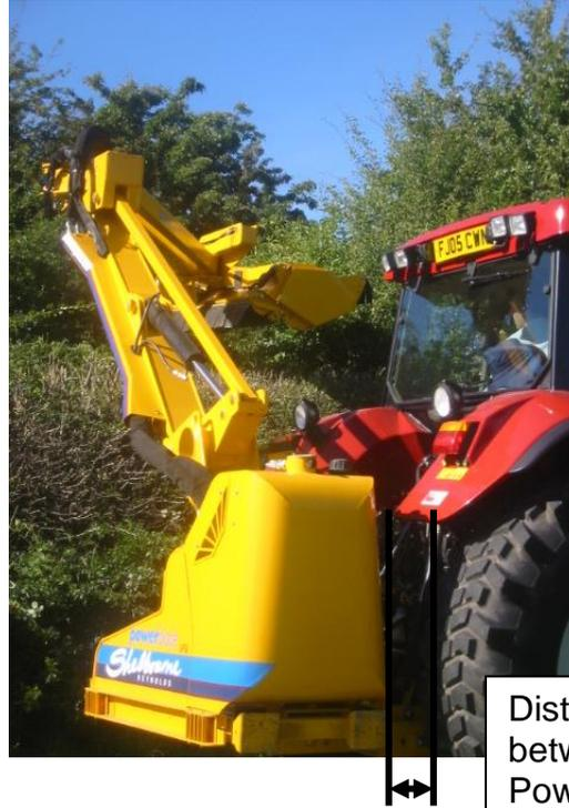
3. It's also possible to reduce the overall axle frame size further if required. This is done by cutting material off the hitch sub frame at the specified points.
