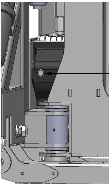
Sight glass for checking gearbox oil level
