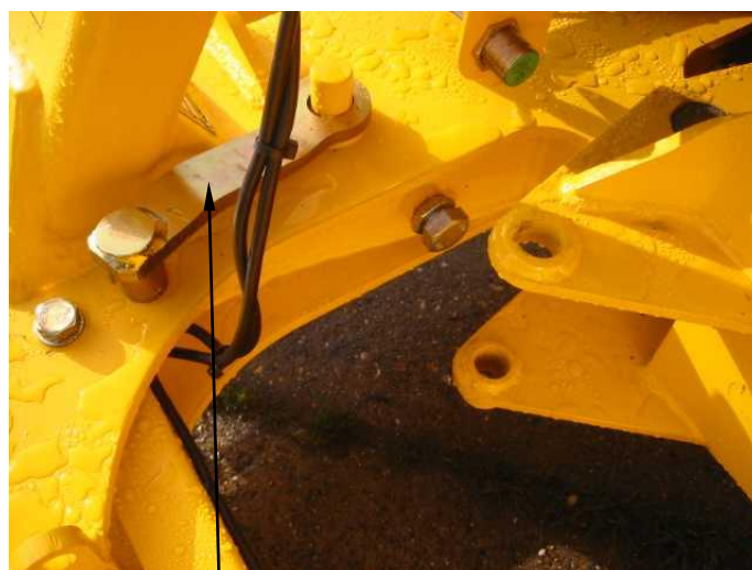
Slew locking device in its storage position during 'work'
