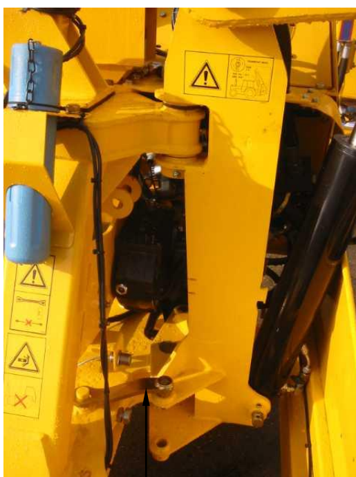
Slew locking device locking the slew cylinder during 'transport'
