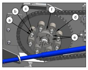
Replace the clutch plates with two new ones, ensuring the four pegs locate into the clutch hub (f) and drive disc when refitted. Fit the nuts and washers and adjust as described above.
