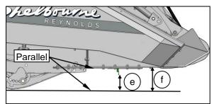
To reduce header loss, it may sometimes be necessary to pitch the header up further.
