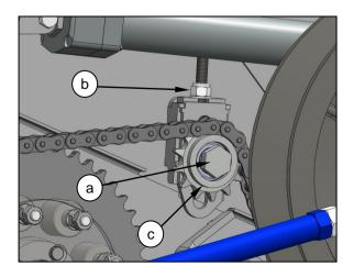
complete, tighten the idler spindle (a), check that the chain tension does not increase as the idler spindle is tightened.
