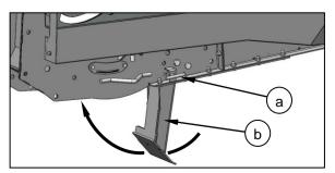
Ensure the header stands are raised on both ends of the machine.
