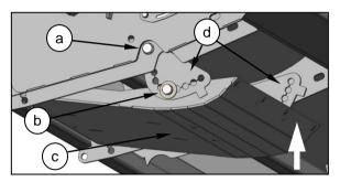
hole in the skid adjuster plate (d) and the skid. Repeat the process on the other side of the skid, ensuring that the same hole is used in both skid adjuster plates. Fully tighten all bolts (a & b) on both sides of the skid.
