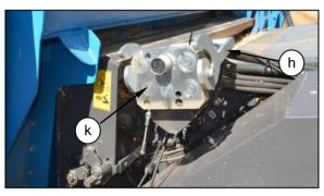
Connect the PTO shaft and monitor electrical connectors, then raise the header stands and release the adaptor plate pivot locking pin, as described in Section 5.1.6.
