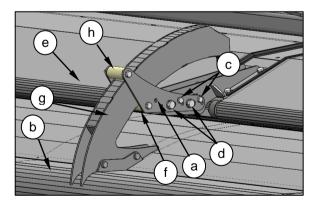
Remove the jack then raise and lower the crop deflector (b) to ensure that the bottom roller (f) supports the weight of the crop deflector and the top roller (h) does not contact the support (g) in all positions.
