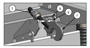
Remove the feeder house cylinder lock.
