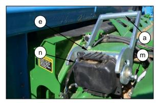
Remove the coupler (g) from the storage bracket (j) on the header and locate it onto the receptacle multicoupler on the feeder house. Pull the handle (a) to a horizontal position so that the dowels are engaged into the handle radial slots.
