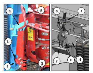
Recheck to ensure the hooks (b) are fully engaged on the pins (f). If they are not, adjust the handle (a) as described above.
