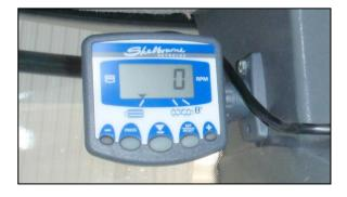
Either the long or short bracket can be attached to the head unit, whichever gives the most suitable orientation. Place the mounting pad underneath the mounting plate. Having established the orientation for the bracket, fix the mounting plate to the cab with the self-tapping screws provided.
