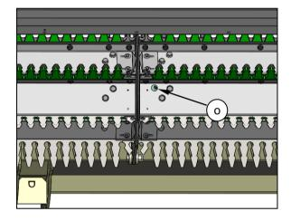
Refit the grease hole plug.
