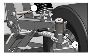
9. Gauge wheel axle hub bearing.
