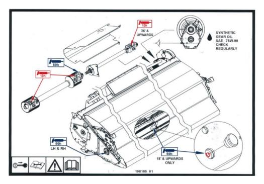
An additional decal is fitted to XCV machines that indicates the grease points on the variable speed drive pulleys and is located under the left hand drive guard.
