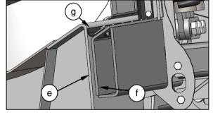
Check the pitch adjustment. The side plates of the header should be parallel to the ground or tilted back very slightly. This should equate to an approximate clearance (e) of 100mm (4") between the stripping rotor finger and the ground and (f) 150mm (6") between the bottom of the side plate and the ground.
