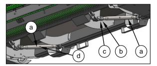
Slacken the two locking nuts (b & c), then wind the turn buckles (a) by placing a bar in the hole (d). The turn buckles should be adjusted until there is a gap of 10mm ( $\frac{3}{6}$ ") in the centre of the header between the main frame bottom beam (e) and the adaptor plate beam (f). Both turn buckles (a) should be adjusted to the same length.
