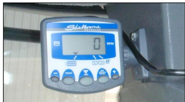
Either the long or short bracket can be attached to the head unit, whichever gives the most suitable orientation. Place the mounting pad underneath the mounting plate. Having established the orientation for the bracket, fix the mounting plate to the cab with the self-tapping screws provided.
