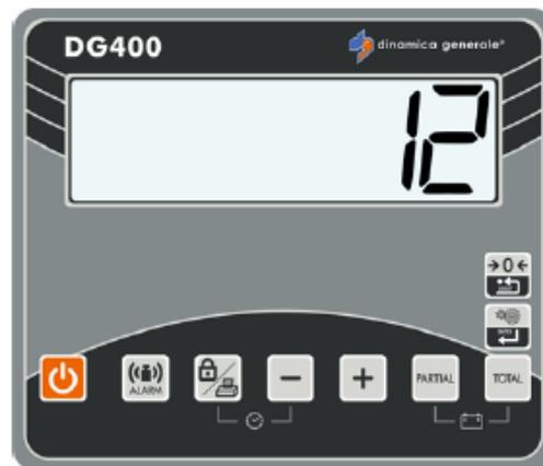
5. The word CALIB will appear on the display. Press the MINUS and PLUS keys to change the value of this parameter to either 5005 or 6674.
