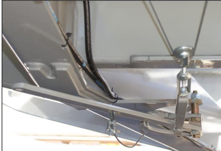
Twin auger models (16-25 m<sup>3</sup>) are supplied with a Rotary spindle type handbrake (See below). To apply the handbrake, simply rotate the crank handle clockwise to tighten the cable which in turn will activate the brake.
