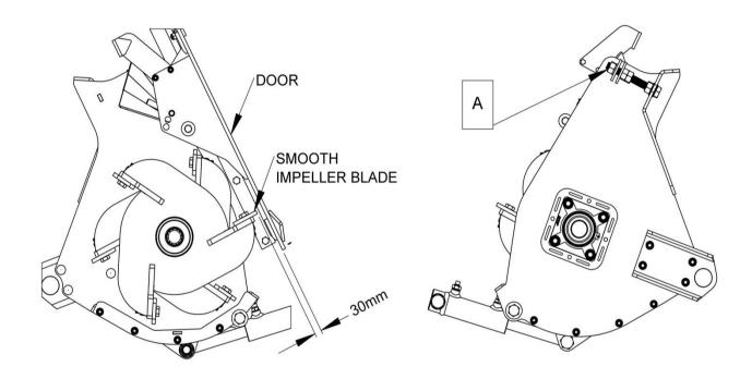
As the impeller blades wear, the whole impeller can be adjusted inwards. The distance can be easily adjusted by slackening or tightening the nuts (A) located on each side of the impeller assembly.
