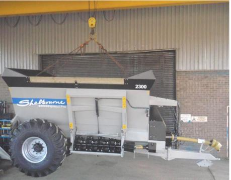
The centre of gravity of the machine is approximately 1.8m back from the inside of the front panel of the tub for 1800-2300 models & 2.3m from the inside of the front panel of the tub for 2400-3200 gallon models.
