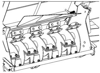
SPREADING DEFELCTOR SET FOR SLURRY
