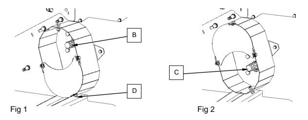
To gain access to the reverser shaft, simply slacken the locking screw (D), and rotate the front guard through 180 degrees, as shown in fig 2.
