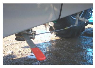
**Rotary spindle type** (See below – crank handle shown in resting position)
