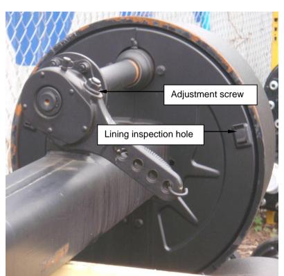
Check and test the brakes before intensive use and every 3 months.
