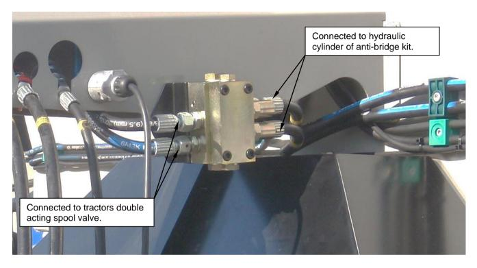
The manual hydraulic option simply connects 2 hydraulic couplings to the hydraulic cylinder of the anti-bridge kit, and is operated by a double acting spool valve on the tractor.
