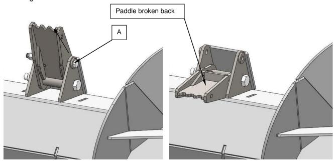
If the spread pattern becomes erratic or excessive noise is present then the machine should be stopped and investigated after the discharge of the current load, possible cause maybe the shearbolt(s) have broken on the auger paddles, or the obstruction is too large for the machine to dislodge.
