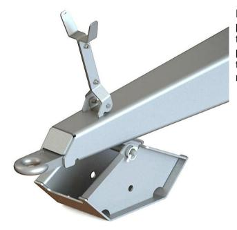
Parking foot shown in lower position. - This is required to gain the height required to position the pickup hitch directly under the towing eye while attaching the machine to the tractor.
