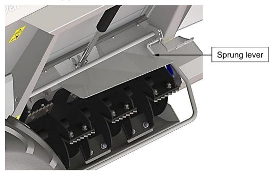
Above – Spreading deflector set for slurry.
