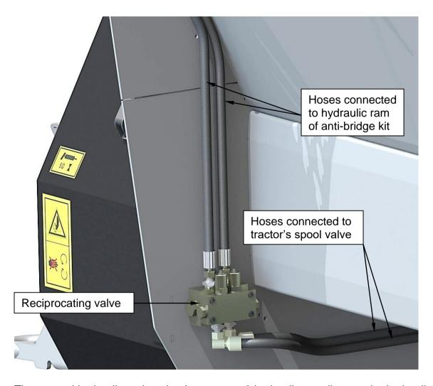
The manual hydraulic option simply connects 2 hydraulic couplings to the hydraulic cylinder of the anti-bridge kit, and is operated by the double acting spool valve of the tractor.
