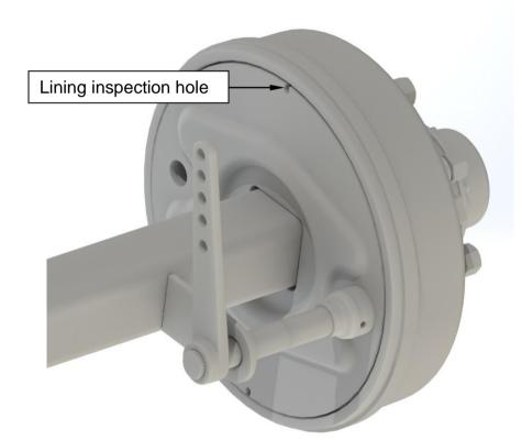
Check and test the brakes before intensive use and every 3 months.
