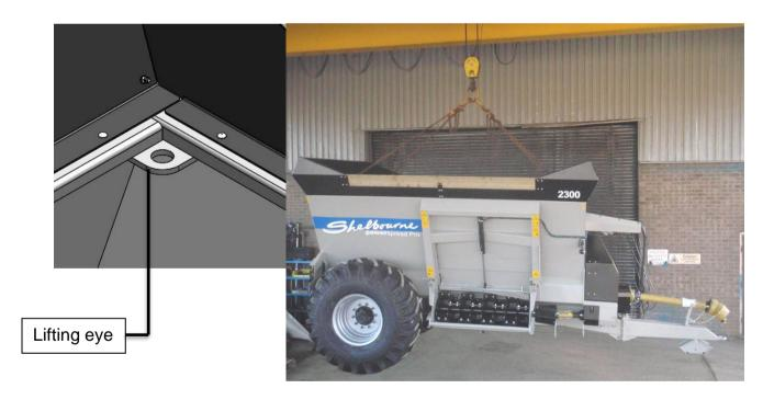
The centre of gravity of the machine is approximately 1.6m back from the inside of the front panel of the tub
