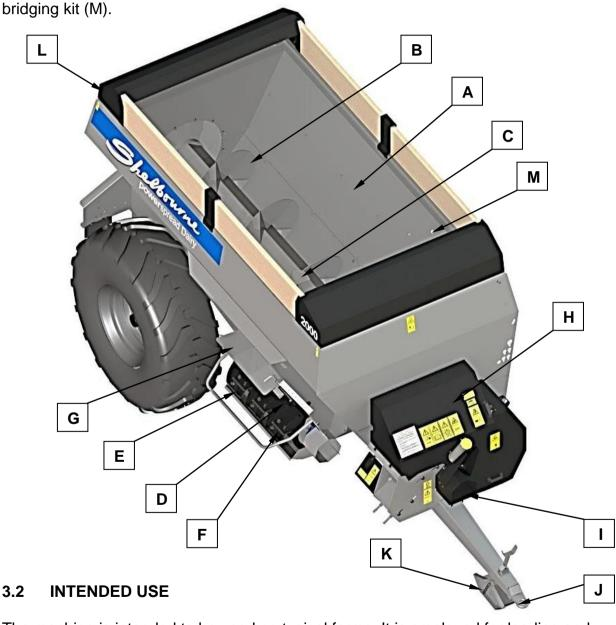
The machine is intended to be used on typical farms. It is employed for loading and spreading varying types of farmyard manure & slurry.
