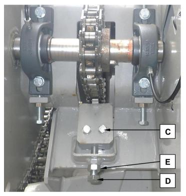
To tension the main 1 1/4" pitch auger drive chain, firstly remove the LH drive guard and then slacken the M10 tensioner fasteners (C), next adjust the M16 tensioner stud (D) to raise the tensioner block to the required position. Finally tighten the fasteners (C) and lock the assembly in place by tightening the lock nut (E).
