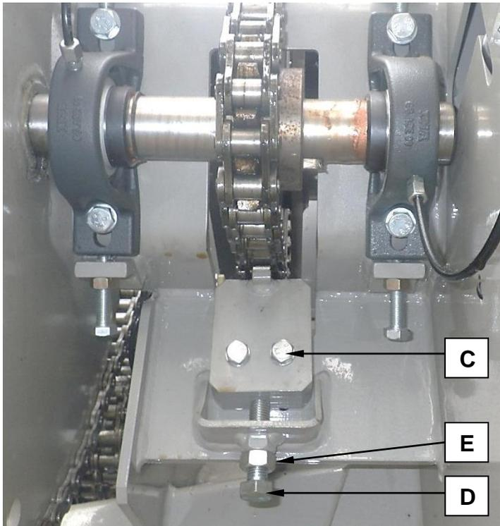
To tension the main 1 ¼" pitch auger drive chain, firstly remove the LH drive guard and then slacken the M10 tensioner fasteners (C), next adjust the M16 tensioner stud (D) to raise the tensioner block to the required position. Finally tighten the fasteners (C) and lock the assembly in place by tightening the lock nut (E).
