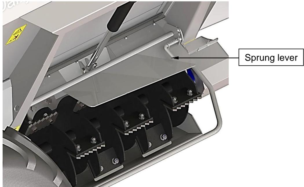
Above – Spreading deflector set for slurry.
