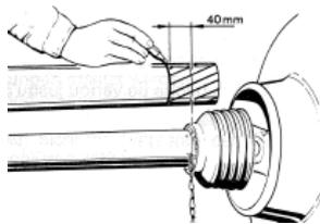
To adjust the lengths hold the half shafts next to each other in the shortest working position and mark them 40mm as shown.
