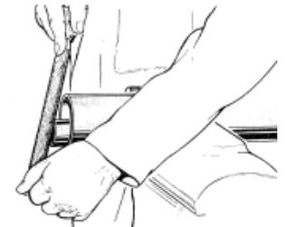
Remove all sharp edges and burrs, grease the sliding . Profile tubes
