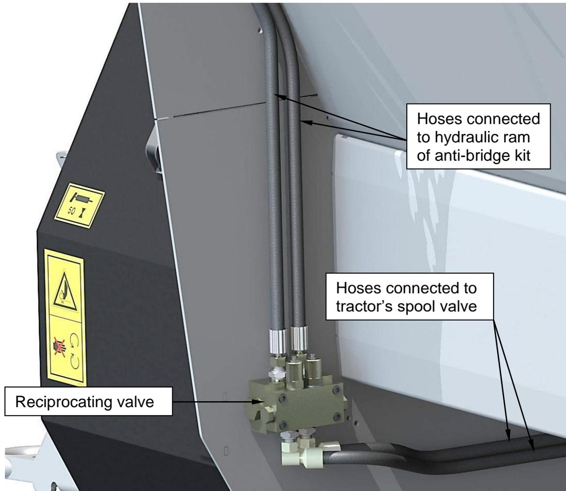
The manual hydraulic option simply connects 2 hydraulic couplings to the hydraulic cylinder of the anti-bridge kit, and is operated by the double acting spool valve of the tractor.
