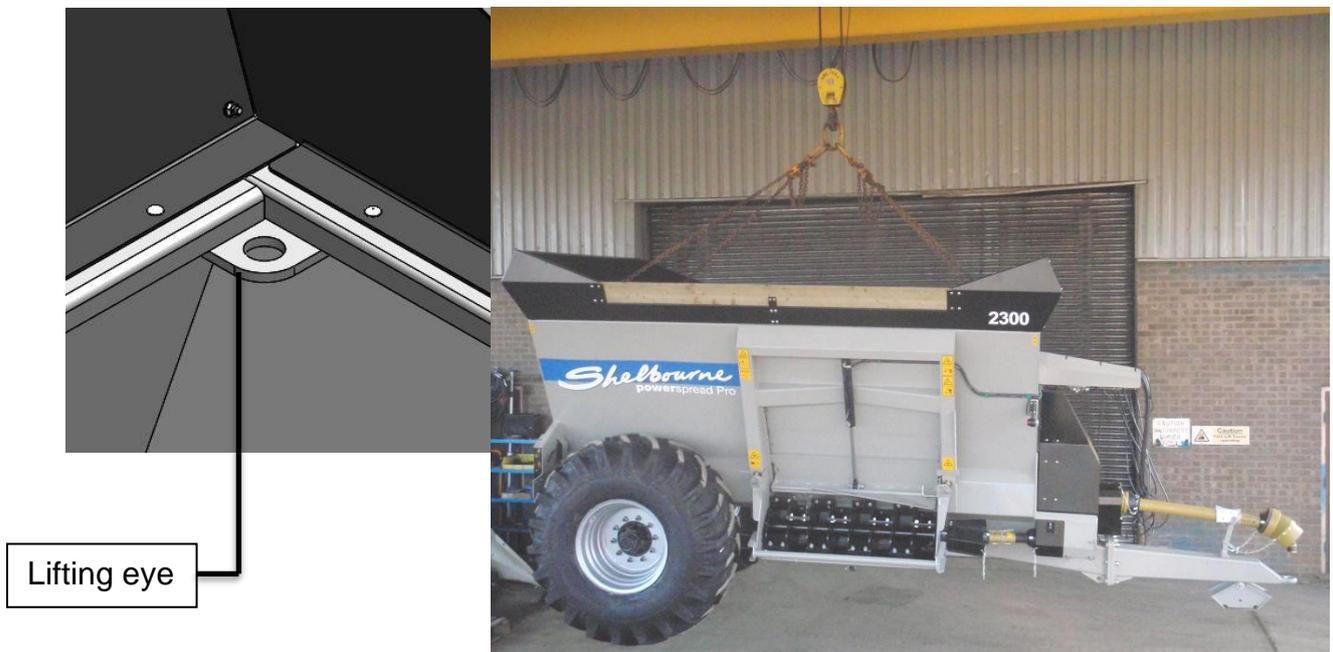
The centre of gravity of the machine is approximately 1.6m back from the inside of the front panel of the tub
