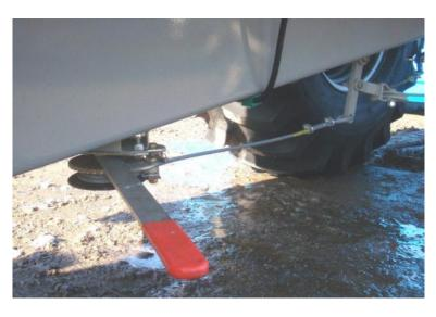
**Rotary spindle type** (See below – crank handle shown in resting position)
