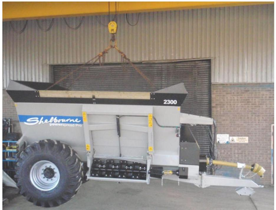
The centre of gravity of the machine is approximately 1.8m from the inside of the front panel of the tub for 1800-2300 models & 2.3m from the inside of the front panel of the tub for 2400-3200 gallon models.
