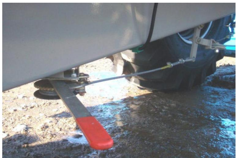
**Rotary spindle type** (See below – crank handle shown in resting position)
