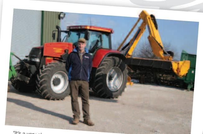
"It's a very clever system which uses a parallel linkage to ensure the head remains in the correct position as it is moved forwards or rearwards."
