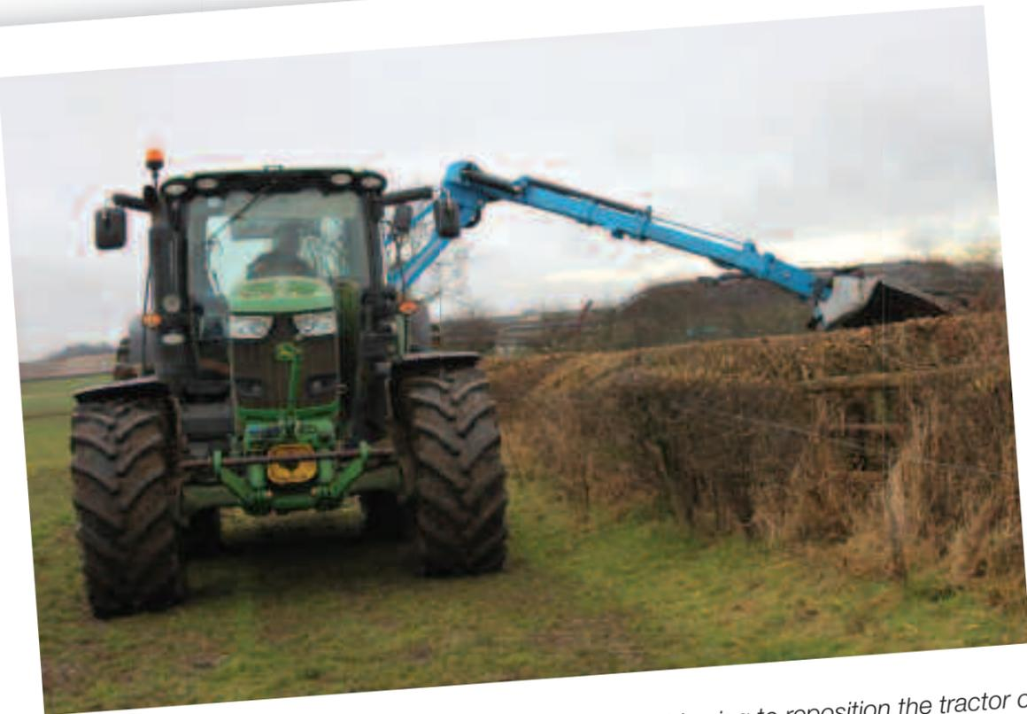
*"Telescopic capability is valued for the benefit it offers in not having to reposition the tractor or get too close to the work." Colin specified C-flails when ordering his Powerblade HD775 VFRT*
