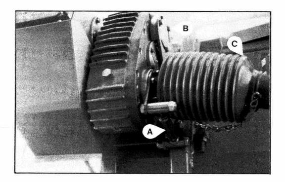
On the wider headers i.e. 5.4m and 6.0m, the gearbox assembly should be positioned so that the side PTO and rear PTO (C) are of approx. equal angles, when standard PTO joints are used. The angle of either shaft should not exceed 20 degrees. Recommended shaft positions are given in the combine model drive kit section, and is determined by the guard kit used.
