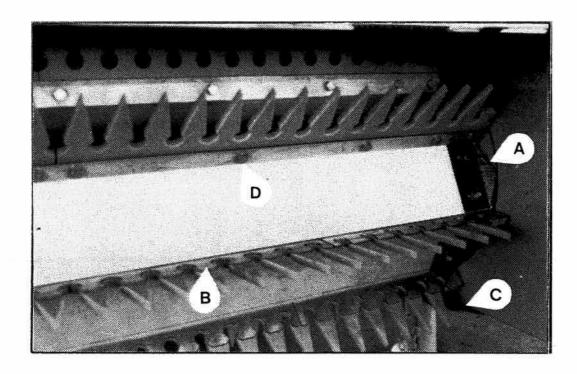
The centre of the rotor is fitted with a replaceable `vee' divider plate FIG 14(A), and anti-wrap finger (B). It is important to ensure that the vee strip overlaps the finger as shown.
