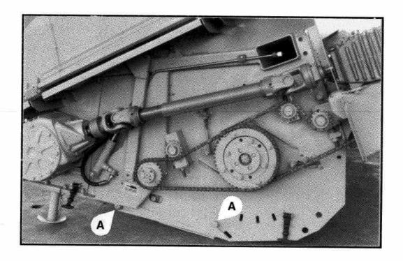
The skids under the *Shelbourne* Header are adjustable FIG 4, and can be moved by slackening off the 4 bolts (A) and sliding the skid in the slots.
