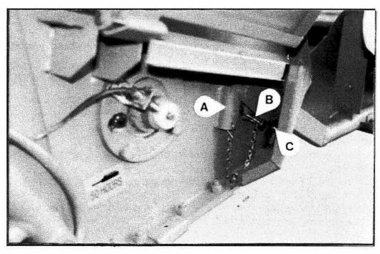
Torpedo type dividers are quick release. To fit the dividers, open the side guards, put the divider through the slot in the side frame, and hook into the catch at point (A) as shown in FIG 7. Place the clip (B) in the catch to prevent the divider falling out. The height of the divider can be adjusted by slackening the bolt and moving the adjusting bracket (C) to set the divider to the correct height.
