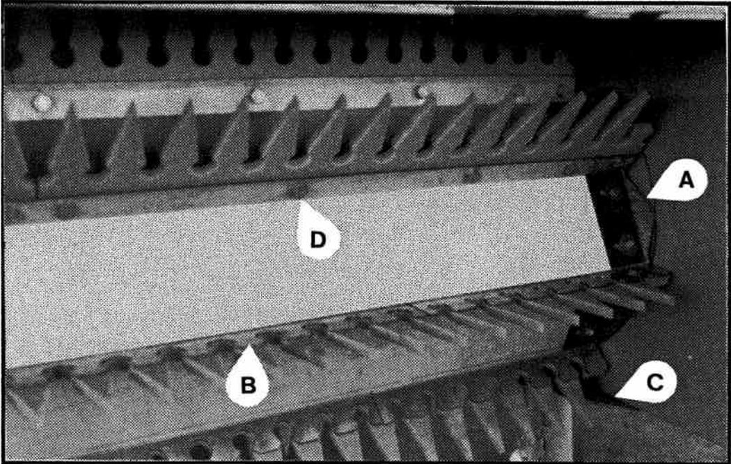
The centre of the rotor is fitted with a replaceable 'vee' divider plate FIG 12(A), and anti-wrap finger (B). It is important to ensure that the vee strip overlaps the finger as shown.
