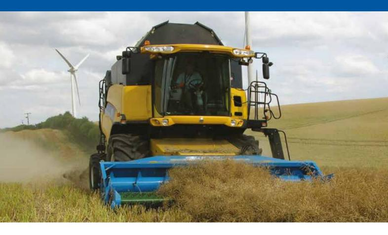
THE SHELBOURNE RANGE OF PICK UP HEADERS ARE DESIGNED FOR PICKING UP A WIDE RANGE OF SWATHS INCLUDING WHEAT, BARLEY, GRASS SEED, OILSEED RAPE AND BORAGE. THEY ARE DESIGNED TO FIT MOST MODERN COMBINE HARVESTERS USING A SIMPLE BOLT ON ADAPTOR PLATE.
