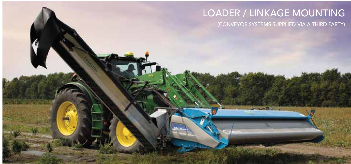
Hydraulic Drive - Requires An Oil Flow Of 90-100 Litres/Min
