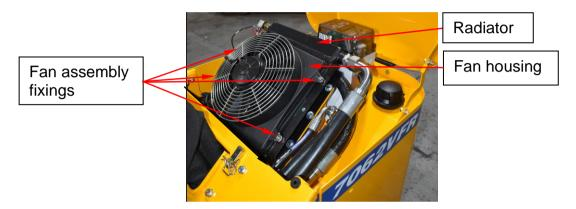
Blow the radiator out using high pressure air until clear line of sight can be seen through the radiator in all areas. Ensure to reach full extremities of the radiator. Then refit the fan assembly using the fixings removed.
