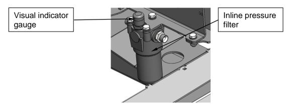
A return filter is fitted to the machine, in a housing, which is part of the top of the hydraulic tank. This must be changed after the first 50 hours and then subsequently after every 500 hours or 6 months. Note that if the filter is allowed to become clogged then the oil will bypass the filter (to avoid the danger of the filter bursting) and could allow contaminants into the tank and hence into the system components.
