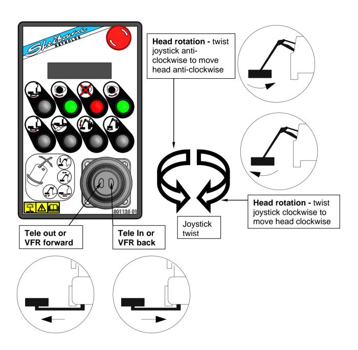
In addition to the joystick, there are 8 additional buttons; each represented by a diagram. Their meanings are detailed below.
