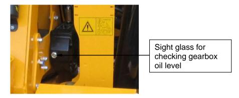
Check gearbox oil level regularly, a sight glass is fitted on the rear face to facilitate this on GEA-0187 – Gearbox (large).
