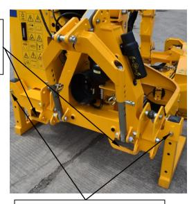
Trimmer stands locking pin (ensure locked in place)
