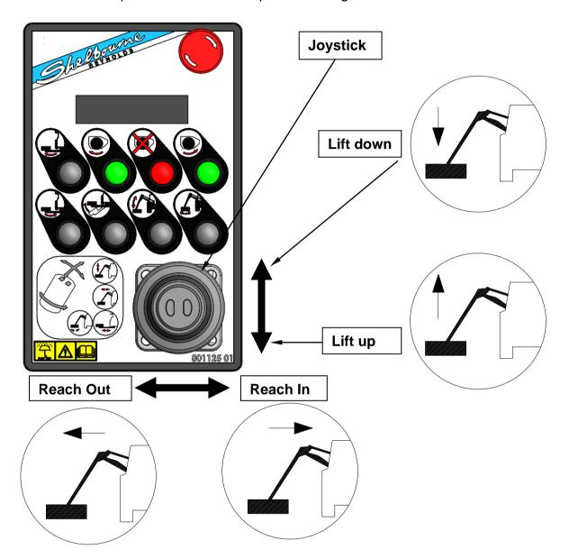
**Head rotation:** Twist the joystick clockwise and anti-clockwise to rotate the head. This service action is also proportional. It's possible for the head rotation to be changed to operate the opposite way around by toggling a setting within the hedge / verge trimmer control box (see section 6.3).
