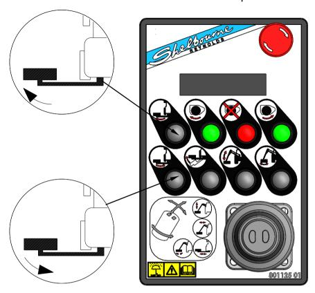
**Slew Backward**: Rotates the arms into the transport position behind the tractor.
