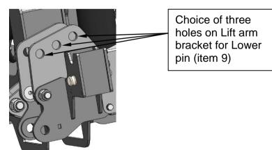
3. For lift arms of the quick release ball end type fit the tractor balls, Lower pin (item 9), Spacers (item 16) and Lynch pins (item 6) to both sides of trimmer frame on the Lift arm bracket.
