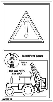
8. Even though the slew cylinder has PO check valves which locks the cylinder hydraulically a mechanical slew locking device should put in place during all transportation on the public highways.
