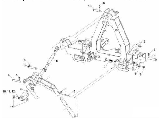
1. Identify if the tractor has lift arms with fixed ball ends or has a quick release ball end style. For Lift arms with the fixed ball ends prepare the pin (item 9), lynch pin (item 6) and spacers (item 16).
