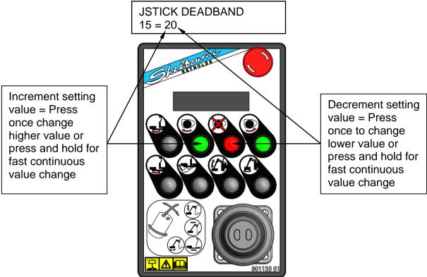
Once the setting value has been changed the control display will automatically save and when no buttons are pressed for a few seconds the controls will exit the setup mode and the screen will default back to the Standard screen display.
