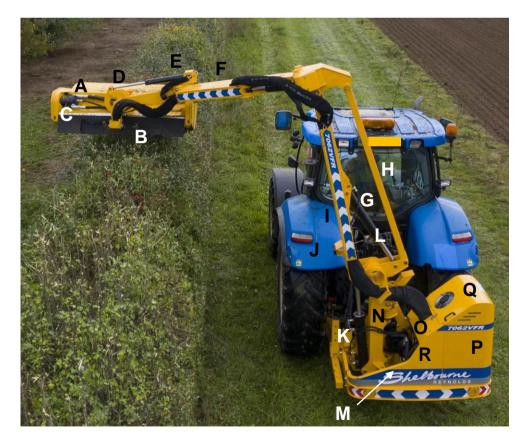
A PTO drive operating at 540rpm (or 800 rpm option), with a 1 & 3/8" SAE 6 spline shaft and rotating in a clockwise direction is required.
