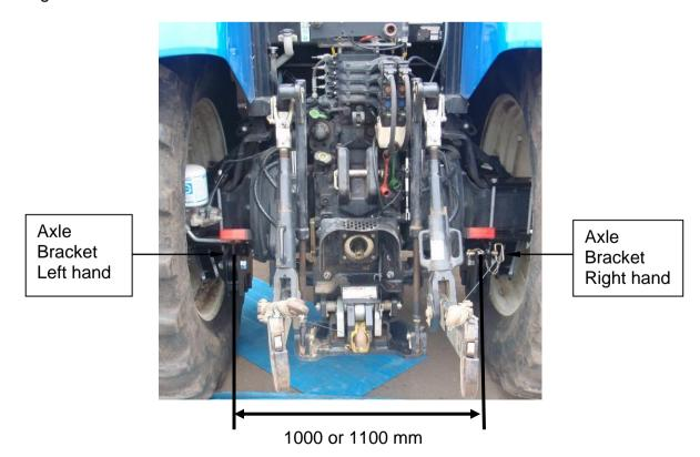
Shelbourne Reynolds axle brackets supplied will be accompanied by the axle bracket parts list and fitting instructions which will include specific instructions on how to fit the axle brackets to specific tractors.
