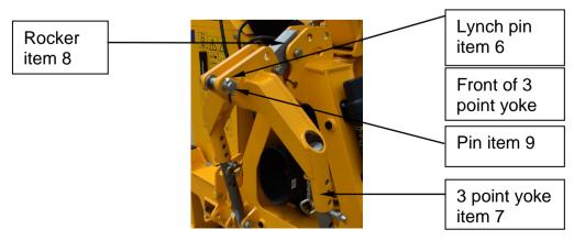
Note: A 65mm longer rocker is also available to order from SRE parts part number: 806071 01 if the tractor is not compatible with the standard fitment.
