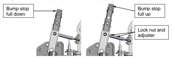
5. Taking care that the booms do not foul the cab top, extend the lift cylinder to bring the rocker to rest gently onto the bump stop. Disengage the PTO.
