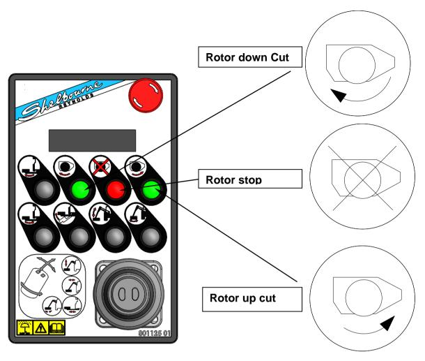
Controls display screen when starting the cutting head rotor:
