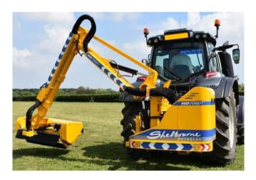
2. Use the slew cylinder to rotate the arms fully back, and then position the cutting head with the flail facing the operator and the top of the cutting head backwards towards the following traffic.
