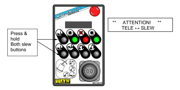
**Rotor down cut**: Engages the cutting head rotor in the down cut direction. Hold down the button for 3 seconds to engage. An LED light (in the button) shows the status of the down cut. A solid light indicates that it is engaged. A flashing light indicates that it is slowing down or that the oil is over temperature. The rotor cannot be started when either the up cut or down cut lights are flashing.
