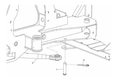
1 Connect the larger diameter end of the adjustable link into the tractor drawbar clevis using the tractor drawbar pin.
