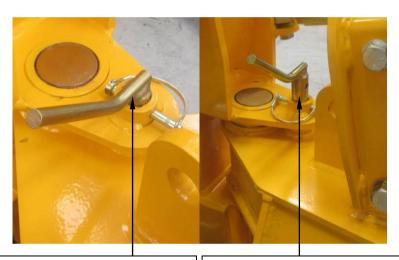
Slew locking device locking the slew cylinder during 'transport'
