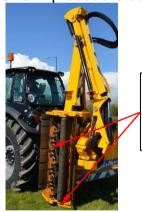
Cutting head in contact with the ground allowing access to the flail area
