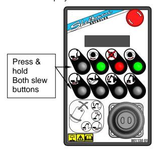
\*\* ATTENTION! \*\* SLEW ↔ TELE To return Slew control to Slew buttons and Telescopic control to Telescopic buttons.
