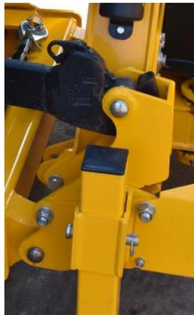
6. Release the axle bracket latches, allowing the sub frame to be lowered clear of the tractor by extending the adjustable top link.
