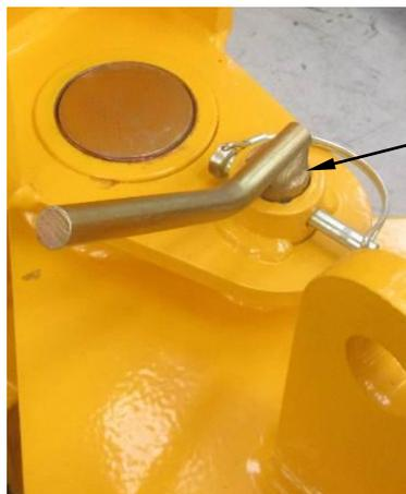
Slew locking device locking the slew cylinder during 'transport'
