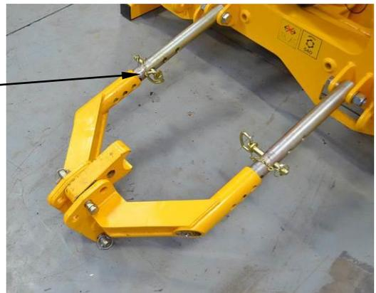
5. Connect item 8 into the middle hole of the three holes in item 7 using pins item 14 & 6.
