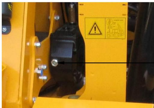
Sight glass for checking gearbox oil level
