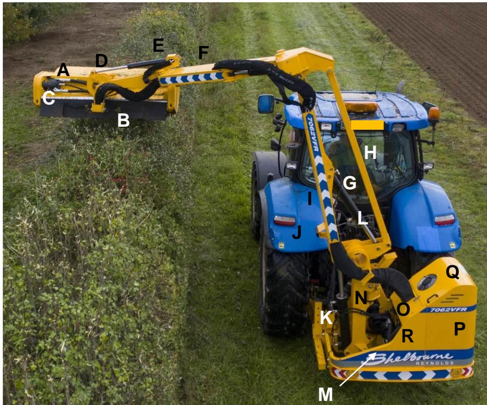
A PTO drive operating at 540rpm (or 800 rpm option), with a 1 & 3/8" SAE 6 spline shaft and rotating in a clockwise direction is required.
