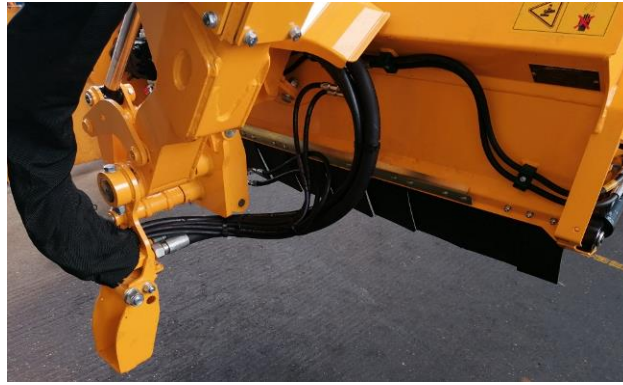
Narrow lane bracket in its fully extended position rotated 53 degrees
