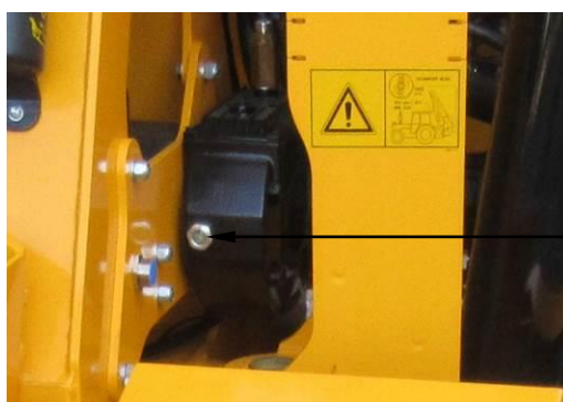
Sight glass for checking gearbox oil level
