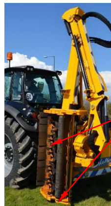
Cutting head in contact with the ground allowing access to the flail area
