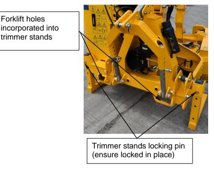
Ensure that the tines go through both slots in the front and back plates.
