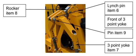
Note: A 65mm longer rocker is also available to order from SRE parts part number: 806071 01 if the tractor is not compatible with the standard fitment.
