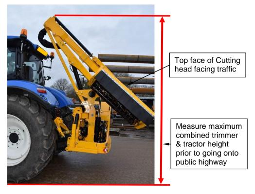
It's recommended to disconnect all electrical, hydraulic connections and the PTO driveshaft from the hedge / verge trimmer so that it cannot be inadvertently operated during road transport.
