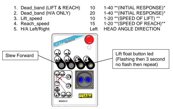
Before adjusting the setting value to another firstly cover the arm float button LED.
