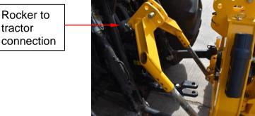
9. Fit the top link (item 13) between the trimmer main frame and the 3 point yoke using the pins and lynch pins provided. Ideally maintain a straight line through the pivot points once in the raised position.
