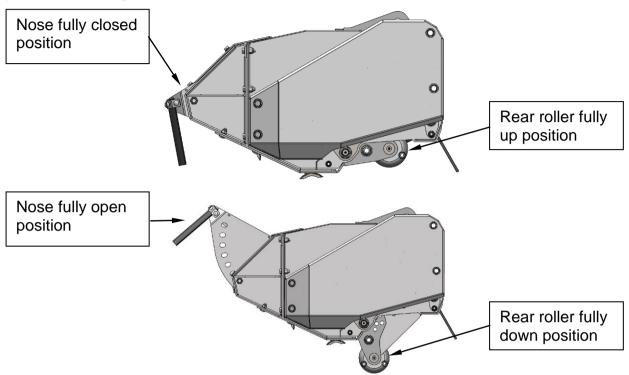
Never remove the nose completely. Always ensure the front and rear curtains are in good condition.
