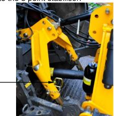
Serious damage may occur if the tractor 3 point linkage is raised without removing 3 point linkage locking pins (item 5).
