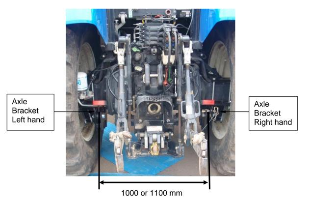
Shelbourne Reynolds axle brackets supplied will be accompanied by the axle bracket parts list and fitting instructions which will include specific instructions on how to fit the axle brackets to specific tractors.
