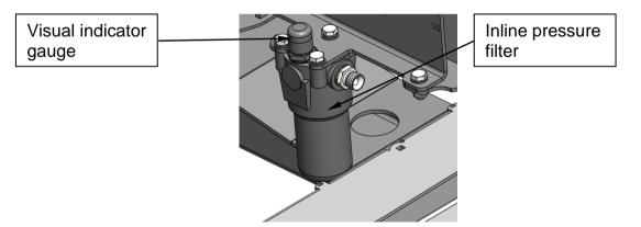
A return filter is fitted to the machine, in a housing, which is part of the top of the hydraulic tank. This must be changed after the first 50 hours and then subsequently after every 500 hours or 6 months. Note that if the filter is allowed to become clogged then the oil will bypass the filter (to avoid the danger of the filter bursting) and could allow contaminants into the tank and hence into the system components.
