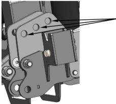
Choice of three holes on Lift arm bracket for Lower pin (item 9)
