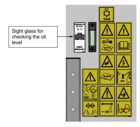
If a biodegradable oil is to be use, please contact Shelbourne Reynolds Ltd with the oil specification to check suitability.
