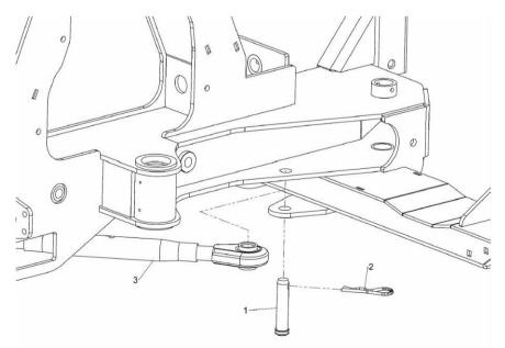
1 Fit item 3 into the clevis incorporated within the trimmer main frame assembly using item 1 and 2. Ensure the smaller diameter end of the adjustable link is fitted into main frame.
