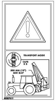
8. Even though the slew cylinder has PO check valves which locks the cylinder hydraulically a mechanical slew locking device should put in place during all transportation on the public highways.
