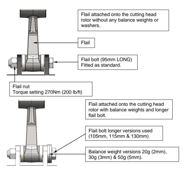
Replace spacers, bolts and nuts exactly when replacing flails. The flails themselves should wear evenly and be replaced as a set. Should one flail be lost then the flail at 180°, one place along should be renewed at the same time to preserve the balance.
