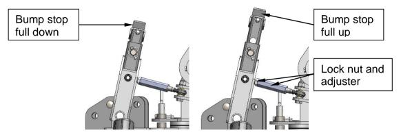
5. Taking care that the booms do not foul the cab top, extend the lift cylinder to bring the rocker to rest gently onto the bump stop. Disengage the PTO.
