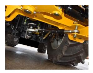
2 Once connected decrease the adjustable link length as much as possible. In some cases, it's also required to place the head horizontal to the ground, close to the tractor tyre in the work position power the booms into the ground. This may then allow further adjustment if required.
