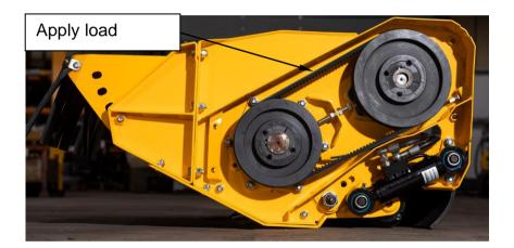
To adjust, slacken the nuts at the motor fixing bolts and the adjuster locknut, then turn the adjuster nut in the required direction. Then tighten lock nut and nuts for the motor fixing bolts. Finally replace the drive cover.
