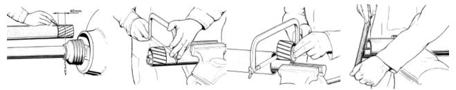
The length adjustment is to be carried out as follows: To adjust the lengths hold the half shafts next to each other in the shortest working position and mark them 40mm as shown.
