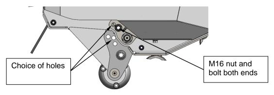
The nose is adjustable into one of seven positions using a series of holes within the nose assembly. To reduce the danger of debris being thrown out of the front of the head the nose **MUST** be set in its lowest position for verge work, and as low as is practical for hedge cutting.
