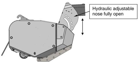
The hydraulic nose includes a mechanical stop bolt which must remain fitted at all times. This mechanical stop helps to protected the cylinders, nose, side pods and nose hinge from being forced during operation.
