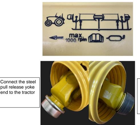
Connect the plastic pull release type yoke end to the hedge / verge trimmer
