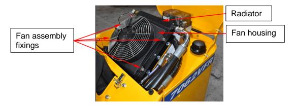
Blow the radiator out using high pressure air until clear line of sight can be seen through the radiator in all areas. Ensure to reach full extremities of the radiator. Then refit the fan assembly using the fixings removed.
