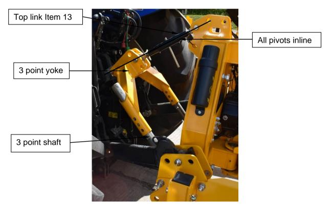
10. Ensure the tractor check chains are free to float at this stage.
