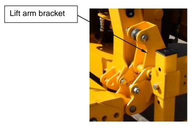
3. For lift arms of the quick release ball end type fit the tractor balls, Lower pin (item 15), Spacers (item 16) and Lynch pins (item 10) to both sides of trimmer frame on the locked Lift arm bracket.
