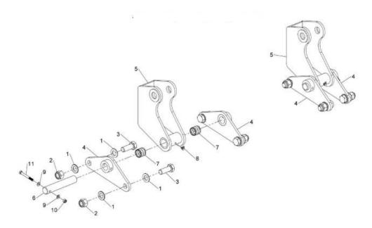
2. The axle frame stabiliser which connects to the tractor can be set at two different widths. Both Pin arms item 2 and 3 can be swapped over to give either 1000 or 1100mm depending on which width the axle brackets attached onto the tractor axle have been set.
