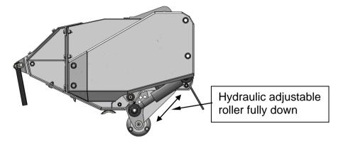
Ensure that both hoses are correctly connected to the tractor spool before adjusting the roller. Damaging high oil pressures can be generated if actuated with one hose disconnected.
