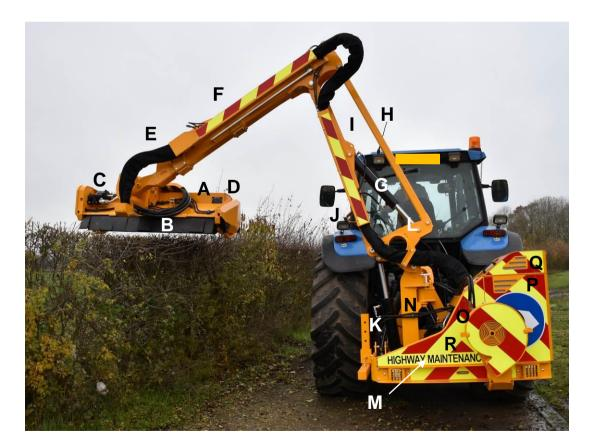
A PTO drive operating at 540rpm, with a 1 & 3/8" SAE 6 spline shaft and rotating in a clockwise direction is required.
