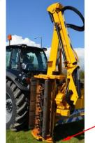
Cutting head vertically upright but in contact with the ground
