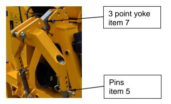
15. Remove the top link pin between the tractor and 3-point linkage rocker. Then swing the 3 point assembly away from the tractor towards the trimmer main frame. Re-position the rocker (item 8) from the front of the 3 point yoke to the rear enabling it to connect between the trimmer main frame and the 3 point yoke.
