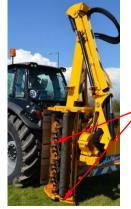
Cutting head in contact with the ground allowing access to the flail area Ensure that there is nothing wrapped around the rotor or roller.
