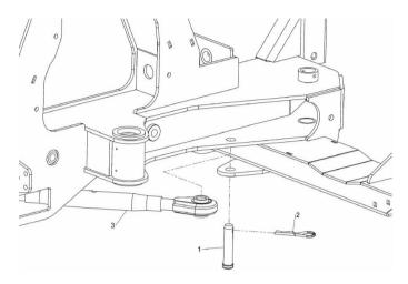
1 Connect the larger diameter end of the adjustable link into the tractor drawbar clevis using the tractor drawbar pin.
