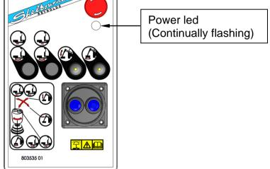
Before adjusting from one function to another (dead band lift & reach, dead band H/A, lift speed, reach speed and H/A) firstly cover the head float button LED. Then pressing the **"Slew forward button**" (left of the four buttons) will enable you to move from one function to another. The **"Lift float button**" led will then simultaneously change and flash to indicate which function you're in.
