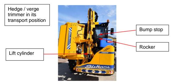
• Use the lift, reach and head angling cylinders to bring the head to a position near to the tractor, parallel to, and close to the ground.
