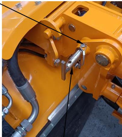
Locking pin (Shown in the unlocked position)
