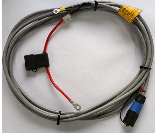
Route and secure the power lead into the tractor cab, terminating close to the controls armrest. Using the large rectangular shaped multi pin connector, connect the machine end wiring loom to the joystick control box. Then also connect the power supply for the controls to the joystick control box, using the two 4 pin screw connectors. Finally, connect the power supply for the oil cooler to the oil cooler control box loom, using two 4 pin screw connectors.
