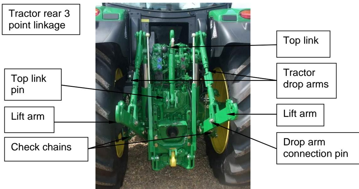
Ensure the tractor drop arms are of equal length ensuring they are kept at the minimum length required while still being able to hitch on the trimmer. Ensure the pin which connects the drop arm to the lift arm is positioned into the fixed rather than the float position (please refer to the tractor operator's manual).
