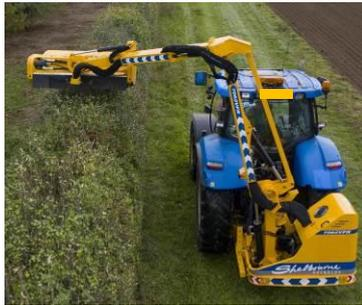
17. Point 15 and 16 should be repeated once the trimmer is fully operational. In some cases, it's also required to place the head horizontal to the ground, close to the tractor tyre in the work position power the booms into the ground. This may then allow further adjustment to the tractor check chains and drop arms if required.
