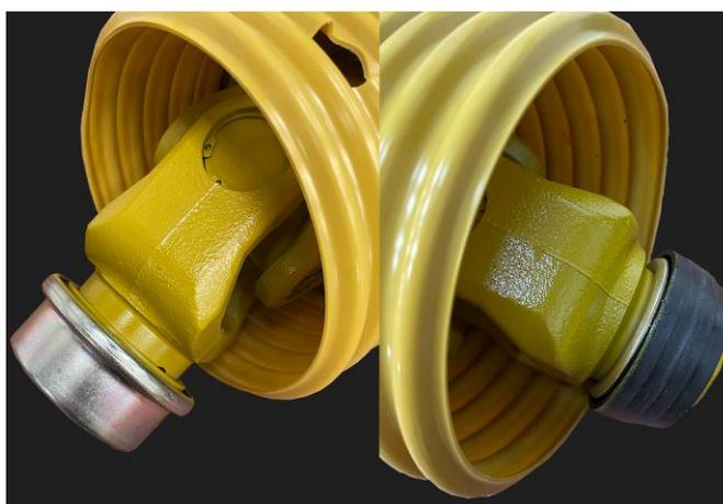
Connect the plastic pull release type yoke end to the hedge / verge trimmer
