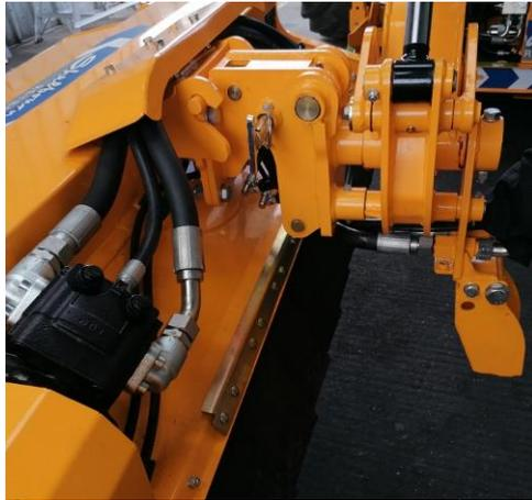
Narrow lane bracket in its fully closed position
