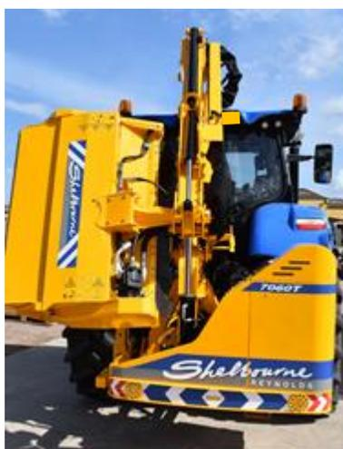
3. The reach cylinder can now be fully closed bringing the outer booms onto the bump stop on the inner boom.
