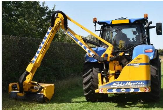
18. Correct adjustment has been reached when with the booms in the work position the machine remains parallel to the rear axle of the tractor. Take tyre squash into account when viewing this.
