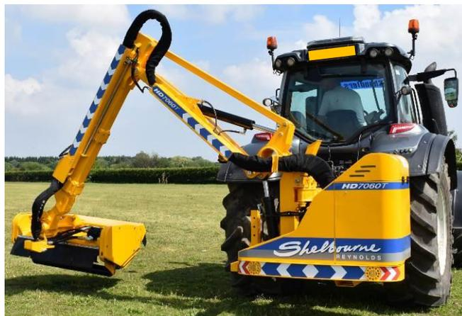
2. Use the slew cylinder to rotate the arms fully back, and then position the cutting head with the flail facing the operator and the top of the cutting head backwards towards the following traffic.
