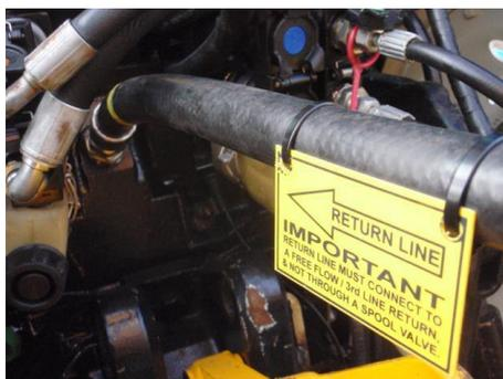
To ensure the fan is running smooth turn the tractor spools flow down to between 30 – 40 l/min or if the fan blower is hunting turn the tractor spool flow down until it runs smooth. Excessive tractor flow may cause heat build-up for both the tractor and the debris blower.
