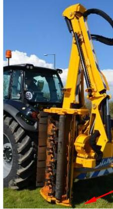
Cutting head vertically upright but in contact with the ground
