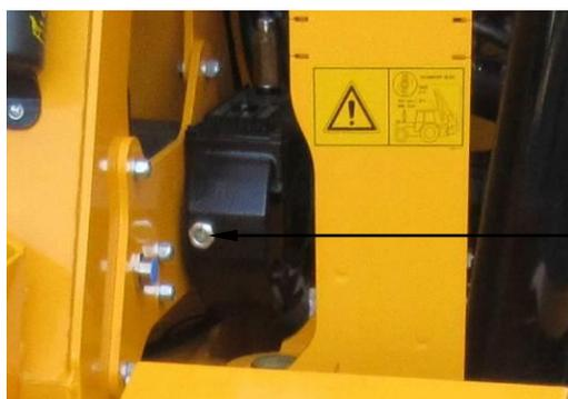
Sight glass for checking gearbox oil level
