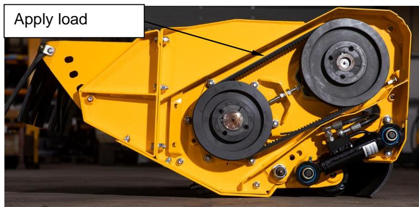
To adjust, slacken the nuts at the motor fixing bolts and the adjuster locknut, then turn the adjuster nut in the required direction. Then tighten lock nut and nuts for the motor fixing bolts. Finally replace the drive cover.
