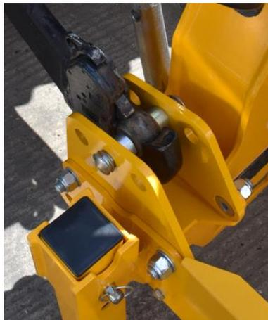
5. Remove the tractor top link from the tractor but ensure to keep the top link pin and lynch pin close to hand.
