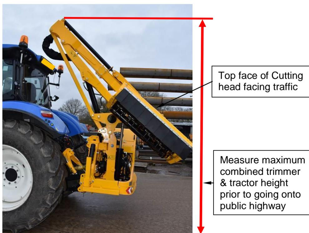
It's recommended to disconnect all electrical, hydraulic connections and the PTO driveshaft from the hedge / verge trimmer so that it cannot be inadvertently operated during road transport.
