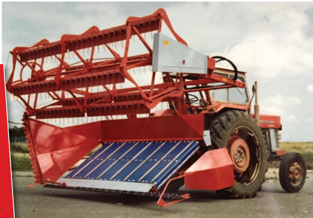
Alto-Chalmers All-Crop 42 The 2-speed power drive Reel has quickly adjustable supports
