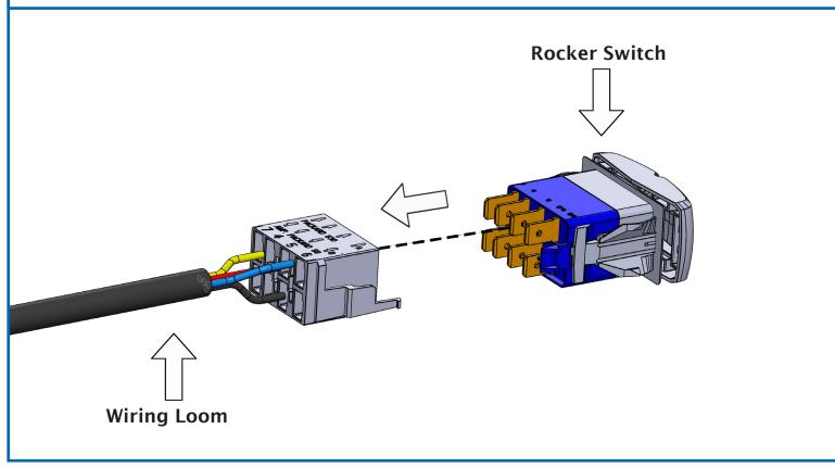
2. Snap off the tab on the quick release block if present, then fix the plug module to the
