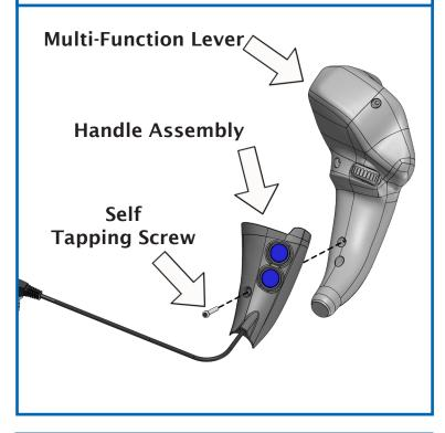
Tighten until there is no movement in the handle assembly but be careful not to overtighten.
