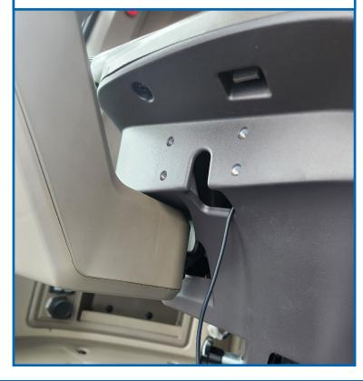
6. Push the multi-function lever into the plug module making sure to use the correct jack port.
