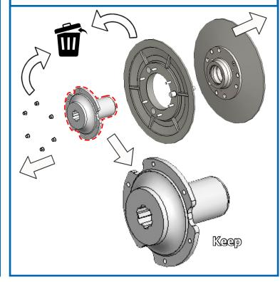
29. Remove the old sprocket and install the new one if provided with your kit, (KIT-19089, KIT-19091 and KIT-19094 only).
