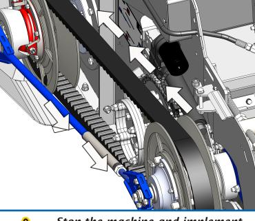
Stop the machine and implement safe stop. DO NOT put hands between pulley sheaves.
