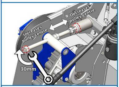
The belt should be tensioned so that the spring is compressed to the same length as the spacer tube. It should still be possible to rotate the spacer tube.
