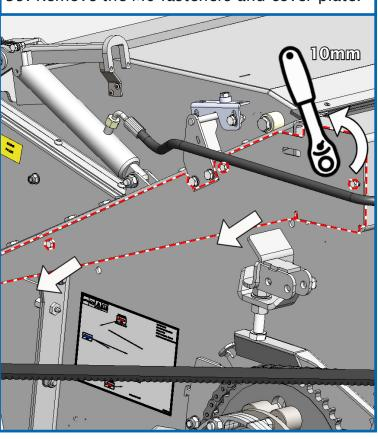
40. Tie up the actuator cable and feed into the top beam then reattach the cover plate.
