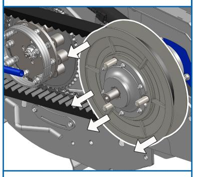
Take care when removing the pulleys from the shafts, as they weigh 40KG (88lbs).
