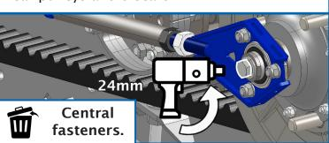
8. Loosen tie rod bearing fasteners on both front and rear pulleys, and remove tie rod.
