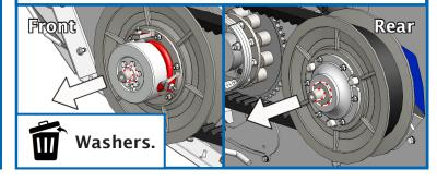
9. Loosen the gearbox adjuster locknuts.
