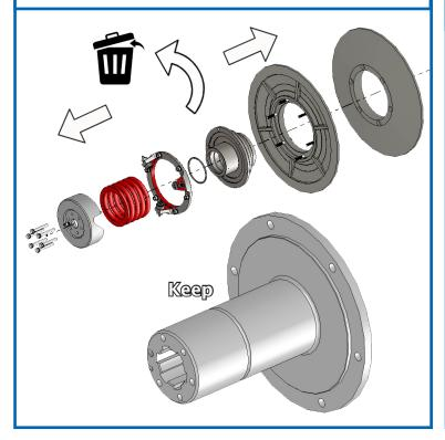
20. Separate the pulley and centre hub.
