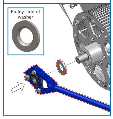
26. Fasten with the **NEW** M16 set screw and tighten to 225Nm (166lb-ft). The pulley should be held tight on the shaft, no end float of pulley on the shaft.
