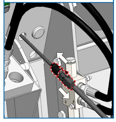
42. Feed the cable back into the header and cable tie in a secure position. No longer required for header attachment to combine.
