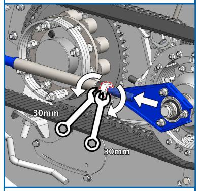
Tighten by hand until taught, then turn an extra 1/6 of a turn and tighten the lock nut.
