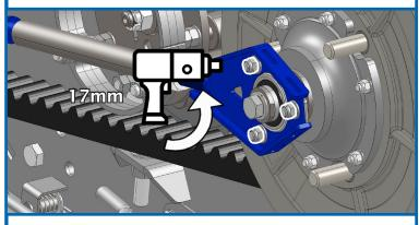
Remove central fasteners on the front and rear pulleys and discard.
