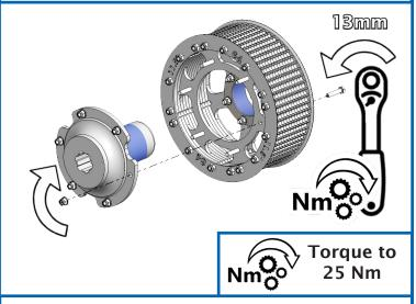
Refer to the speed chart to determine what pulley size to install on the front hub, change the sprocket if needed.
