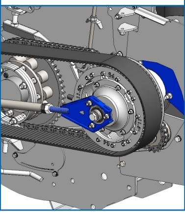
36. Adjust the gearbox pivot to tension the belt. The tension of the HTD drive belt is indicated by the spacer tube which fits over the spring on the gearbox adjuster.
