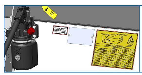
The decals should be placed near the identification plate of the machine.
