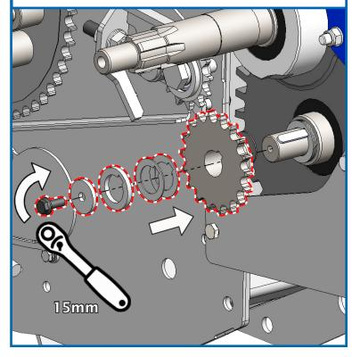
30. Refit the chain and tension accordingly. The chain length may need to be adjusted to suit the new sprocket size.
