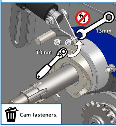
13. Remove the electric actuator with cam brackets.
