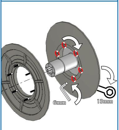
22. Check wear on pulley hub. Ensure fitment of laminate pulley onto hub (shaded region), has little to no side play <0.8mm (1/32").
