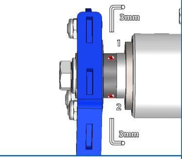
If the front shaft has a groove beneath the tie rod bearing you need to align one grub screw so it tightens into it.
