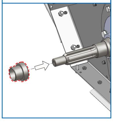
24. Grease the shaft using black grease and then push on the new front pulley.
