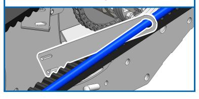
6. Loosen tie rod bearing grub screws (x2) on both front and rear pulleys.
