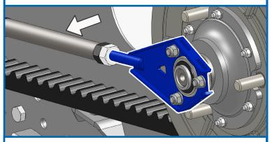
Remove washers from front and rear pulleys then discard.
