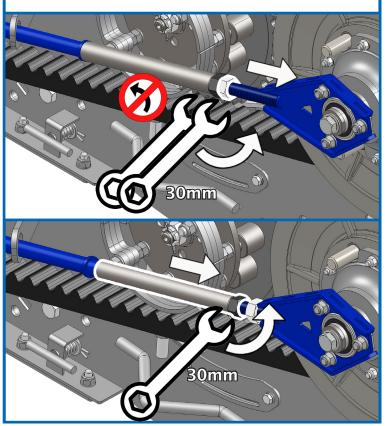
5. Remove the tie rod support fasteners.
