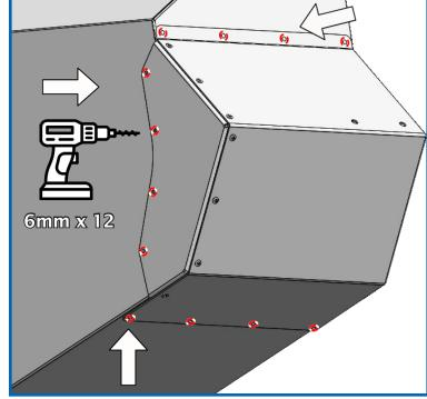
9. Fix the assembled extension guard to the main guard using 6mm pop rivets.
