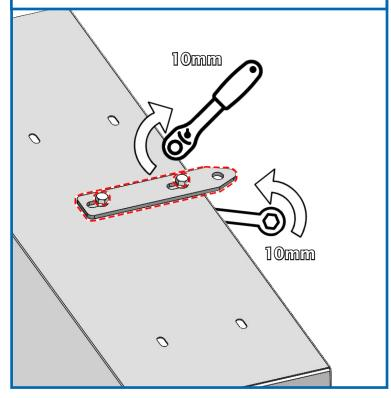
13. Reattach the main guard to the machine using the two locating plates and pins.
