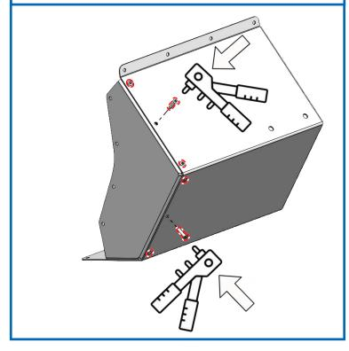
8. Mark out the holes needed to secure assembled extension guard to the main guard. Drill the marked holes using a 6mm drill bit.
