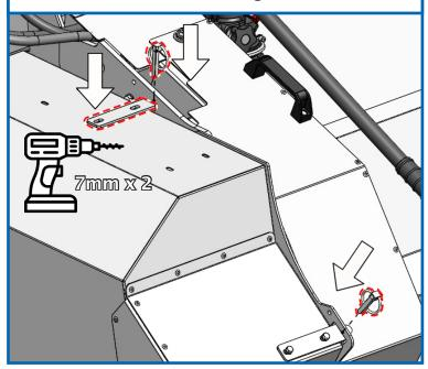
12. Fix the second locating plate (item 1), to the main guard using two M6 x 20mm bolts, washers and nyloc nuts.
