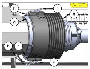
Reconnect the left hand end PTO guard retaining chain (b) to the header
