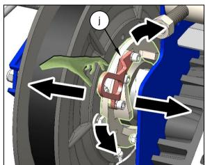
Refit the cam retaining bar (i) ensuring it slides into slot in static cam arm (k). Refit both R-clips (g) to secure the cam retaining bar (i)
