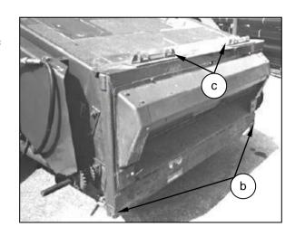
Raise the feeder house to lift the header, ensuring that the pivot blocks (c) are properly seated in the pockets (e) in the adaptor plate top beam, then fully raise the header.
