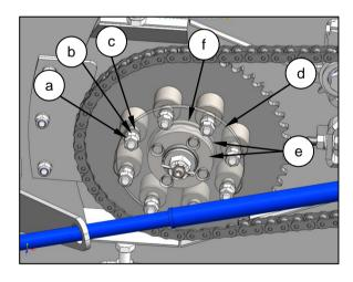
Loosen and remove the outer locknut (a) then loosen and remove the inner nut (b) and washer (c). The drive disc (d) can now be removed exposing the two clutch plates (e).
