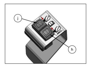
The position of the crop deflector is shown by the color coded indicator rod.
