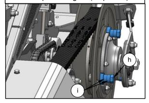
**11.** Re-fit the ram to the gearbox bracket using bolt (g)
