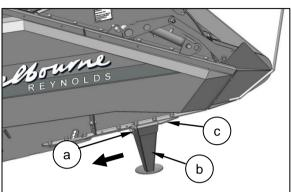
The header stands can then be stored on a bracket on the rear (right hand side) of the header. Slide each stand (b) onto the bracket (d) and secure in place with the linchpin (a).
