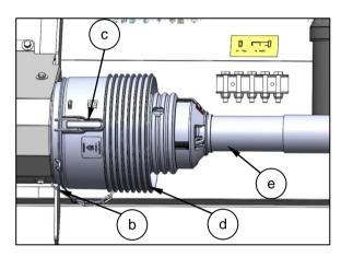
Remove any remnants of the broken shearbolt, align the two halves of the PTO shear bolt clutch (f) and fit a new shearbolt (a), fully tighten the locking nut.
