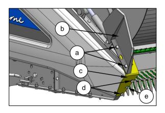
There is no need to remove the right hand guard fastener (e).
