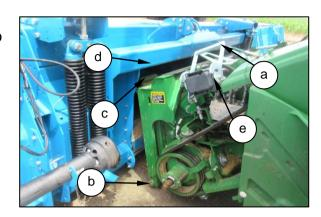
Raise the feeder house to lift the header, ensuring that the feeder saddle is properly engaged in the adaptor plate, then fully raise the header.
