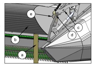
Remove support (a) and disengage the crop deflector safety stop (d), then fully lower the crop deflector by operating the combine's reel lower or reel fore/aft function.
