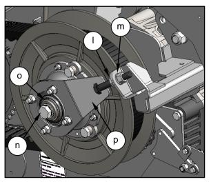
9. Remove the spacer (q) and slide the rear gearbox pulley assembly off the gearbox shaft and carefully lower it to the ground. At this stage the belt will remain inside the pulley sheaves.
