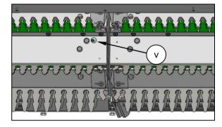
Refit the grease hole plug.
