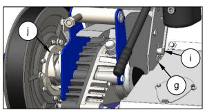
Both cams (h & j) are free to rotate to check for smooth rotation and wear in the bearings.
