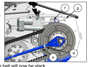
**9.** Ensure that the wooden block is wedged securely between the rotor pulley sheaves and remove the belt, first from the rotor pulley, then from the gearbox pulley.
