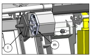
Connect the PTO shaft and monitor electrical connectors, then remove the header stands, as described in Section 5.1.10.
