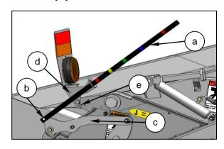
Remove the bolt (b) securing the indicator rod to the link arm (c). Thread the end of the indicator rod through the light mounting bracket (d). Bolt the indicator rod back onto the link arm.
