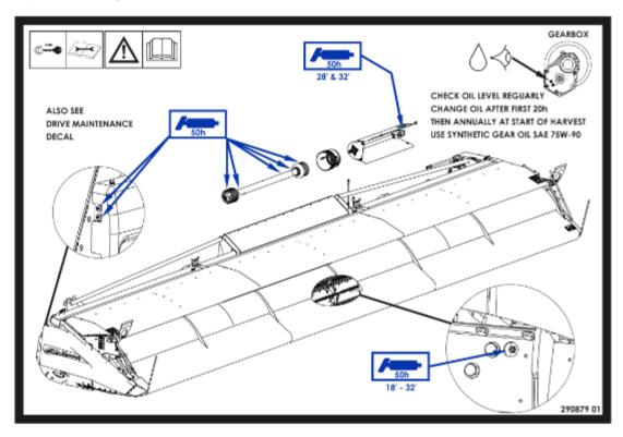
A second decal is fitted under the left hand drive guard and indicates the grease points on the variable speed drive pulleys (CVS & RVS only) and the left hand rotor and auger bearings.
