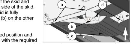
Lower the skid to the desired position and then refit bolt (b) aligning it with the required
