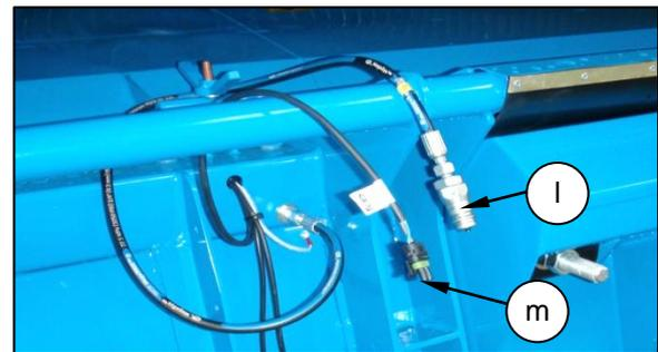
Remove the header crop deflector hose (l) from the combine reel lift connector (k) and refit the plug.
