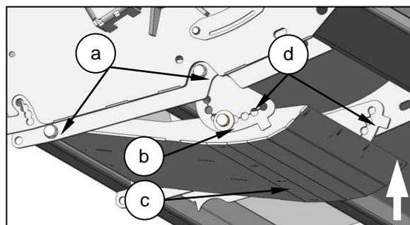
Lower the skid to the desired position and then refit bolt (b) aligning it with the required hole in the skid adjuster plate (d) and the skid. Repeat the process on the other side of the skid, ensuring that the same hole is used in both skid adjuster plates. Fully tighten all bolts (a & b) on both sides of the skid.
