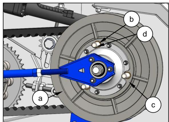
To replace bushes and pins the gearbox pulley will need to be removed and stripped, contact your Shelburne dealer.
