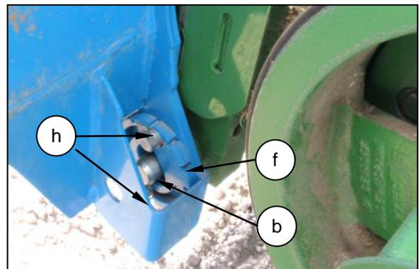
Re-tighten the bolts. Adjust this to ensure the locking pins (b) do not have too much movement in the adjuster plate (f).
