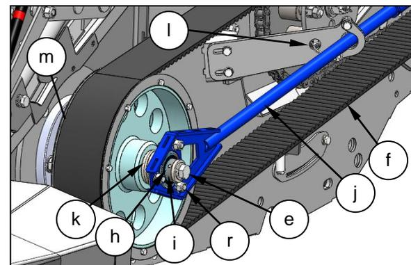
7. Remove the required pulley securing bolts (e) and associated washers, then remove the tie rod bearing (i) and tie rod (j) from either, or both of the shafts.
