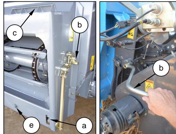
Raise the feeder house to lift the header, ensuring that the feeder house hooks (c) are properly engaged in the adaptor plate thus allowing the lower pins (e) to penetrate the sockets (f), then fully raise the header.
