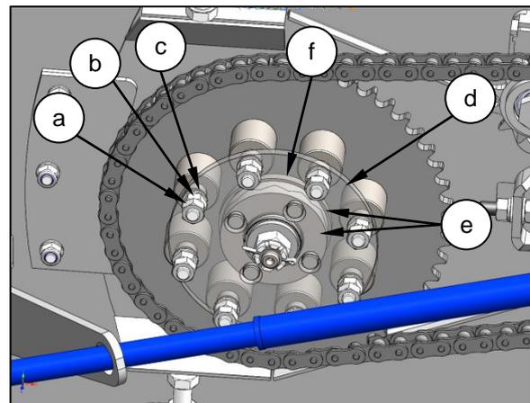
Loosen and remove the outer locknut (a) then loosen and remove the inner nut (b) and washer (c). The drive disc (d) can now be removed exposing the two clutch plates (e).
