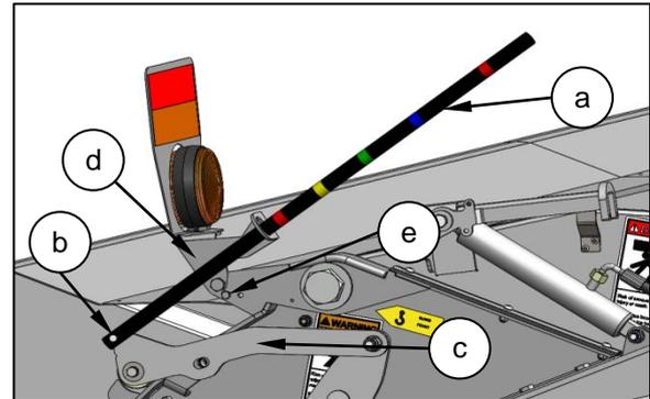
Remove the bolt (b) securing the indicator rod to the link arm (c). Thread the end of the indicator rod through the light mounting bracket (d). Bolt the indicator rod back onto the link arm.
