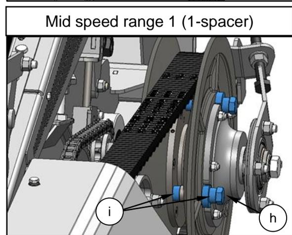
10. Tighten the three nuts & bolts (h)
