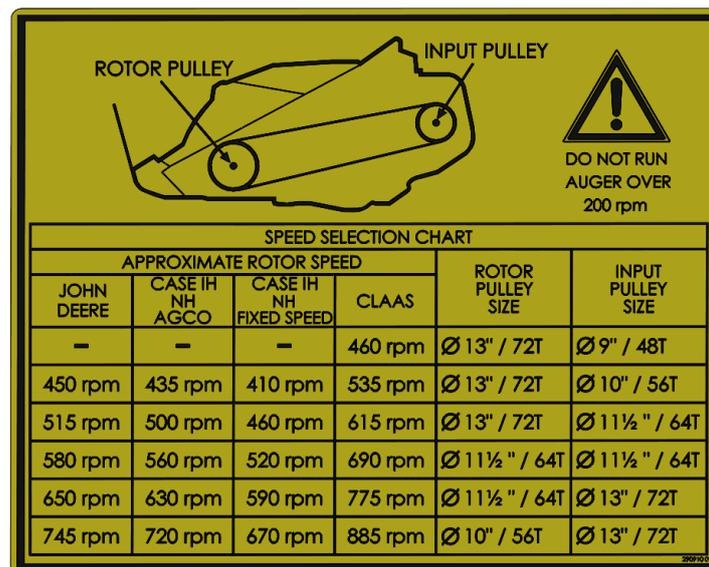
The rotor speeds are approximate and are dependent on the combine feeder house output shaft speed and the correct gear combinations being fitted inside the gearbox. These are shown in the table below for RSD Stripper Headers
