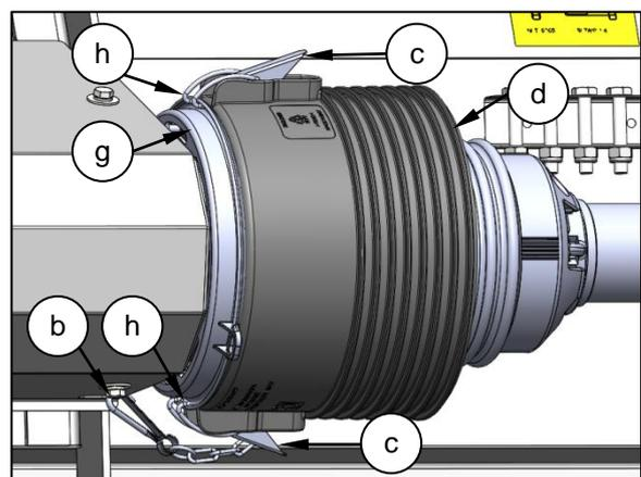
Reconnect the left hand end PTO guard retaining chain (b) to the header
