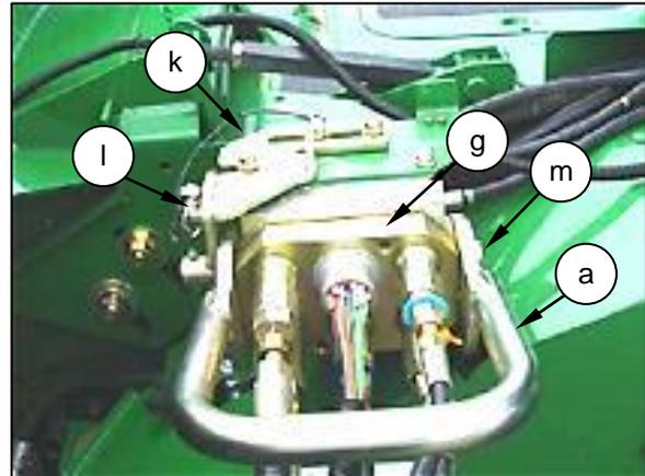
Ensure the button (m) engages to lock the handle (a) or slide latch (k) across and secure with the linchpin (l).
