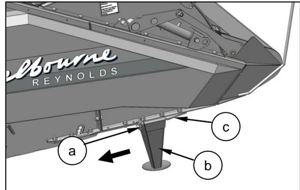
The header stands can then be stored on a bracket on the rear (right hand side) of the header. Slide each stand (b) onto the bracket (d) and secure in place with the linchpin (a).
