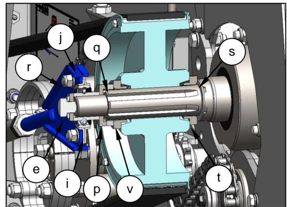
9. Remove the required pulley. Ensure that the inner tapered collar (m), stepped washer (t) or flat washer (u) and any shims (s) are left on the shaft and not removed with the pulley.
