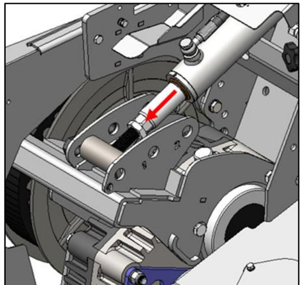
12. Remove the wooden block from the front pulley.
