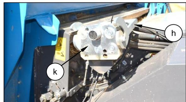
Remove the coupler (g) from its storage bracket (j) on the header and clean both multicoupler faces.
