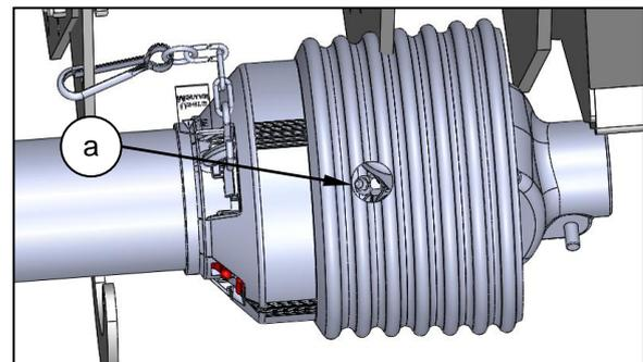
Machines over 7.2m (24') have an additional grease point. Turn the fastener (g) and open the rear guard inspection cover (h). Rotate the driveline with a wrench on the central bolt of the pulley until the grease (i) point is accessible through the inspection hole. Once this has been greased close the inspection cover (h) and secure with fastener (g).
