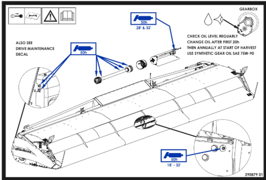
A second decal is fitted under the left hand drive guard and indicates the grease points on the variable speed drive pulleys (CVS & RVS only) and the left hand rotor and auger bearings.
