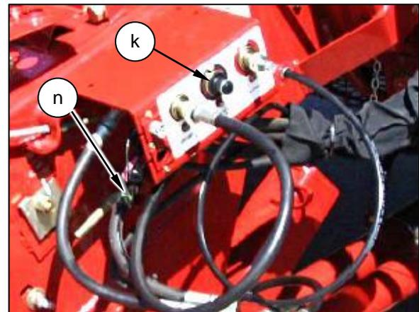
Connect the header 3 pin electrical cable connector (m) to the combine electrical connector (n).
