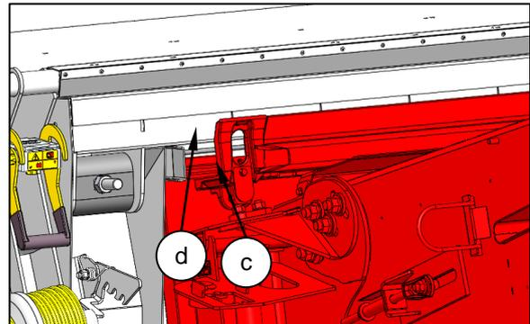
Raise the feeder house to lift the header, ensuring that the feeder saddle is properly engaged in the adaptor plate, then fully raise the header.
