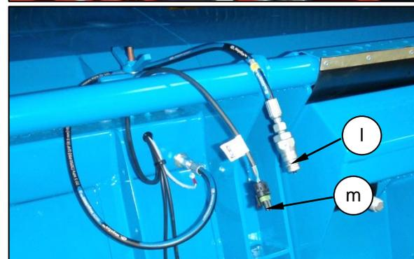
Connect the PTO shaft and monitor electrical connectors, then remove the header stands, as described in Section 5.1.10.
