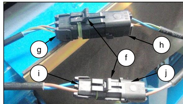
Secure the disconnected cables to prevent damage occurring.
