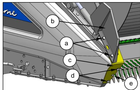
There is no need to remove the right hand guard fastener (e).
