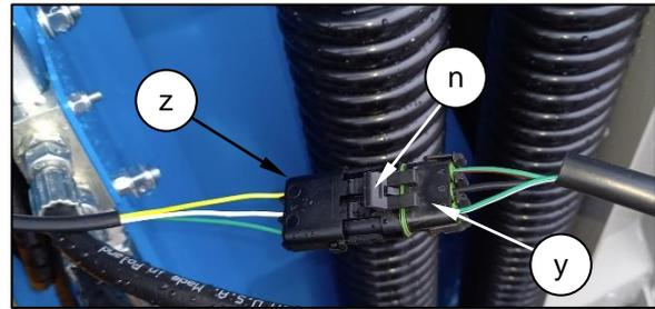
Ensure that the tab (n) is engaged to prevent the connectors from coming apart
