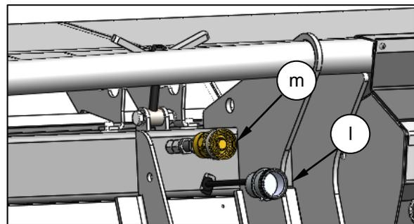
Connect the PTO shaft and monitor electrical connectors. Then remove the header stands, as described in Section 5.1.10.
