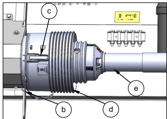
Remove any remnants of the broken shearbolt, align the two halves of the PTO shear bolt clutch (f) and fit a new shearbolt (a), fully tighten the locking nut.
