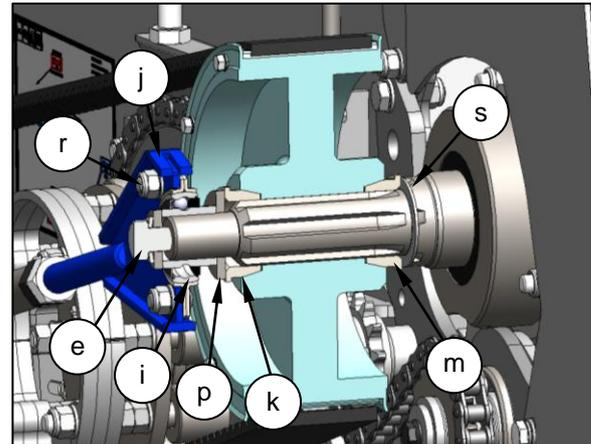
8. Remove the washer (p), outer shim (q), if fitted and tapered collar (k), this may require a light tap with a hammer. On later Stripper Headers the tapered collars (k & m) have been replaced by either stepped washers (t & v) or flat washers (u & w) and can have shims (q & s) on both side of the gearbox pulley. Later Stripper Headers with hexagonal tie rod bearing do not have washer (p) fitted
