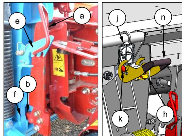
Close the cover (j) on the header multicoupler and lower the handle (n) to the "closed position".
