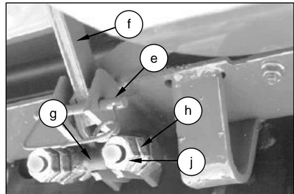
Lift the handles (f) to the "over centre position" to lock. The force required to over centre the handle should be 180-220 Nm (40-50 lbf). Adjust the nuts (h) on the fixing bar to vary force required on handle.
