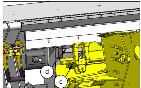
Raise the feeder house to lift the header, ensuring that the feeder saddle is properly engaged in the adaptor plate, then fully raise the header.
