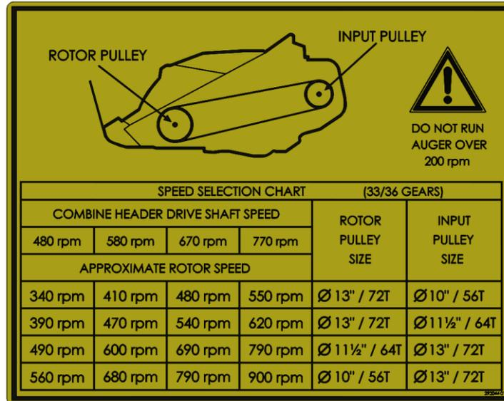
The gearbox on CSD Stripper Headers is fitted with a 33 tooth input gear and a 36 tooth output pinion gear.
