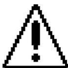
This safety alert symbol indicates an important safety message in this manual and on safety signs on the machine.
