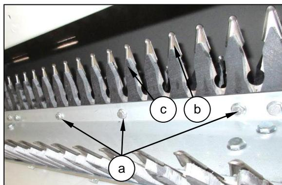
Place the new section in position, ensuring formed cups are pointing in the correct direction. If it is difficult to push into the rotor, it may be tapped into place with a small bar in the bottom of the keyhole.
