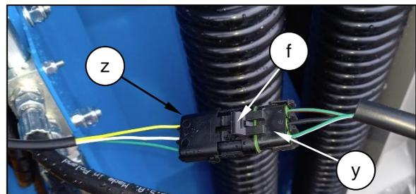
On John Deere X9, S7 and T5/6 combines fitted with Shelbourne light loom kit raise the tab (f) and pull the plug (y) and socket (z) apart.
