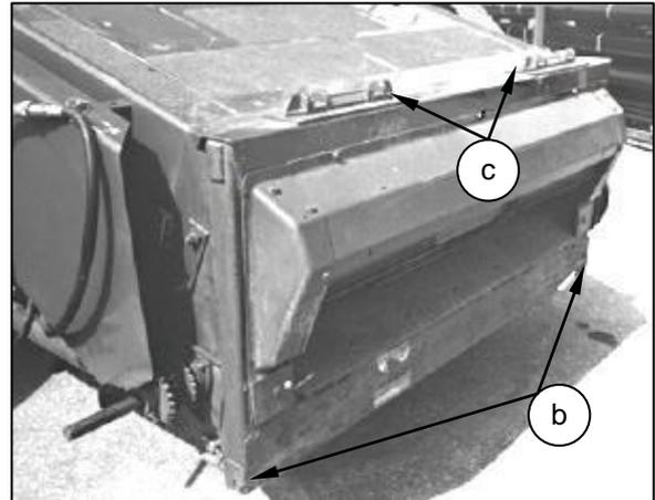
Raise the feeder house to lift the header, ensuring that the pivot blocks (c) are properly seated in the pockets (e) in the adaptor plate top beam, then fully raise the header.
