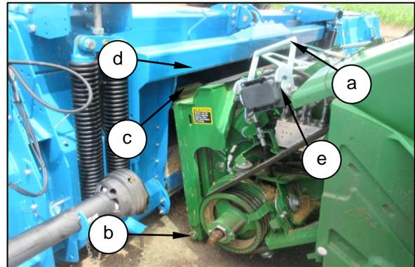
Drive the combine slowly forward, ensuring the feeder house is centred and parallel with the adaptor plate opening, until the feeder house saddle (c) is directly under the adaptor plate top beam (d).
