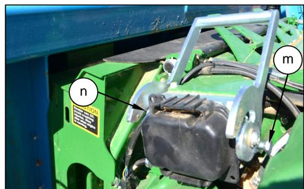
Push up the multicoupler handle (a) to the "nearly up position", remove the plastic cover (n) from combine multicoupler (e) and clean the multicoupler face.
