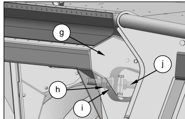
Once the required pitch has been achieved adjust inner nuts (j) to the adaptor plate and tighten outer nuts (i) fully. Tighten lock nuts (h). Ensure that the adjustment is the same either side of the adaptor plate. If the Stripper Header needs to be pitched down follow the same procedure, except wind nuts (h, i & j) towards the combine. Do not unthread the nuts off of the bolt as this will cause the Stripper Header to fall.
