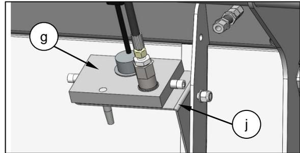
Locate the coupler (g) onto the receptacle multicoupler (k) on the feeder house. Pull the handle (h) down to fully engage the coupler (g).
