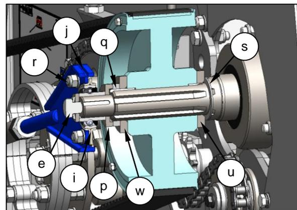
11. Refit the tapered collar (k), stepped washer (v) or flat washer (w), shim (q) and washer (p). On later Stripper Headers the gearbox pulley washer (p) has a counterbore, so ensure it is fitted the correct way around.
