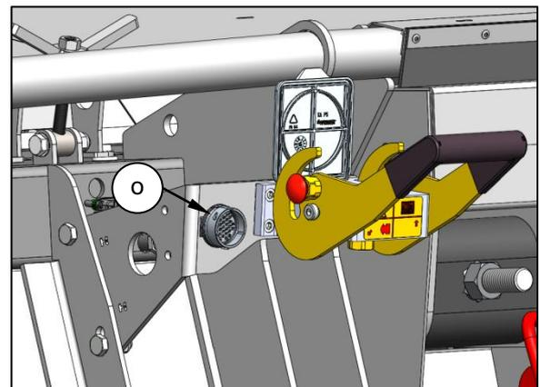
Connect the PTO shaft and monitor electrical connectors, then remove the header stands, as described in Section 5.1.10.
