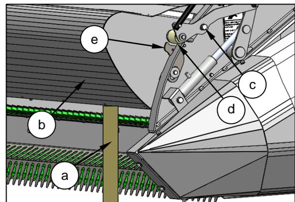
Remove the shipping bolt (c) and its spacers and washers. The nut for this is fixed.
