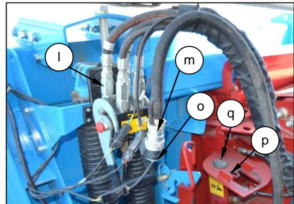
Depress the red button (k) on the header multicoupler (h) and raise the handle (n) to release the combine quick coupler (l).
