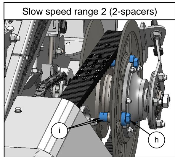
9. Re-fit the bolts (h) with the required number of spacers (i) between the pulley sheaves.
