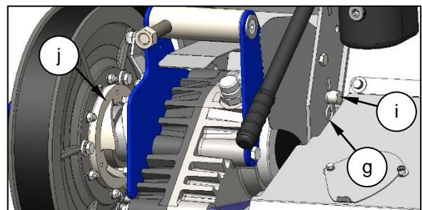
Both cams (h & j) are free to rotate to check for smooth rotation and wear in the bearings.
