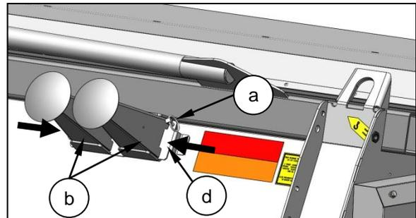
Remove the feeder house cylinder lock.
