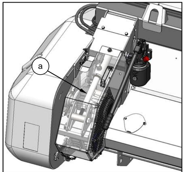
4. Open and remove the LH drive guard (see section 6.10.1), and then open the gearbox guard.
