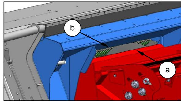
Raise the feeder house to lift header, ensuring that the feeder saddle is properly engaged in the adaptor plate, then fully raise the header.
