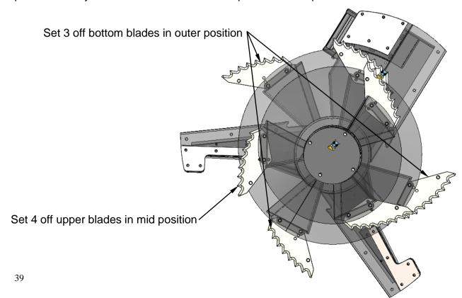
Follow the below procedure when changing the angle of the auger blades:
