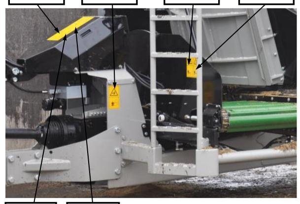
193391 01 Ensure PTO shaft guards are fitted and safety chains are attached.
