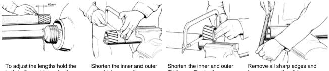
half shafts next to each other in the shortest working position and mark them 40mm as shown. guard tubes equally.
