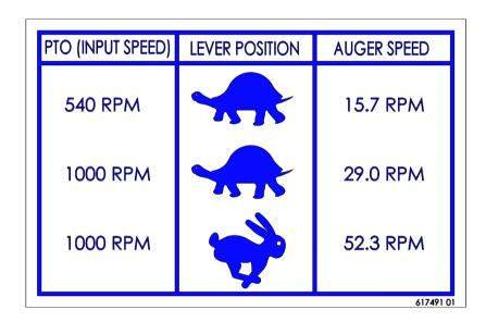
The 29 rpm auger speed is suitable for the majority of mixing and chopping situations. If the mix is being over processed the engine revs / PTO rpm of the tractor can be reduced to achieve a slower auger speed.
