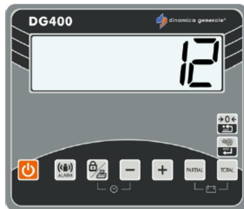
5. The word CALIB will appear on the display. Press the MINUS and PLUS keys to change the value of this parameter to 5005.
