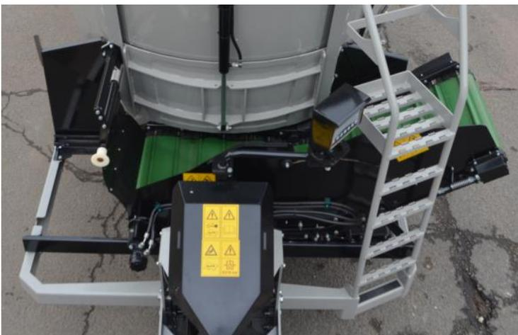
The movement of the conveyor belt is generated by operating two linked hydraulic cylinders (a) which are situated underneath the conveyor belt. To move and elevate the conveyor to the right the hydraulic cylinders are extended, and to move and elevate the conveyor to the left the hydraulic cylinders are retracted. The conveyor system starts to elevate when the jacking arms (b) reach a stop which allows one half of the conveyor frame to pivot which in turn starts the lifting motion.
