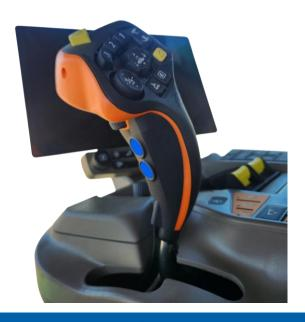
A combine multi-function lever mounted switch will be available (June 2025) as an alternative to the console bracket-mounted rocker switch. This molded switch assembly fixes to the John Deere multi-function lever.
