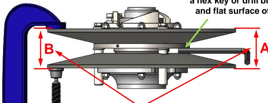
Measure width on outside of pulley sheaves
