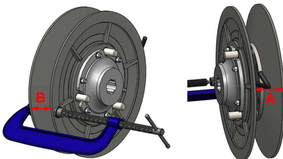
Use a reliably sized shim such as a hex key or drill bit between hub and flat surface of inner pulley
