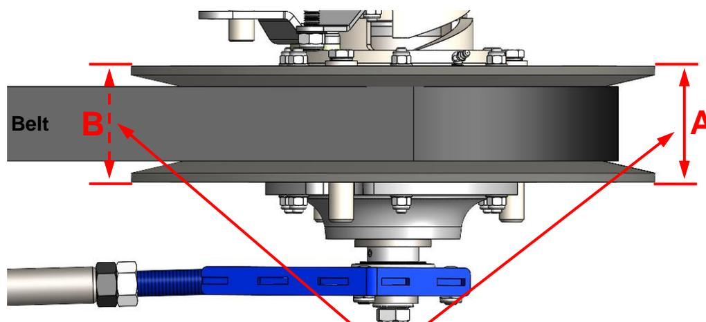
**Measure width on outside of pulley sheaves**
